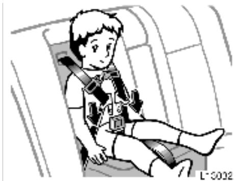
7. Sit the child on the child seat. Place a shoulder belt over each shoulder. Insert the tabs into the buckle.
