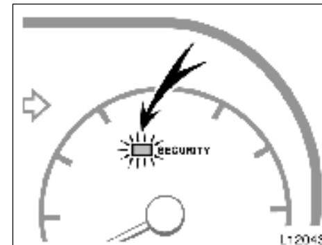
The system is automatically set when the key is removed from the ignition switch. The indicator light will start flashing every 1 second to show the system is set.
