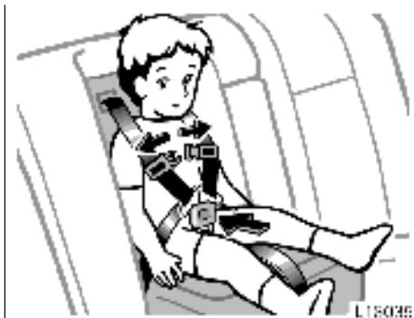
10. To release the child from the seat belts, separate the shoulder belts then press the buckle release button.
