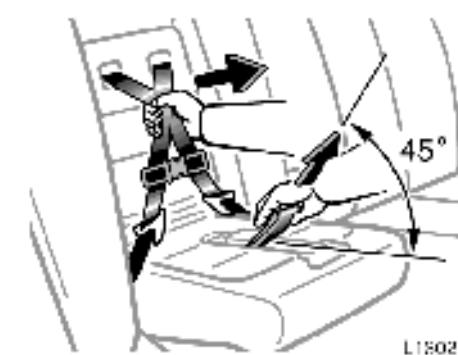
1. Remove the head restraint and upper pad by pressing the head restraint lock release button and pulling up the head restraint and upper pad. Lower the child seat cushion.
