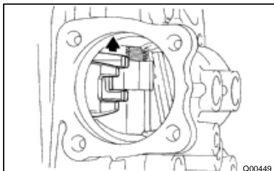
9. REMOVE OUTPUT SHAFT LOCK NUT
