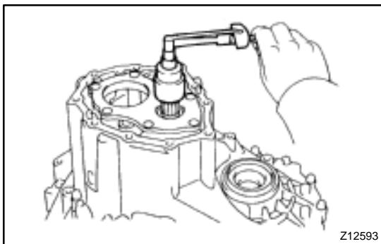
(j) Using a torque wrench, measure the preload.
