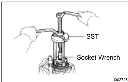
(b) Using SST and a socket wrench, remove the No.3 clutch hub with the synchronizer ring.
