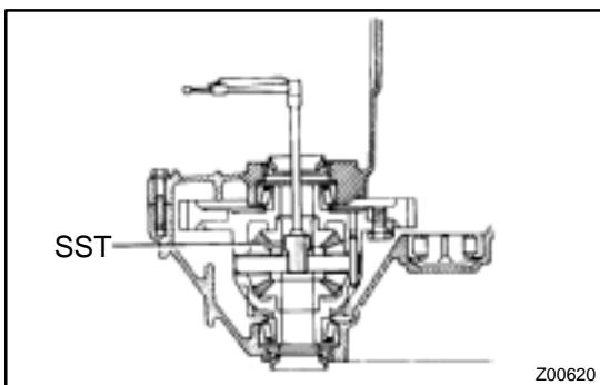
(g) Using SST and a torque wrench, measure the preload.
