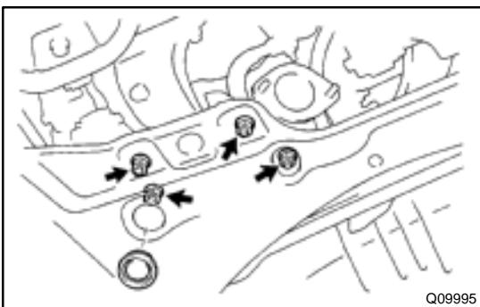
**22. REMOVE HOLE PLUG AND 4 ENGINE REAR SIDE MOUNTING NUTS**
