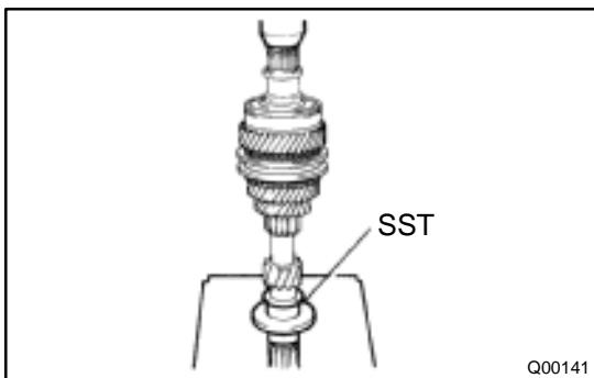
(j) Using SST and a press, install a new input shaft front bearing inner race.
