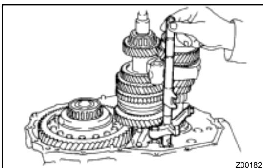
**30. REMOVE NO.3 SHIFT FORK SHAFT WITH REVERSE SHIFT FORK AND NO.2 SHIFT FORK**
