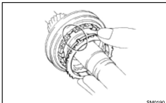
(c) Place the synchronizer ring on the gear.
