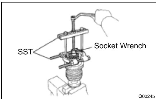
(e) Using SST and a socket wrench, remove the output shaft front bearing.
