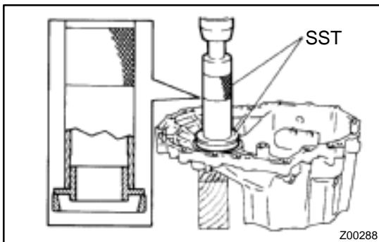
(f) Using SST and a press, install a new tapered roller bearing outer race.
