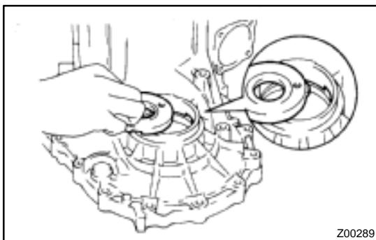
(g) Install the oil baffle.
