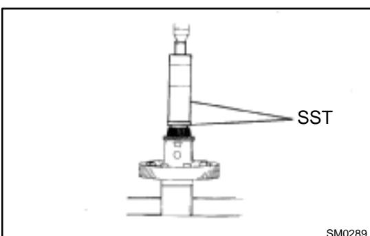
(c) Using SST and a press, install a new side bearing to the transaxle case side.
