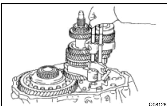
**29. REMOVE NO.2 SHIFT FORK SHAFT, SHIFT HEAD AND NO.1 SHIFT FORK**
