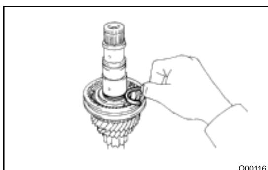
**4. MEASURE 3RD GEAR THRUST CLEARANCE
