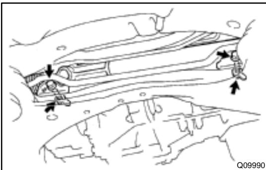
(d) Tie the PS gear assembly to the proper position with a code or an equivalent to suspend the assembly securely.
