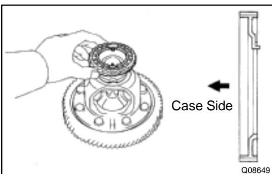
(b) Install the vehicle speed sensor drive gear to the trans-
