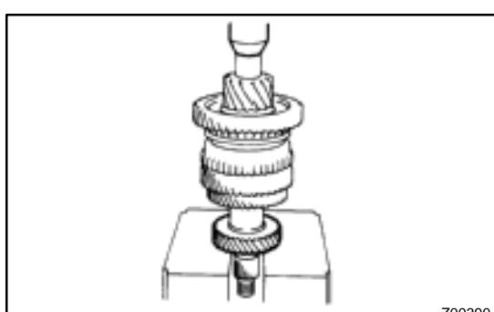
**8. INSTALL OUTPUT SHAFT REAR BEARING**
