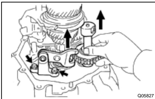
21. **REMOVE REVERSE IDLER GEAR AND SHAFT**
