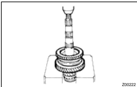
**7. REMOVE NO.1 HUB SLEEVE ASSEMBLY AND 1ST GEAR**
