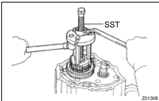
(b) Using SST, remove the No.3 clutch hub with the synchronizer ring and 5th gear.
