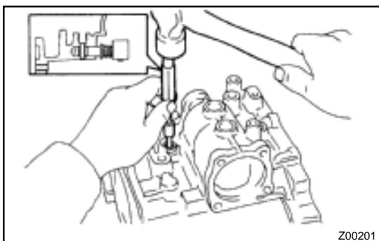
(d) Using a pin punch and hammer, drive in the slotted spring pin.
