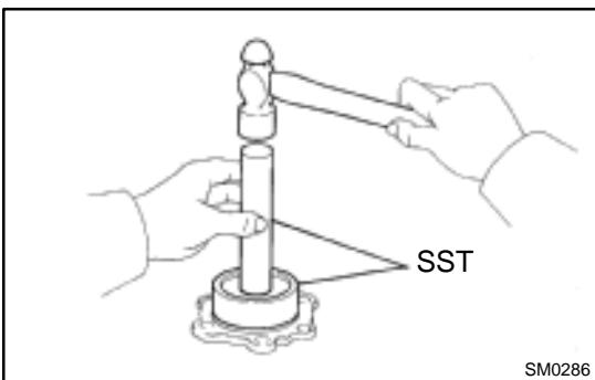
(b) Using SST and a hammer, drive in a new oil seal until its surface is flush with the case surface.
