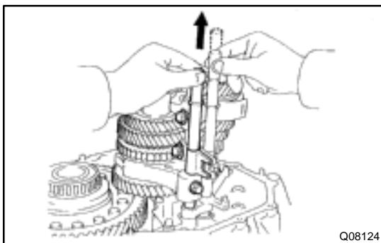
**26. REMOVE NO.1, NO.2 SHIFT FORKS AND SHIFT HEAD SET BOLT**
