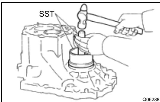
(h) Using SST and a hammer, drive in a new oil seal.
