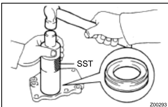
(f) Using SST and a hammer, drive in a new oil seal.
