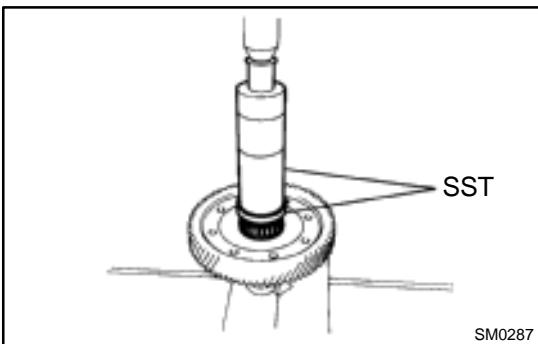
**3. INSTALL SIDE BEARING TO DIFFERENTIAL CASE**
