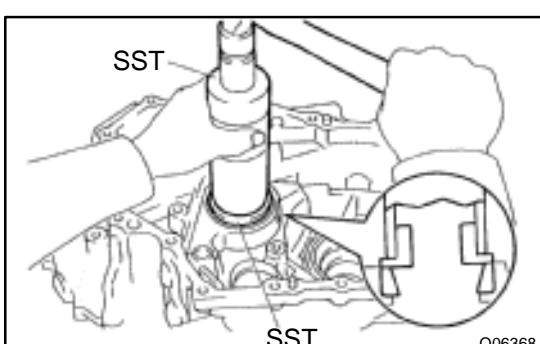
(d) Using SST and a hammer, drive in a new output shaft front bearing outer race.
