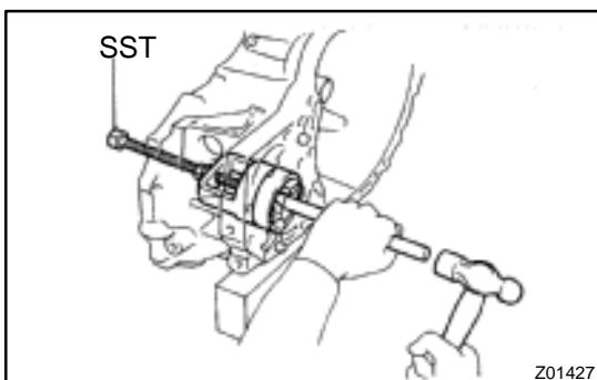
(d) Using SST, a brass bar and hammer, remove the tapered roller bearing outer race.
