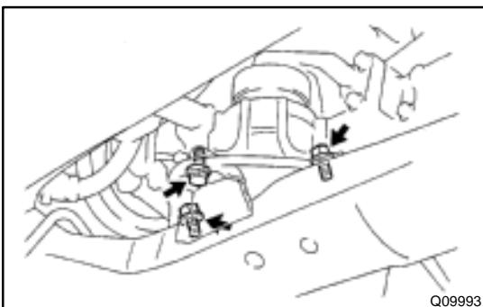
**20. REMOVE 3 ENGINE FRONT SIDE MOUNTING BOLTS**
