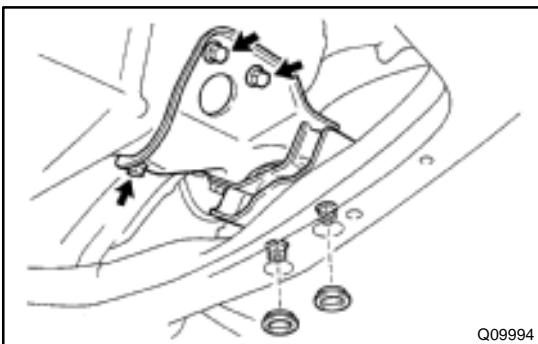
**21. REMOVE LH ENGINE MOUNTING INSULATOR WITH BRACKET**
