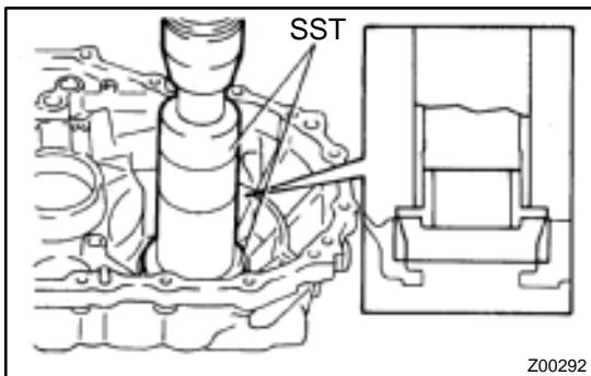
(e) Using SST and a press, install a new tapered roller bearing outer race.
