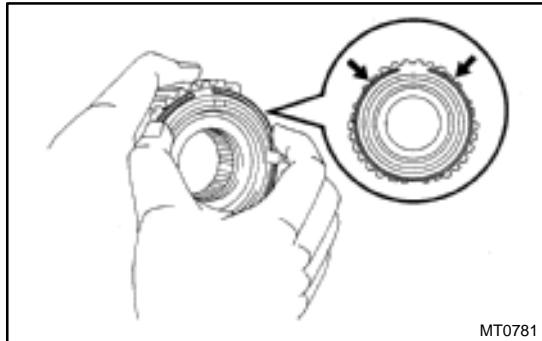
36. **REMOVE NO.5 SYNCHRONIZER RING WITH KEY SPRING FROM NO.3 CLUTCH HUB**
