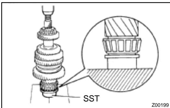
(f) Using SST and a press, install a new output shaft front bearing.
