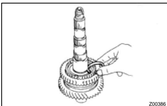
**4. MEASURE 1ST GEAR THRUST CLEARANCE
