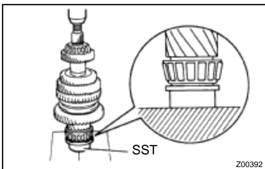
**9. INSTALL OUTPUT SHAFT FRONT BEARING**
