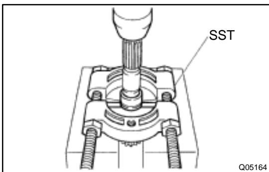
(i) Using SST and a press, remove the inner race.
