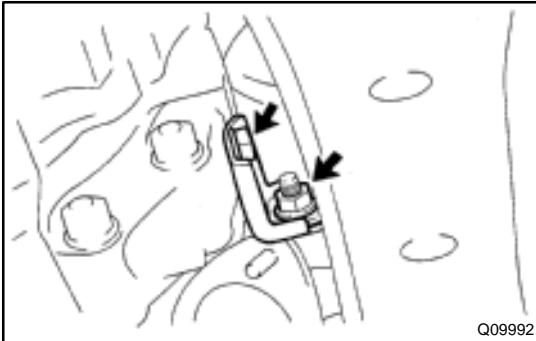
**19. REMOVE RH EXHAUST MANIFOLD STAY**
