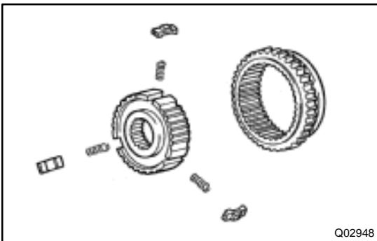
**6. REMOVE NO.1 HUB SLEEVE, 3 SHIFTING KEYS AND SPRINGS FROM NO.1 CLUTCH HUB**
