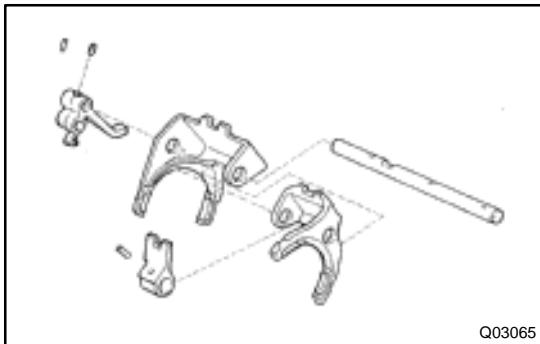
27. **SEPARATE NO.1 SHIFT FORK SHAFT, NO.1 SHIFT HEAD, NO.1, NO.2 SHIFT FORKS AND REVERSE SHIFT FORK**
