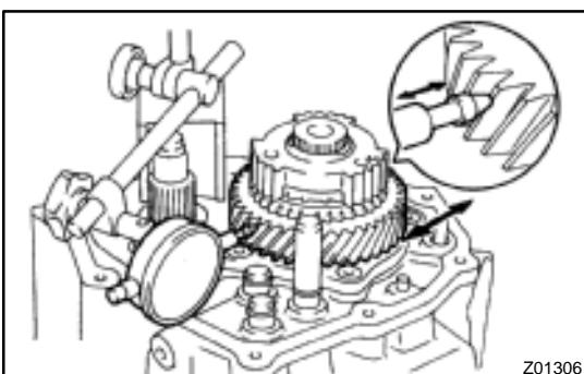
(b) Using a dial indicator, measure the radial clearance.
