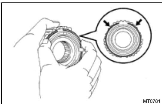
**28. REMOVE NO.5 SYNCHRONIZER RING WITH KEY SPRING FROM NO.3 CLUTCH HUB**
