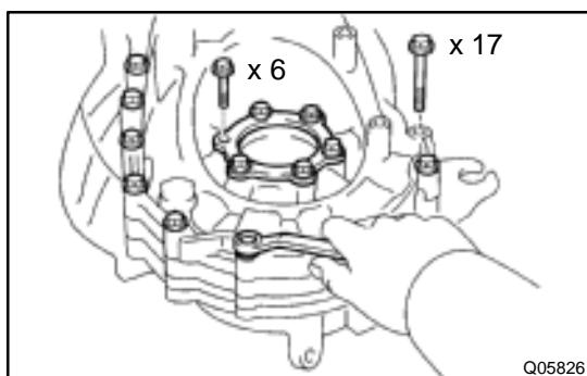
**18. REMOVE REVERSE IDLER GEAR SHAFT LOCK BOLT AND GASKET**
