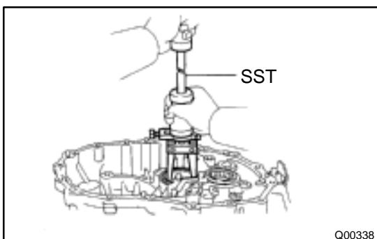
**4. IF NECESSARY, REPLACE OUTPUT SHAFT FRONT BEARING OUTER RACE AND OUTPUT SHAFT FRONT COVER**
