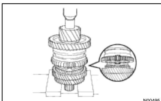
**7. INSTALL SPACER AND 4TH DRIVEN GEAR**
