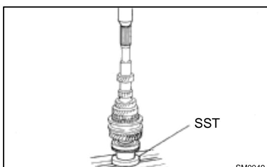
(d) Using SST and a press, install the rear ball bearing.
