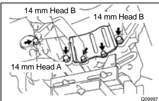
**27. REMOVE FLYWHEEL HOUSING UNDER COVER AND TRANSAXLE LOWER SIDE MOUNTING BOLT**
