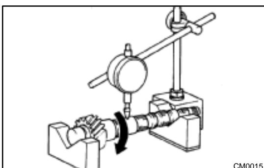
(b) Using a dial indicator, check the shaft runout.
