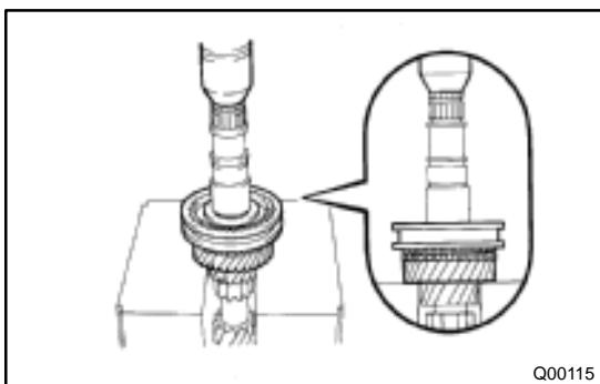
**7. REMOVE NO.2 CLUTCH HUB ASSEMBLY, SYNCHRONIZER RING AND 3RD GEAR**
