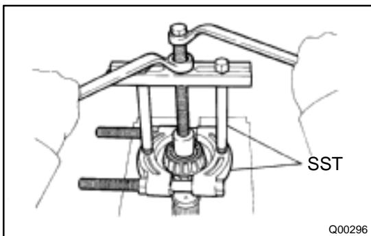
**9. REMOVE OUTPUT SHAFT FRONT BEARING**
