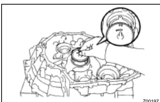
(c) Install a new output shaft cover.
