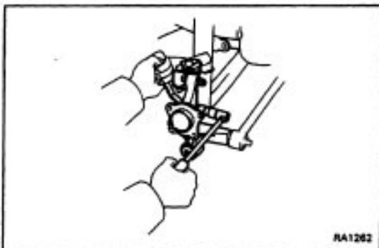
(e) Remove the axle carrier from the rear shock absorber.
