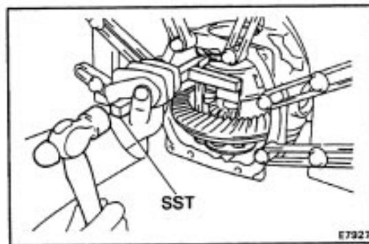
(b) Install a new plate washer of 0.06 – 0.09 mm (0.0024 – 0.0035 in.) thicker than the removed washer.
