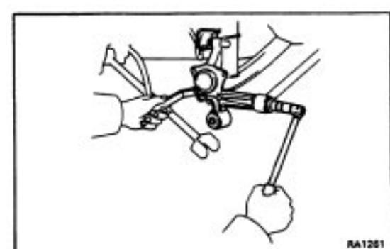
(b) Disconnect the No. 1 and No.2 suspension arm from the axle carrier.
