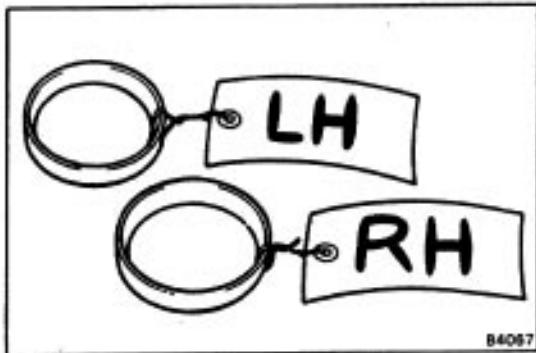
HINT: Tag the bearing outer races to show the location for reassembly.
