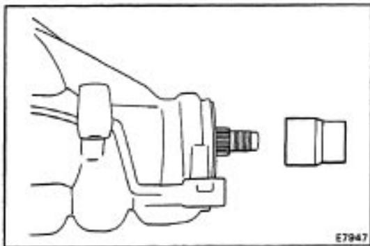
(b) Remove the bearing spacer.
