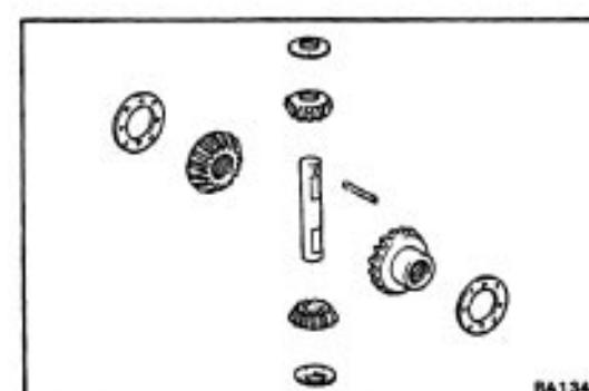
(b) Remove the following parts from differential case:
