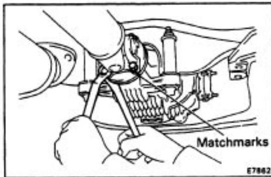
**11. CONNECT PROPELLER SHAFT**
