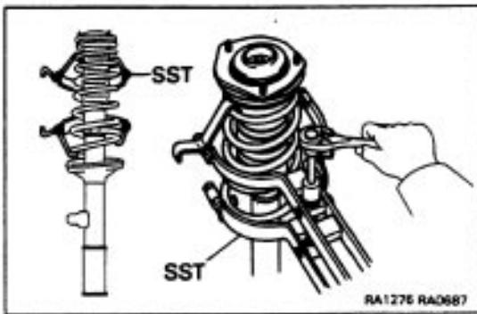
(b) Using SST, compress the coil spring.
