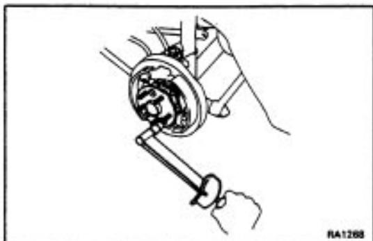
(c) Install the axle hub and torque the four bolts.
