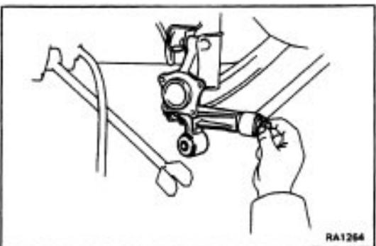
(c) Connect the No. 1 and No.2 suspension arm to the axle carrier with the bolt, and temporarily install the retainer and nut.
