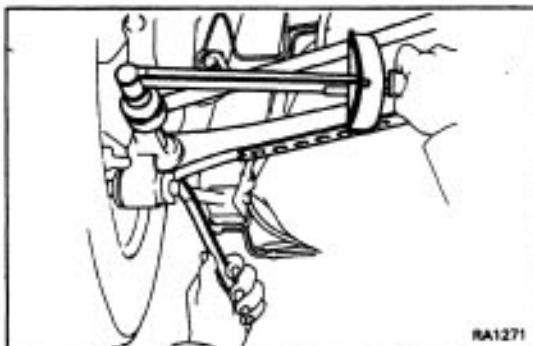
(b) Torque the suspension arm installation bolt to the axle carrier with the vehicle weight on the suspension.
