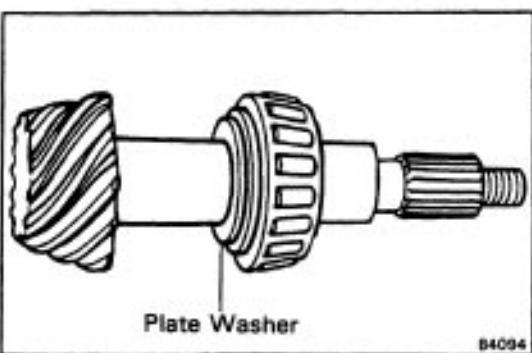
If the teeth are not contacting properly, use the following chart to select a proper washer for correction.
