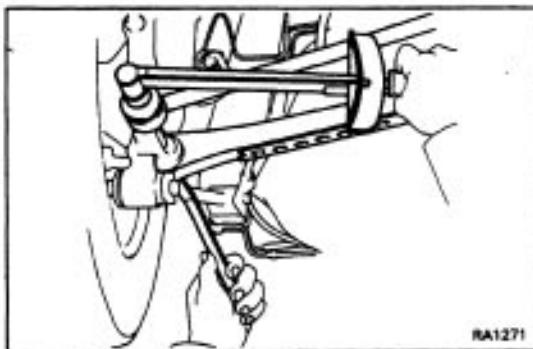
(b) Torque the suspension arm installation bolt to the axle carrier with the vehicle weight on the suspension.
