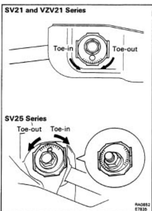
If the left-right error is within specifications but the overall toe-in is not, lengthen or shorten both arms an equal amount by turning the two cams in the opposite direction, until the adjustment standard is obtained.
