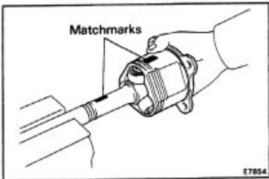
(b) Align the matchmarks placed before remove, and install the inboard joint tulip to the drive shaft.
