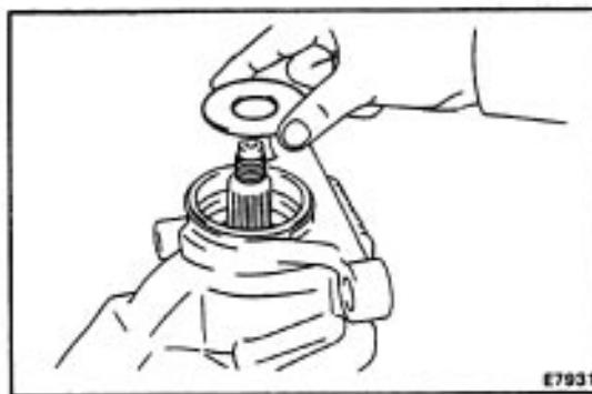
**16. INSTALL OIL SLINGER**
