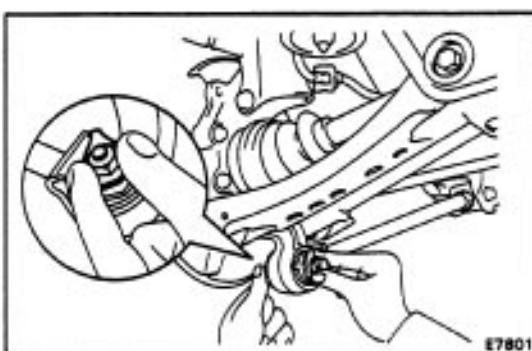
(e) Temporarily connect the strut rod to the axle carrier.
