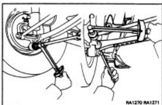
**REPLACEMENT OF REAR AXLE HUB BOLT**
