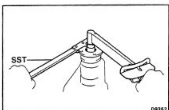
(c) Adjusting the drive pinion preload by tightening the companion flange nut.
