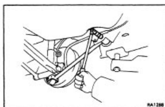
(b) Remove the strut rod installation bolt and nut from the body.
