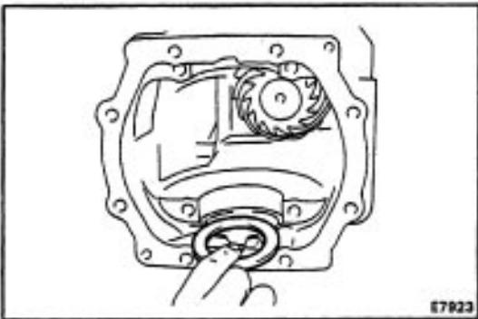
(f) Remove the plate washer and differential case. Install the plate washer into the ring gear back side.
