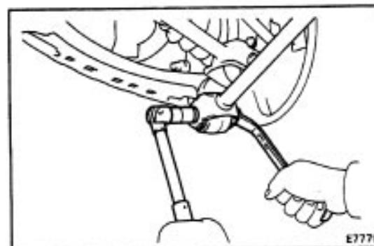
(b) Disconnect the strut rod from the axle carrier.
