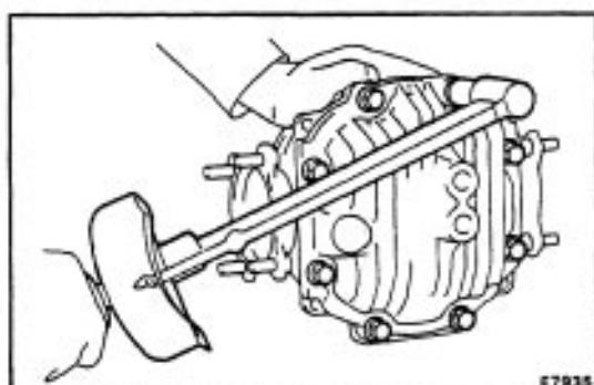
(c) Install and tighten the eight set bolts.
