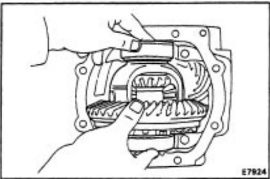
(g) Place the other plate washer onto the differential case together with the outer race, and install the differential case with the outer race into the carrier.
