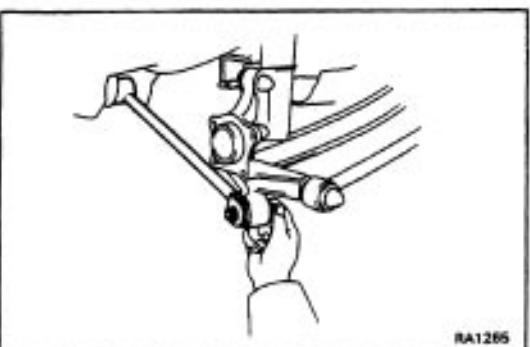
(d) Temporarily connect the strut rod to the axle carrier with the bolt and the nut as shown in the figure.
