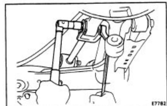
(c) Disconnect the No. 1 suspension arm from the axle carrier.
