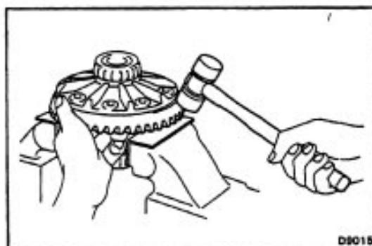
(d) Using a plastic hammer, tap on the ring gear to separate it from differential case.
