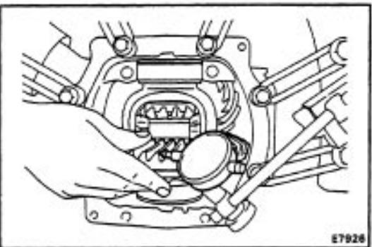
(j) Using a dial indicator, measure the ring gear backlash.
