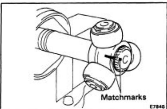
(b) Place matchmarks on the shaft and the tripod.
