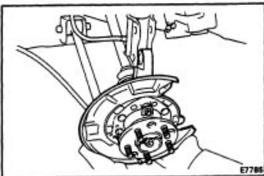
(e) Remove the axle carrier with axle hub.
