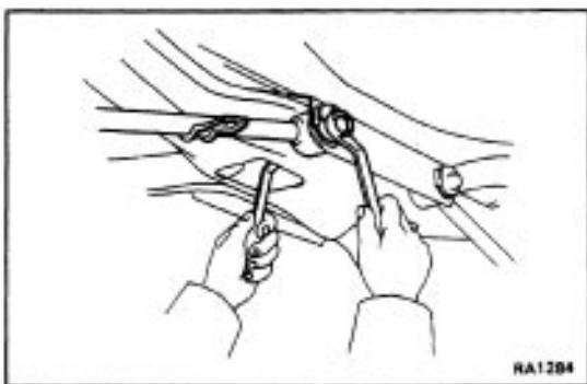
(b) Remove the cam and the cam bolt from the body and remove the No.2 suspension arm.
