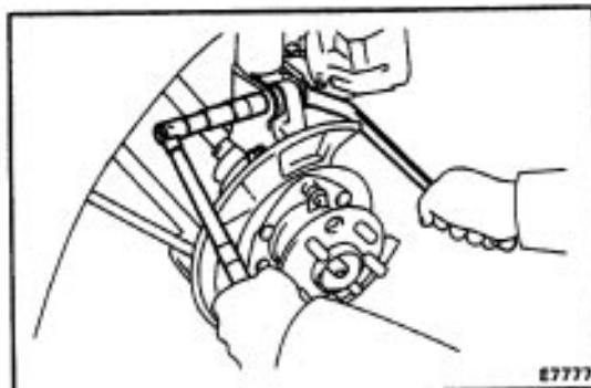
**9. REMOVE AXLE CARRIER WITH AXLE HUB**
