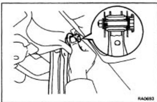
Temporarily install the No. 1 suspension arm to the body with the bolt, plate and nut.
