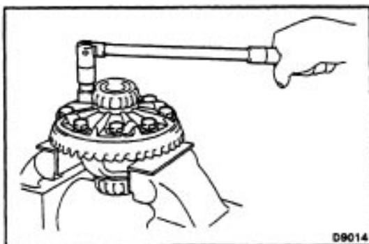
(c) Remove the eight bolts and lock plates.
