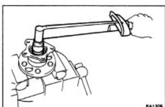
(c) Install and torque a new lock nut.
