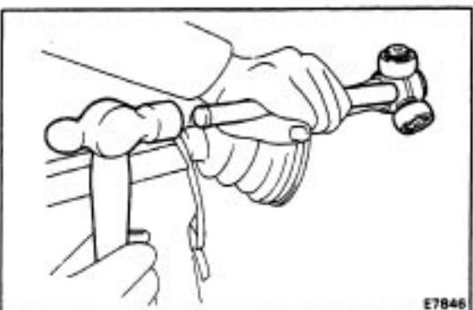
(c) Using a hammer and brass bar, drive out the tripod joint from the drive shaft.
