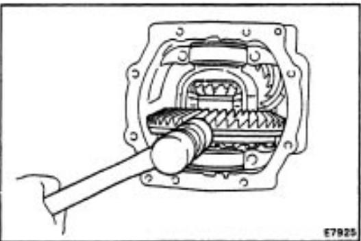
(h) Using a plastic hammer, snug down the washer and bearing by tapping the ring gear.
