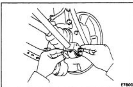
(d) Temporarily connect the No. 1 suspension arm to the axle carrier.
