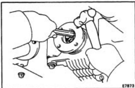
**10. STAKE DRIVE PINION NUT**
