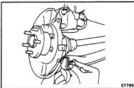
(c) Temporarily connect the No. 2 suspension arm to the axle carrier.
