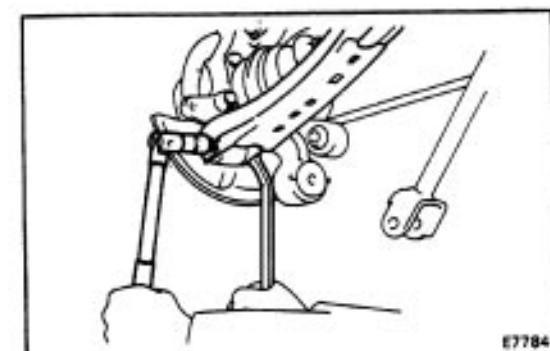
(d) Disconnect the No. 2 suspension arm from the axle carrier.
