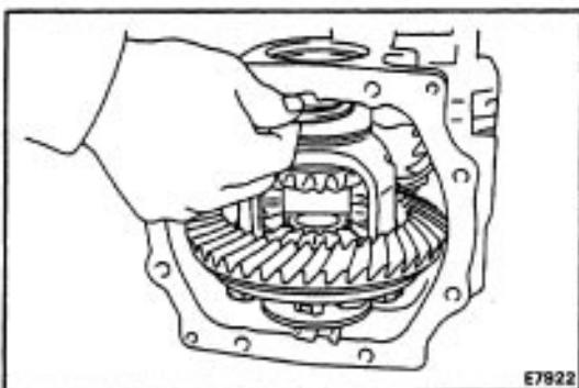
(e) Select a ring gear teeth side washer with a thickness which eliminates any clearance between the outer race and case.
