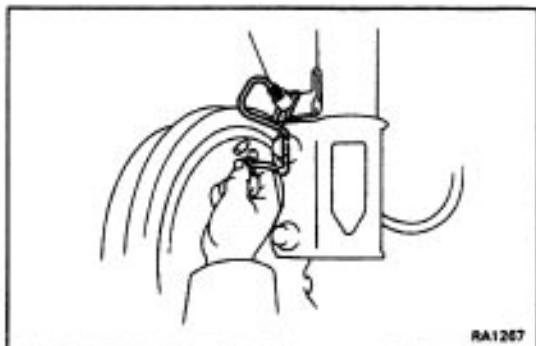
(b) Temporarily connect the brake tube to the backing plate.
