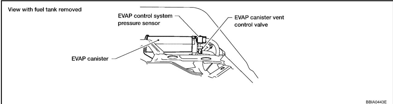
3. Pressurize the EVAP line using pressure pump with 1.3 to 2.7 kPa (10 to 20 mmHg, 0.39 to 0.79 inHg), then remove pump and EVAP service port adapter.
