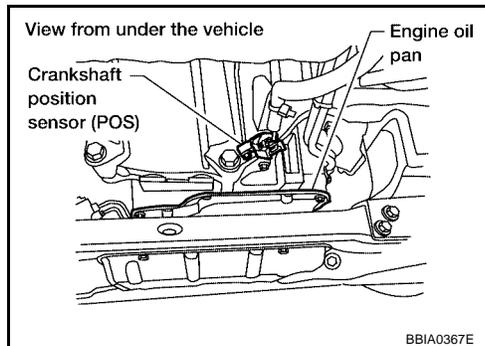
3. Check voltage between CKP sensor (POS) terminal 3 and ground with CONSULT-II or tester.
