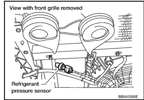
3. Check voltage between refrigerant pressure sensor terminal 1 and ground with CONSULT-II or tester.
