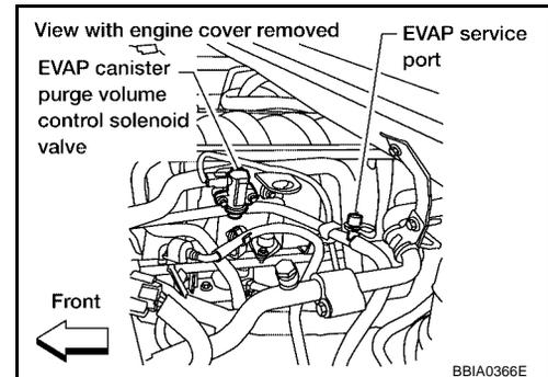
4. Check voltage between EVAP canister purge volume control solenoid valve terminal 1 and ground with CONSULT-II or tester.
