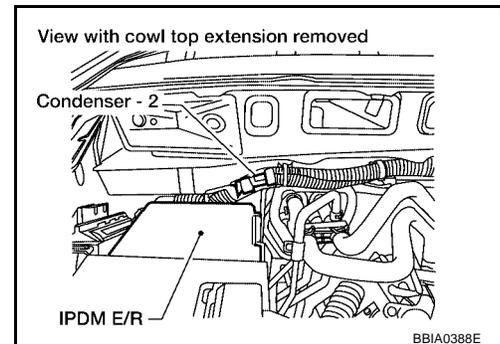
5. Check voltage between condenser terminal 1 and ground with CONSULT-II or tester.
