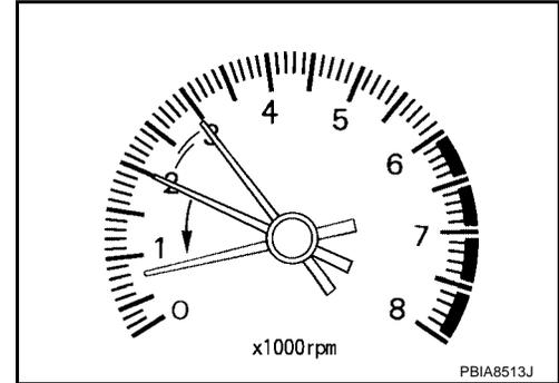
3. Read idle speed in "DATA MONITOR" mode with CONSULT-II. Refer to [EC-76, "IDLE SPEED"](#) .
