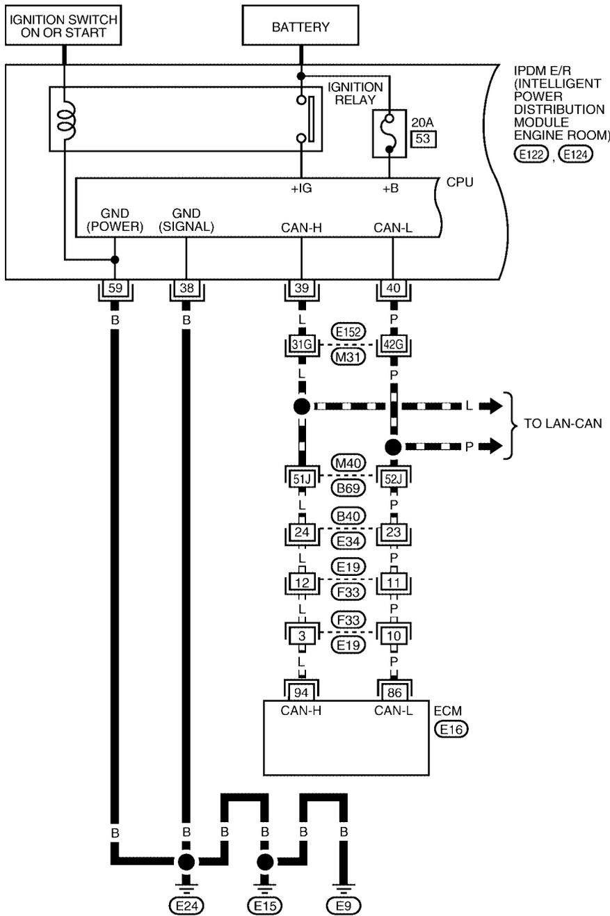
: DETECTABLE LINE FOR DTC
