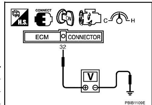
8. Verify that EVAP control system pressure sensor value stays 0.1V less than the value at idle speed (measured at step 6) for at least 1 second.
