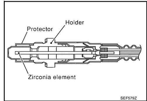
An electronic circuit controls the pump current through the oxygen-pump cell so that the composition of the exhaust gas in the diffusion gap remains constant at  $\lambda = 1$ . Therefore, the A/F sensor 1 is able to indicate air/fuel ratio by this pumping of current. In addition, a heater is integrated in the sensor to ensure the required operating temperature of 700 - 800°C (1,292 - 1,472°F).
