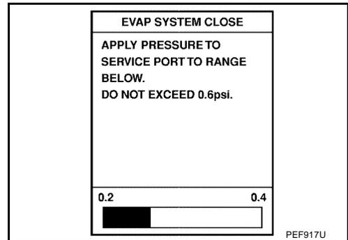
4. Using EVAP leak detector, locate the EVAP leak. For the leak detector, refer to the instruction manual for more details. Refer to [EC-33, "EVAPORATIVE EMISSION LINE DRAWING"](#).
