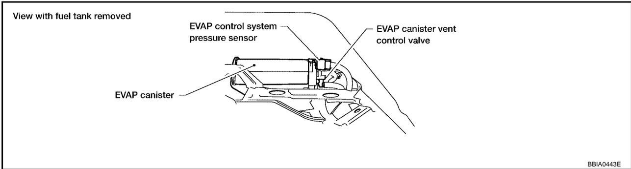
2. Check sensor harness connector for water.
