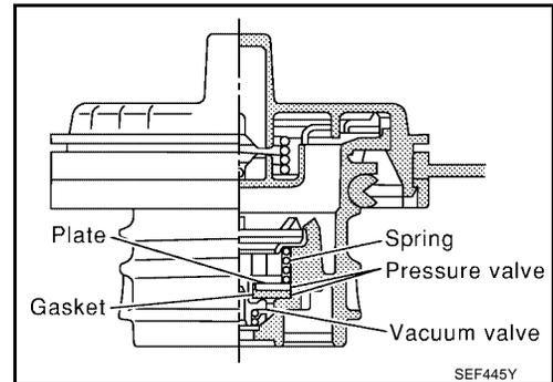
2. Check valve opening pressure and vacuum.
