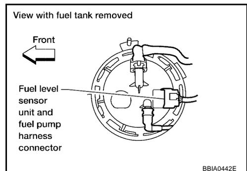
3. Check voltage between "fuel level sensor unit and fuel pump" terminal 4 and ground with CONSULT-II or tester.
