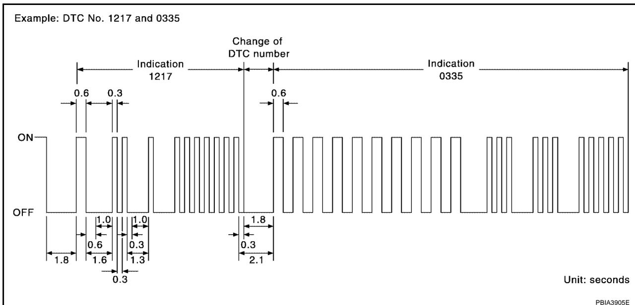
A particular trouble code can be identified by the number of four-digit numeral flashes. The “zero” is indicated by the number of ten flashes. The length of time the 1,000th-digit numeral flashes on and off is 1.2 seconds consisting of an ON (0.6-second) - OFF (0.6-second) cycle.
