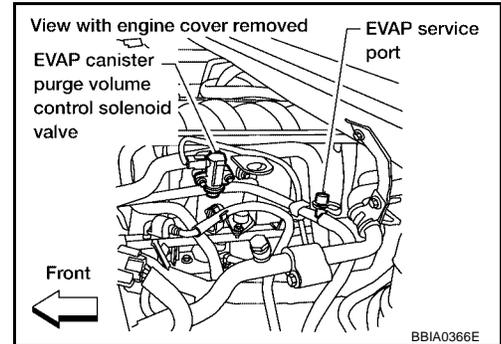
4. Check voltage between EVAP canister purge volume control solenoid valve terminal 1 and ground with CONSULT-II or tester.
