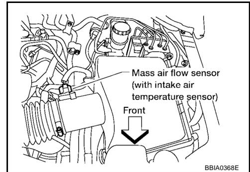
3. Check voltage between MAF sensor terminal 2 and ground with CONSULT-II or tester.
