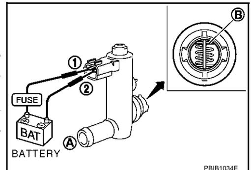
4. Clean the air passage (Portion **A** to **B**) of EVAP canister vent control valve using an air blower.
