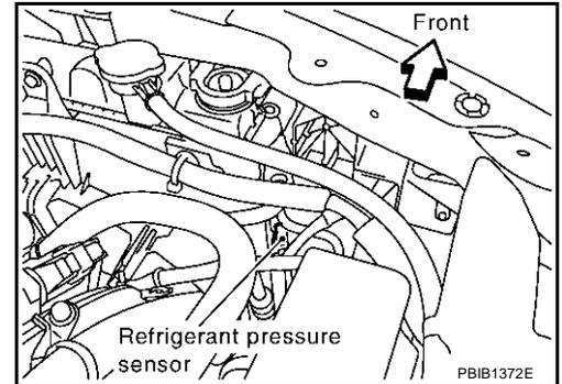
5. Check voltage between refrigerant pressure sensor terminal 1 and ground with CONSULT-II or tester.
