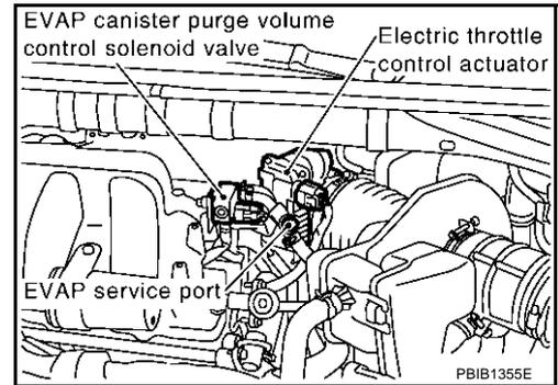
3. Check voltage between electric throttle control actuator terminal 1 and ground with CONSULT-II or tester.
