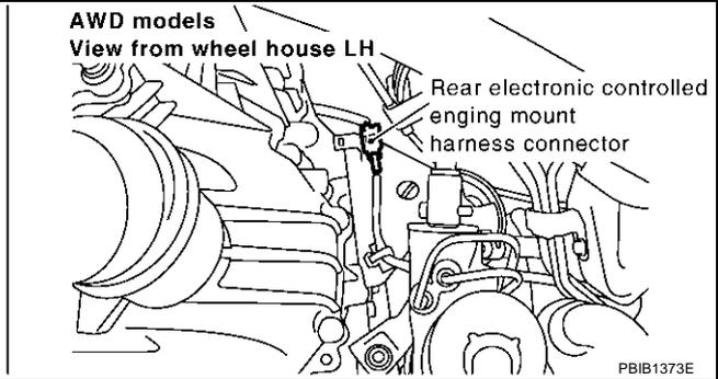
3. Check voltage between electronic controlled engine mount terminal 3 and ground with CONSULT-II or tester.
