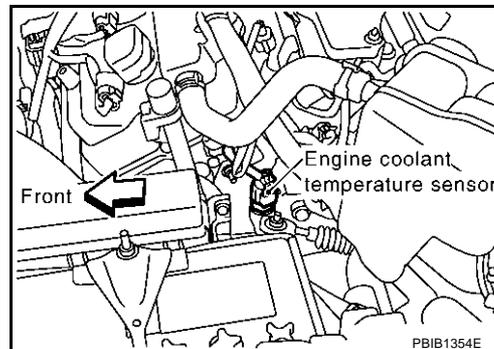
4. Check voltage between ECT sensor terminal 1 and ground with CONSULT-II or tester.
