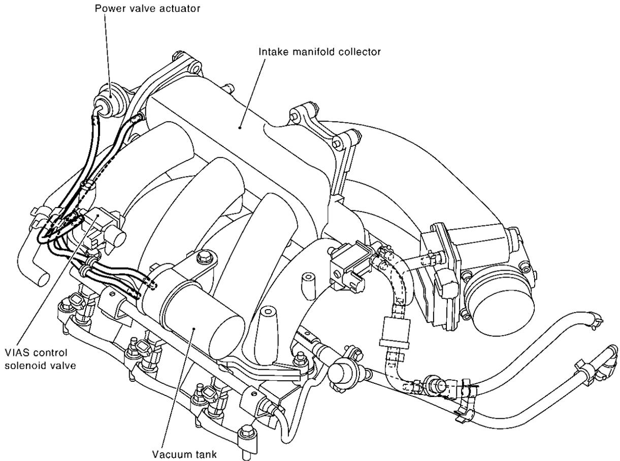
**NOTE: Do not use soapy water or any type of solvent while installing vacuum hose or purge hoses.**
