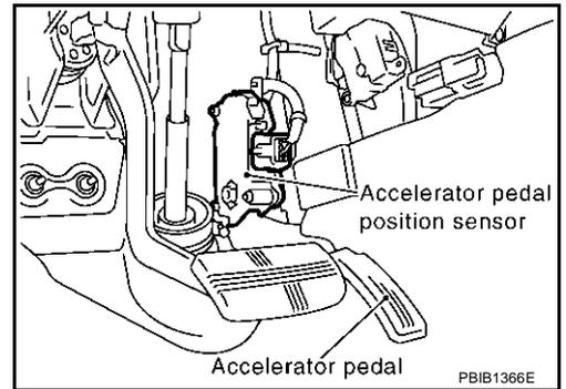
3. Check voltage between APP sensor terminal 2 and ground with CONSULT-II or tester.
