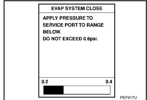
4. Using EVAP leak detector, locate the EVAP leak. For the leak detector, refer to the instruction manual for more details. Refer to [EC-653, "EVAPORATIVE EMISSION LINE DRAWING"](#)
