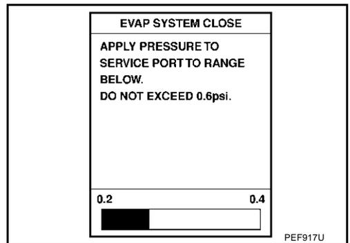
4. Using EVAP leak detector, locate the EVAP leak. For the leak detector, refer to the instruction manual for more details. Refer to [EC-653, "EVAPORATIVE EMISSION LINE DRAWING"](#)
