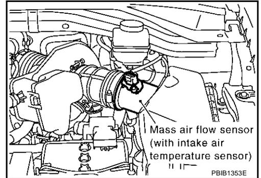
4. Check voltage between mass air flow sensor terminal 5 and ground.
