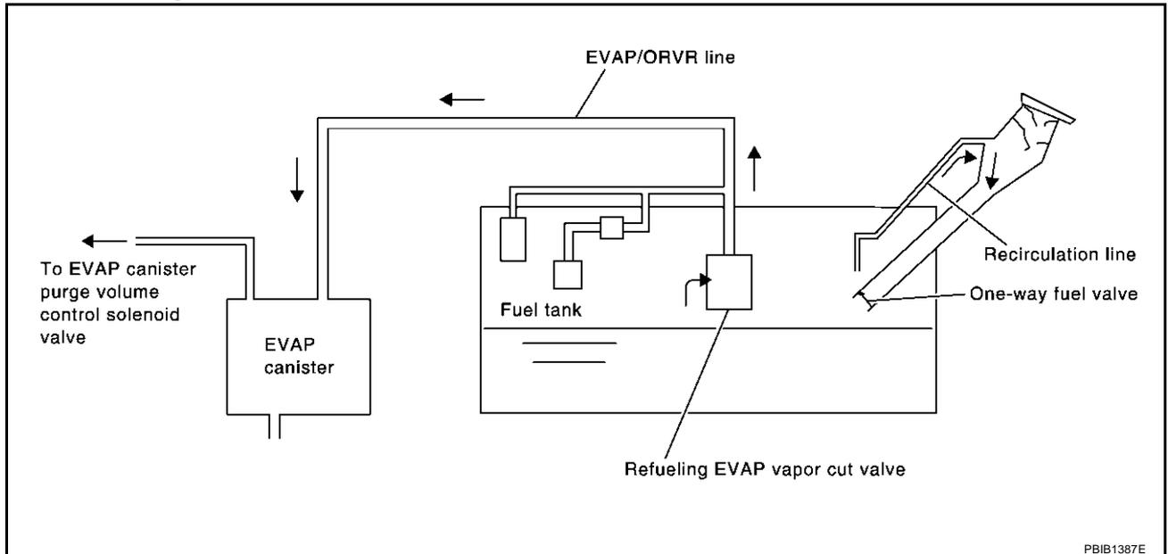
From the beginning of refueling, the air and vapor inside the fuel tank go through refueling EVAP vapor cut valve and EVAP/ORVR line to the EVAP canister. The vapor is absorbed by the EVAP canister and the air is released to the atmosphere.
