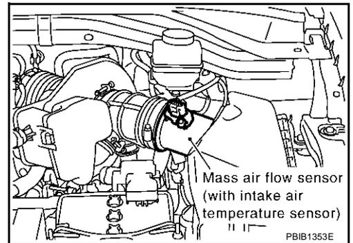
3. Check voltage between MAF sensor terminal 2 and ground with CONSULT-II or tester.
