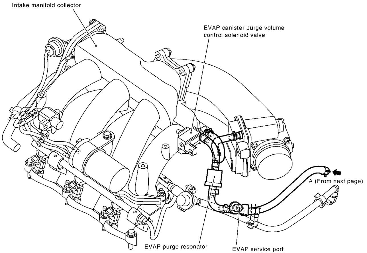
**NOTE: Do not use soapy water or any type of solvent while installing vacuum hose or purge hoses.**
