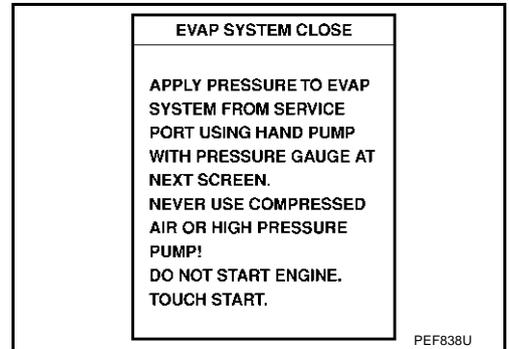
6. Apply positive pressure to the EVAP system until the pressure indicator reaches the middle of the bar graph.
