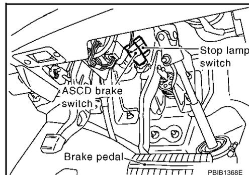
4. Check voltage between ASCD brake switch terminal 1 and ground with CONSULT-II or tester.
