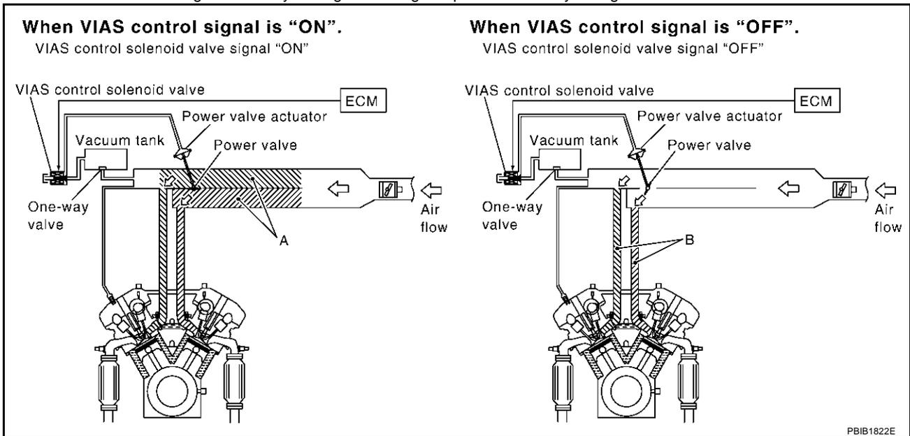
When the engine is running at medium speed, the ECM sends the "ON" signal to the VIAS control solenoid valve. This signal introduces the intake manifold vacuum into the power valve actuator and therefore closes the power valve.
