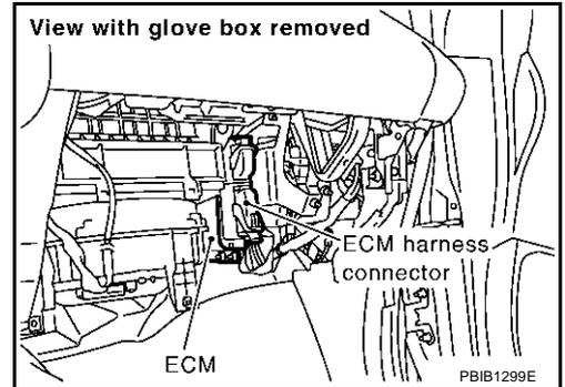
3. When disconnecting ECM harness connector, loosen it with levers as far as they will go as shown at right.
