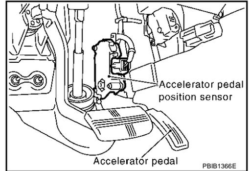
3. Check voltage between APP sensor terminal 4 and ground with CONSULT-II or tester.
