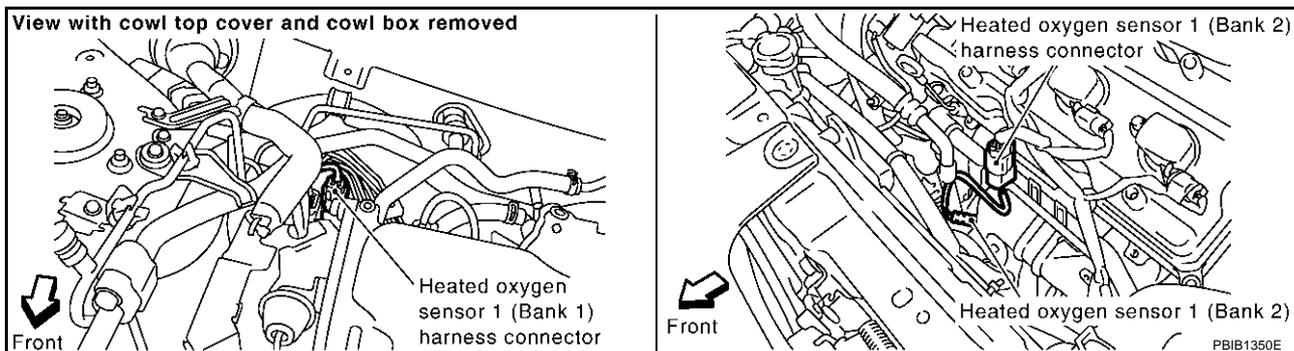
2. Check harness continuity between HO2S1 terminal 4 and engine ground.
