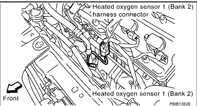
2. Check harness continuity between HO2S1 terminal 4 and engine ground. Refer to Wiring Diagram.
