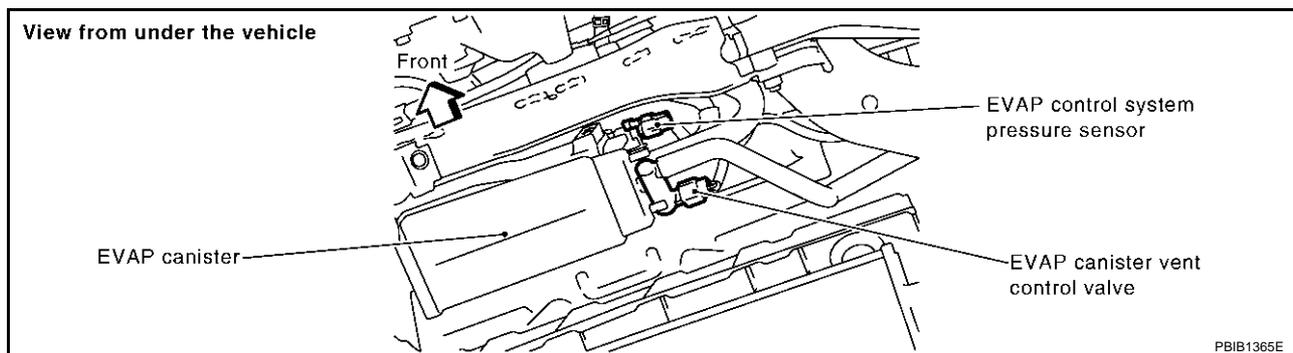
2. Check sensor harness connector for water.
