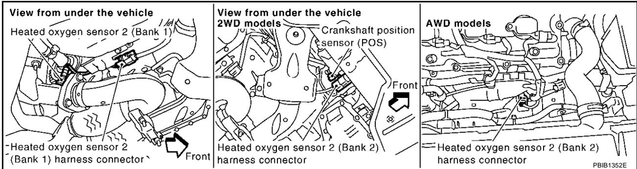
3. Check harness continuity between HO2S2 terminal 4 and engine ground. Refer to Wiring Diagram.
