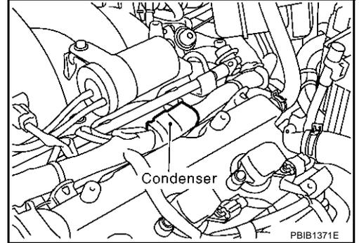
4. Check voltage between condenser terminal 1 and ground with CONSULT-II or tester.
