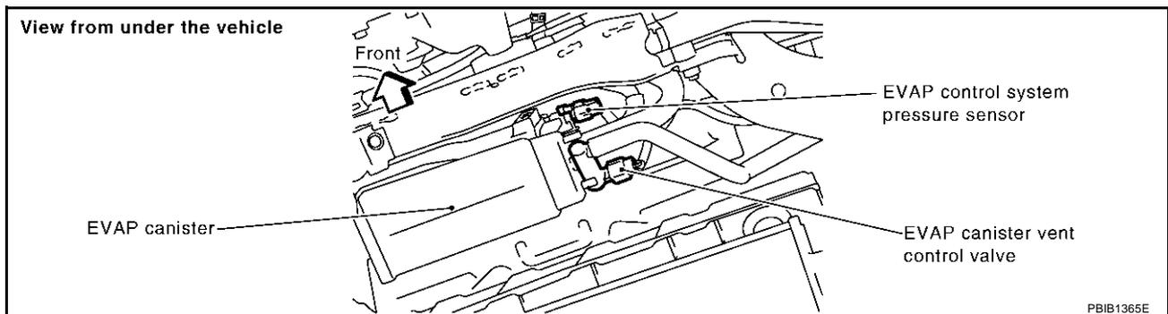
2. Check sensor harness connector for water.
