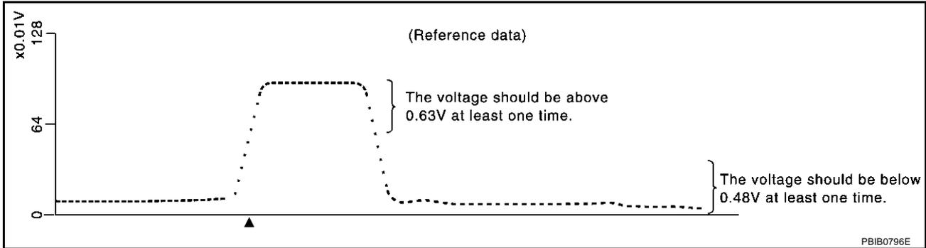
"HO2S2 (B1)/(B2)" should be above 0.63V at least once when the "FUEL INJECTION" is +25%.
