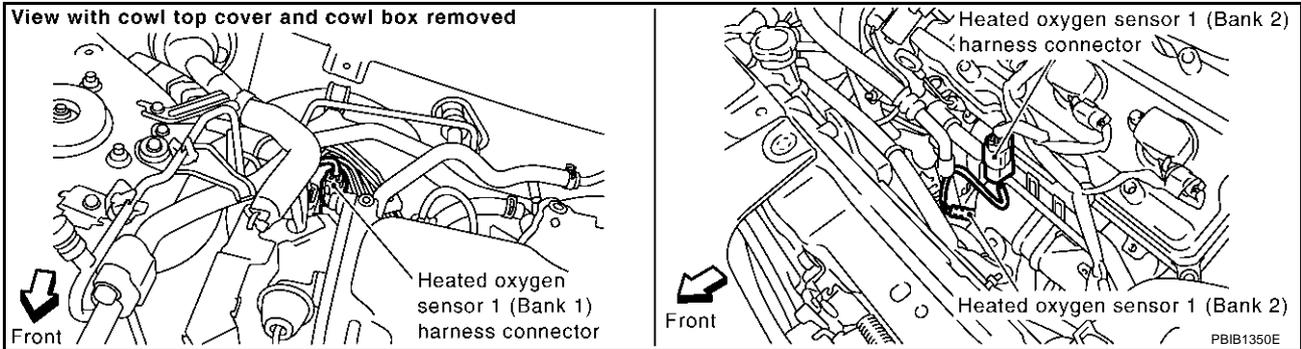
3. Check harness continuity between HO2S1 terminal 4 and engine ground. Refer to Wiring Diagram.
