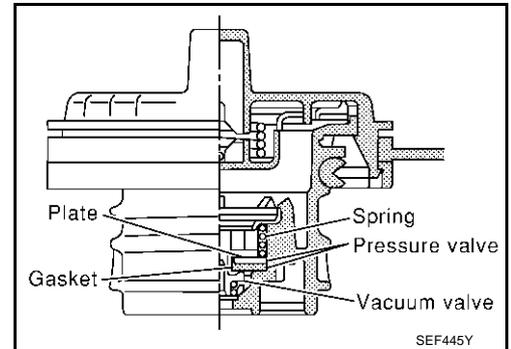
2. Check valve opening pressure and vacuum.
