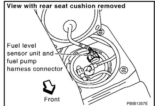
4. Check voltage between "fuel level sensor unit and fuel pump" terminal 4 and ground with CONSULT-II or tester.
