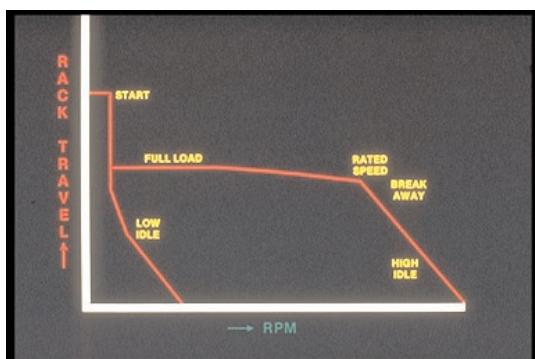
8. . . let's look at a similar graph of these governing points showing how rack travel changes with RPM. In the calibration of governor and pump, both rack travel and delivery are checked against pump RPM.
