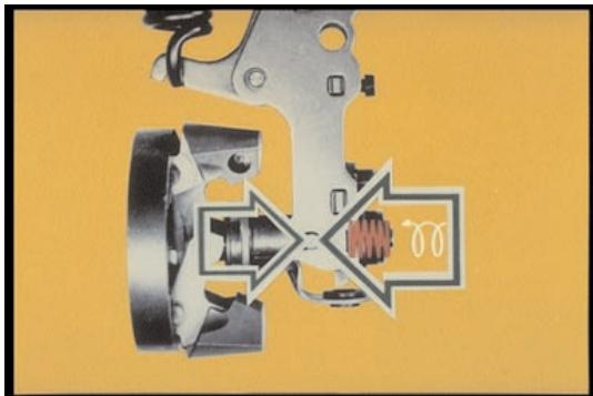
49. Turning the collapsed torque capsule against the guide sleeve will increase delivery. How will it increase delivery?
