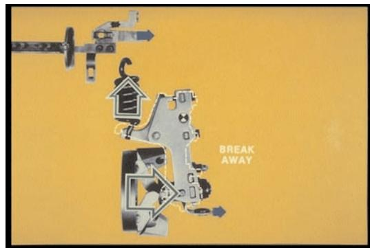
55. . . flyweight force moves the tensioning lever, stretching the main spring. Guide sleeve movement pulls the rack.
