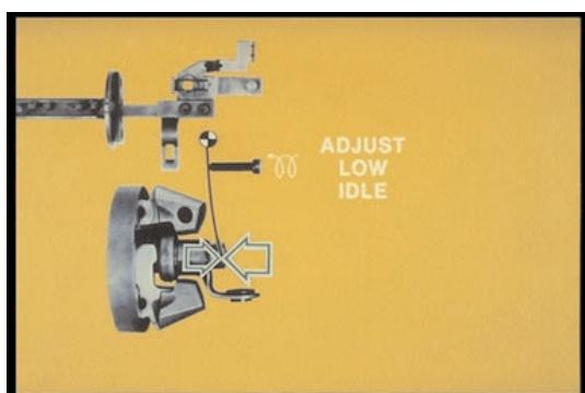
24. When you screw in the internal adjustment for low idle, what happens? You increase the leaf spring force on the guide sleeve and the flyweights.
