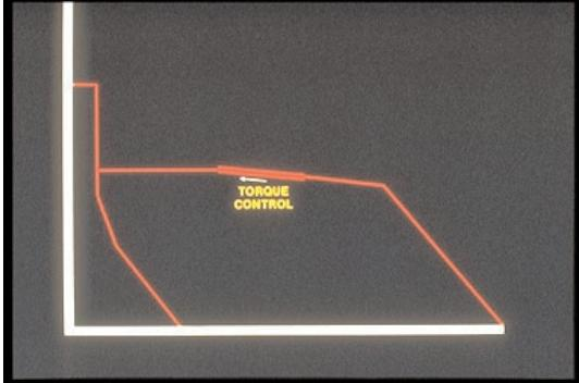
45. So, in the RW calibration, torque back-up is checked like this. The torque control capsule will expand at lower RPM, pushing the rack up to full load.
