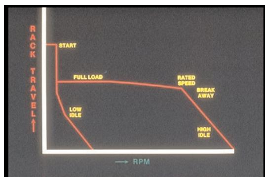
71. . . to control rack travel and regulation for low RPM's, high RPM's and full load . . .
