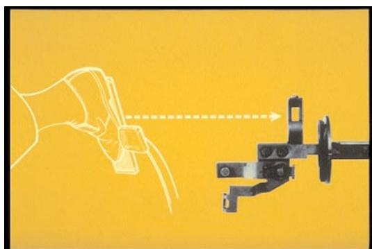
6. We know that, at part loads, the accelerator controls the engine — controls the rack through the RW governor linkage.
