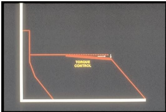
43. . . called torque control. At full load, with an RPM increase, torque control will allow flyweights to pull the rack like this — reduce the full load limit. As RPM increases toward rated speed . . .
