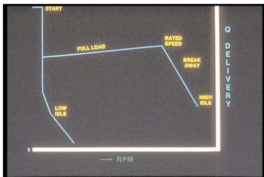
7. As far as the engine is concerned, the governor controls the pump "Q" quantity or delivery at start, low idle, full load, rated speed, breakaway, high idle — all those points you're already familiar with. But instead of looking at how pump delivery changes with RPM . . .
