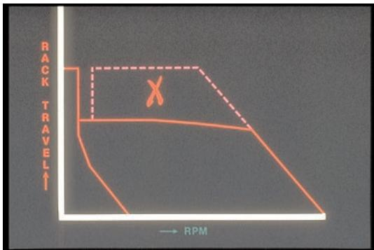
66. Above cranking RPM, the rack cannot travel above the full load limit. But for emission control, that full load limit may be reduced with altitude.
