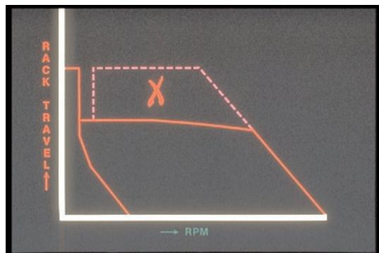
64. At all normal engine running speeds, this follower cam is moved by the flyweights so the finger on the full load stop limits rack travel.
