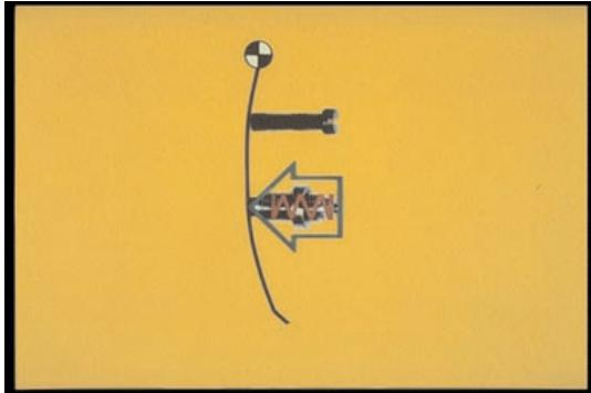
33. Idle regulation is changed by the bumper spring. It just touches the leaf spring at normal idle. So, during unloading, it adds to the spring forces against the flyweights.
