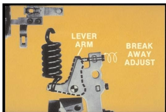
56. When you turn in the screw for breakaway adjustment, the lever arm stretches the main spring so it pulls harder on the tensioning lever.
