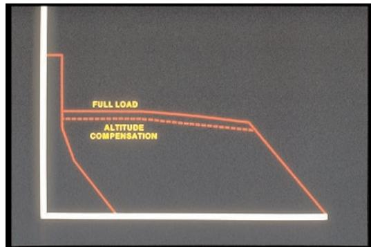
69. Depending on altitude, full load rack travel is reduced by altitude compensation.
