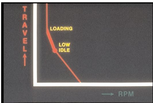
27. When loading causes a loss of RPM, how does the governor increase rack travel for greater fuel delivery?
