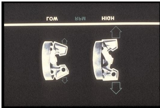
9. At low RPM, small forces are developed by governor flyweights. As the RPM gets higher, flyweight forces are greater.
