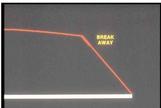
51. This is called breakaway. When the engine revs beyond rated speed, the governor will pull the rack.
