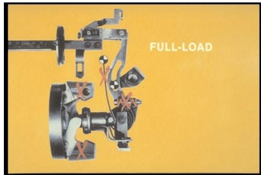
38. . . full load limitation is not a balance of forces; the flyweights are not controlling — the springs are not controlling.
