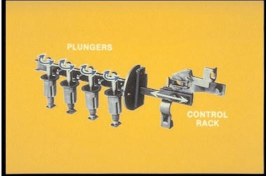
16. Just remember, flyweight force tends to pull the rack for less delivery; governor spring forces tend to push the rack into the pump.
