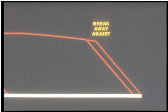
57. This breakaway adjustment means higher RPM and greater fly-weight force. After breakaway . . .
