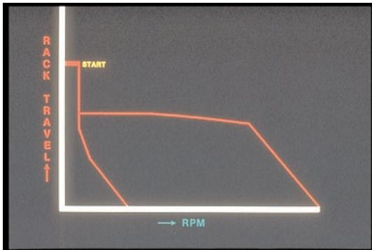
17. What do we need for start-up? That's right, pushing the rack full in for greatest fuel delivery.
