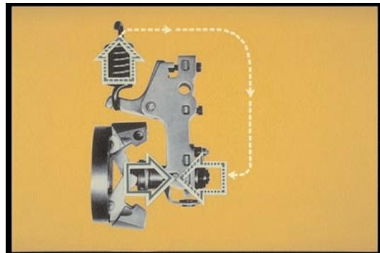
53. Just before breakaway, the main spring continues to oppose the flyweight force, working through the lever arm and the tensioning lever.
