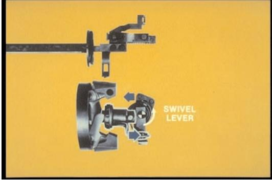
13. With increasing speed, the flyweights move the guide sleeve with its arm to the right, causing the swivel lever to swivel to the left.
