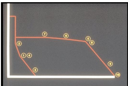
60. In order, one, low idle; two, loading; three, unloading; four, bumper spring. Then, at higher RPM's, five, rated speed; six and seven, torque control and full load; eight, breakaway; nine, high idle; and ten, fuel cut-off.
