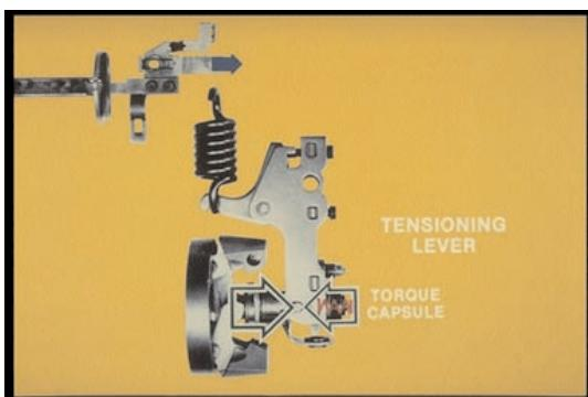
44. . . flyweight force overcomes spring force of the torque capsule in the tensioning lever. This pulls the rack to reduce fuel delivery.
