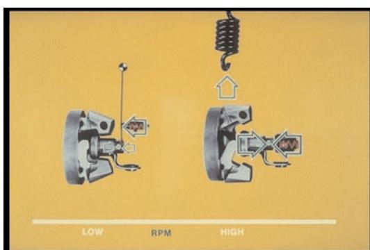
12. At low RPM, flyweight force is small; it can be countered by small springs, ones you can easily compress with your fingers. At higher RPM, greater flyweight force is countered by heavier springs. In either case, when flyweight force overcomes spring force, how does that move the rack?
