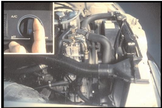
29. Unloading could be turning off an accessory or any way of reducing load on the idling engine.
