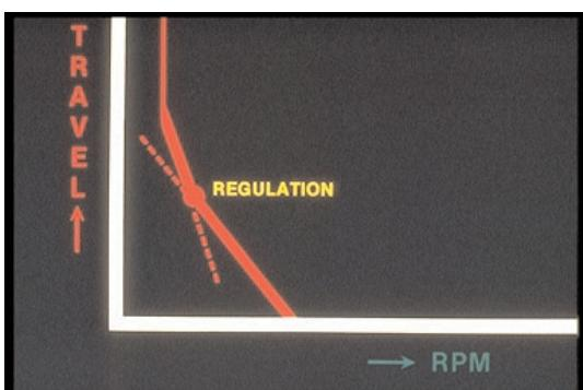
32. Stable RPM comes from regulation — that is, how much rack travel for a certain RPM change. In this RW, loading has a different regulation, or slope, than unloading.
