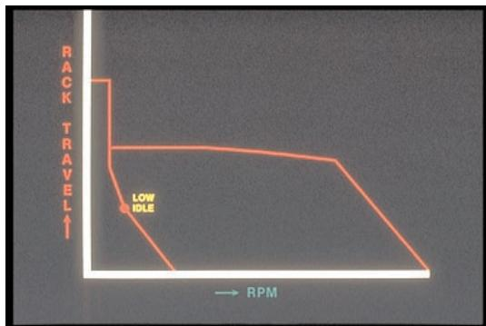
22. At the specified low idle RPM, this rack travel should deliver the proper quantity of fuel.
