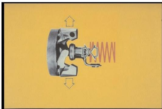
10. The flyweight forces work to push the guide sleeve to the right. Spring force tends to push the guide sleeve the other way.
