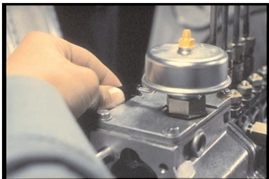
68. In most cars, altitude compensation is automatic; it can be manual in some vehicles. Vacuum is pulled on the test bench to simulate altitude.
