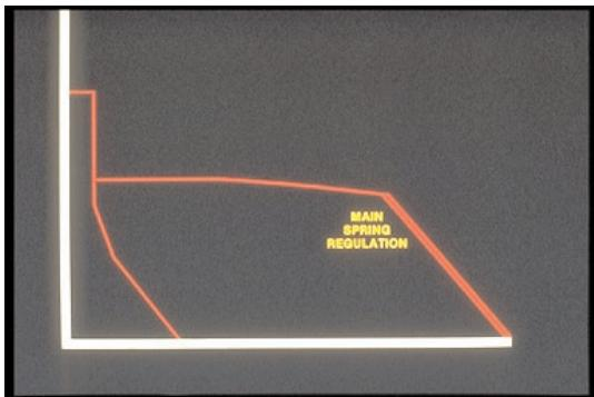
. . . as RPM rises, main spring regulation determines how the rack is pulled to high idle, and finally to cut-off.
