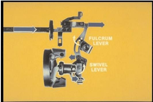
14. This movement causes the fulcrum lever to pivot in the opposite direction, moving the rack. It's easy to remember — when the sleeve moves right, the rack moves to the right. Sleeve left, rack left. From now on, we'll simplify our flyweight rack story without this linkage.
