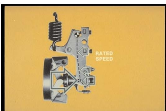
52. At rated speed, flyweight force has overcome all the spring forces in the tensioning lever, but not the main spring.
