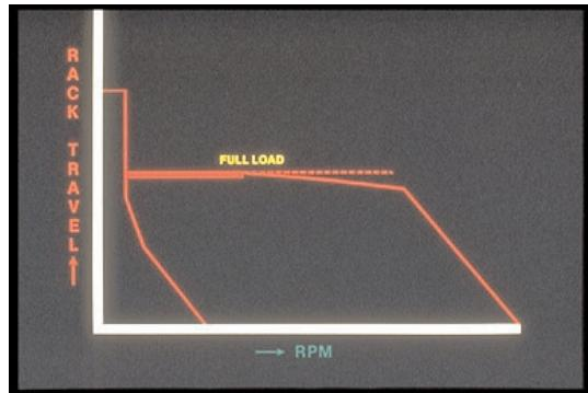
37. ... must limit full load rack travel to this heavy red line to avoid too much fuel. This could overstress the engine; it could also cause smoke. At these RPM's . . .
