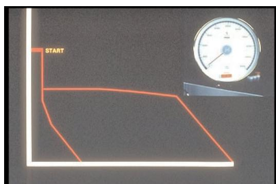
63. But at higher RPM's, the starting quantity cut-out must prevent rack travel above full load.
