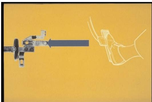
18. At start, the control rack is pushed full in for max. fuel delivery.
