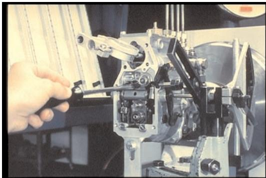
25. On the test bench, this adjustment changes low idle fuel delivery.
