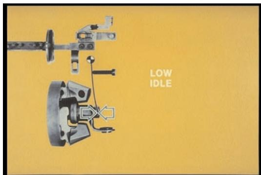
23. The rack is positioned at low idle as the leaf spring force counters the flyweight force.
