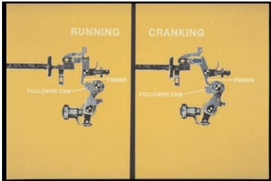
65. In comparison, at cranking RPM, the guide sleeve moves left so the swivel lever lowers the follower cam. The finger drops into the slot so the rack can be pushed to start quantity.
