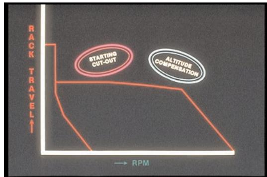
62. With the pump at cranking RPM, the governor should permit the full starting rack travel.
