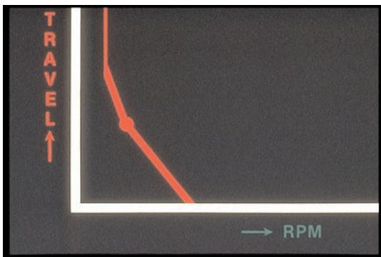
34. You have seen how low speed governor settings control rack travel at low idle. Above low idle . . .
