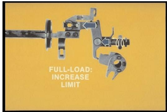
40. Turning in the full load screw will increase the limit — the amount the rack can travel.
