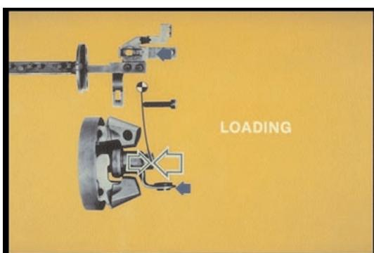
28. As the engine slows, there is less flyweight force. So the spring force can push the sleeve; and through levers, push the rack in the same direction. If this is loading, what's unloading?
