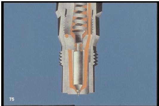
75. . . and, on pressure drop, the spring and pressure-spindle snap the needle shut without dribble or smoke.
