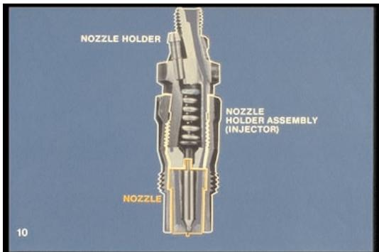
10. Each injector is made up of a nozzle holder and a nozzle; the whole thing is sometimes called a nozzle-holder assembly.
