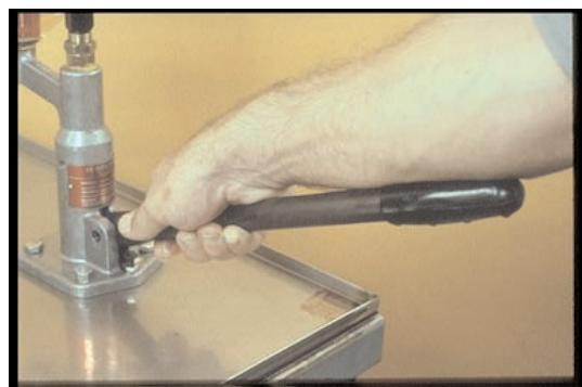
71. You know how to apply measured pressure — for opening pressure or leak testing.
