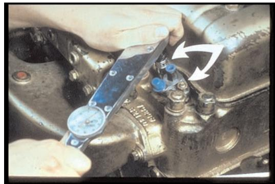
70. The differences between installing and torquing the different kinds of nozzle holders as well as what happens if you under-torque or over-torque.
