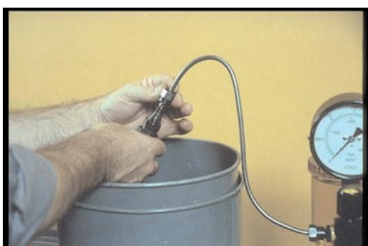
36. . . . you will test it, as shown in another program in this series. If it checks out, reinstall it in the engine. If it does not, replace it, or send it to a diesel specialist for reconditioning.
