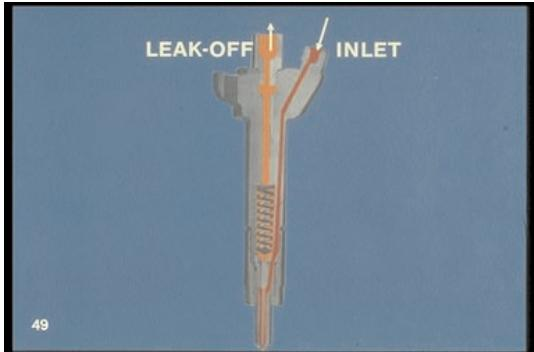
49. Still another job of the holders is to provide fuel connections for inlet, or high-pressure fuel -- and leak-off, or return-fuel. Be sure you know which is which -- sometimes, as in this KB holder, the high-pressure inlet is on the side,
