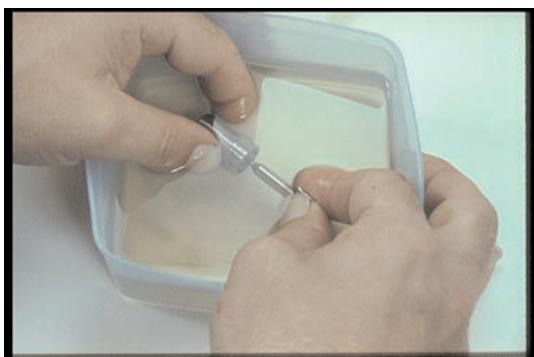
67. For your final check of the nozzle, assemble the nozzle under the test oil, like this.
