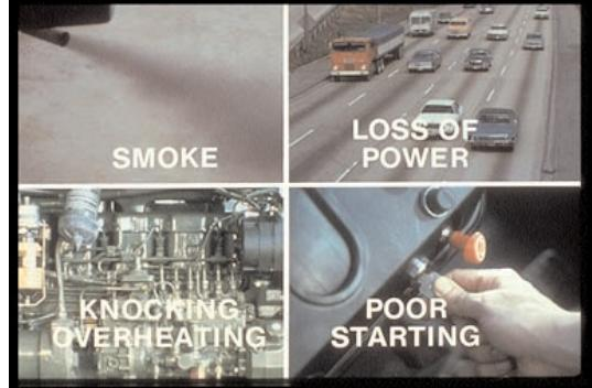
13. Most likely, engine problems are causing these symptoms—but these can also be injector symptoms. How would you check out whether injectors are at fault—and which ones?
