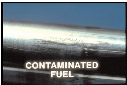
52. When you see this, you're seeing the evidence of contaminated fuel. Contamination damaged this needle valve; and could cause nozzle-seat damage. Contaminated fuel is a problem the operator's got to deal with.
