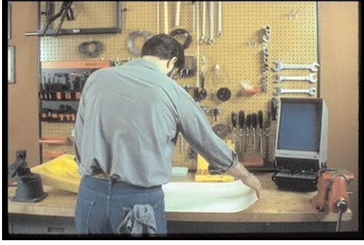
8. In your clean room, use clean, smooth paper as a work surface. If you don't have a dust-free place to work, you probably should not be disassembling injectors.
