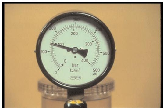
39. Be sure to check your specs for proper test pressure; here's a special case — use 95 bar to leak-test a nozzle used in Chevrolet 6.2 liter engines. Stop now to review leak test.
