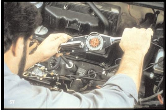
57. The KC holder, for pintle nozzles, is simply screwed into the cylinder head. Provided it's properly torqued, it will spray in the right direction. The direction of the spray is straight in line with the nozzle axis.
