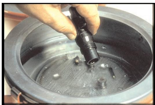
40. With carbon loosened, clean the nozzle-nut. Don't sand-blast — that's too abrasive.
