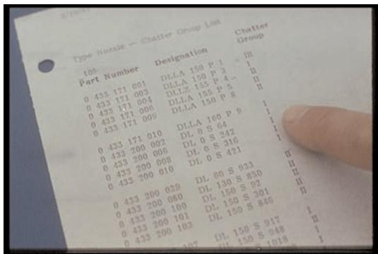
58. When you check the specs for testing, you'll find three chatter groups which define chatter and spray patterns according to pumping rates. Group one is widely used in the United States and Canada. Groups two and three differ mainly in lack of chatter at intermediate pumping speeds.
