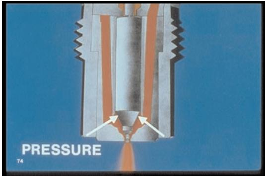
74. You've seen how high-pressure fuel lifts the needle valve so the nozzle can deliver fuel;
