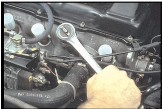
25. Some injectors unscrew—like this. Others come out by removing their clamp nuts and using a puller. Cap all injectors not being removed.
