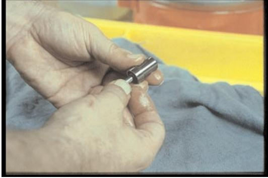
29. So wet your fingers with test oil. And when you join these mated parts, dip them in test oil; avoid damage from finger-acid or from any tiny dust particle in the air.
