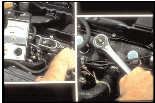
13. Use the injector-tester when you're troubleshooting the engine and you suspect one or more injectors.
