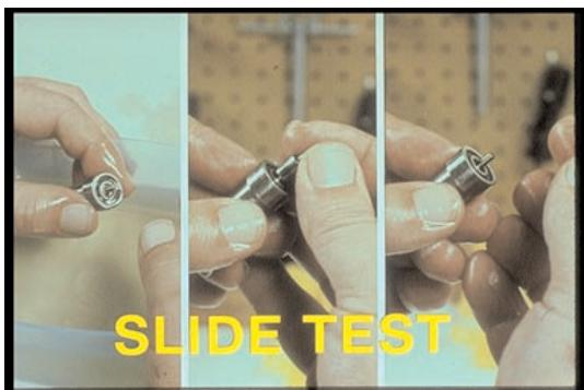
68. In the slide test, wet the needle; pull the needle out about one-third and hold the body at 45 degree slant like this. The needle should slide in of its own weight. If the nozzle fails this test, clean it and try it once more. If it fails again, replace it. Stop now for review of inspection.
