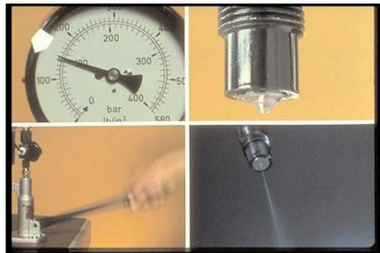
78. You know how to test injectors for opening-pressure — leak-test — chatter — and spray-pattern.
