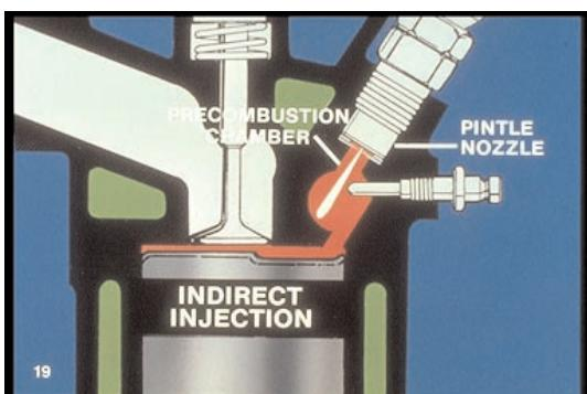
19. To distribute fuel into the precombustion chamber of this indirect-injection automobile engine, the pintle nozzle delivers a narrow spray pattern; injected fuel ignites in the prechamber; the burning air-fuel mixture spreads to the main chamber above the piston. Stop now for review of what nozzles do.
