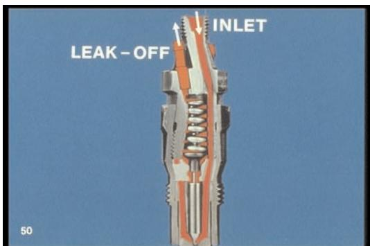
50. . . and sometimes, as in this KC holder, the high-pressure inlet is in the center. Leak-off fittings connect the injectors in series to each other and return fuel to the tank.
