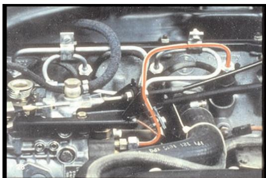
28. . . . high pressure fuel, shown in red, is delivered to the injector in a fraction of a millisecond.
