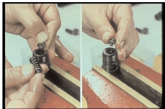
72. With the holder body upside down, be sure these parts are wet with test oil as you assemble the shims, spring and pressure spindle like this.
