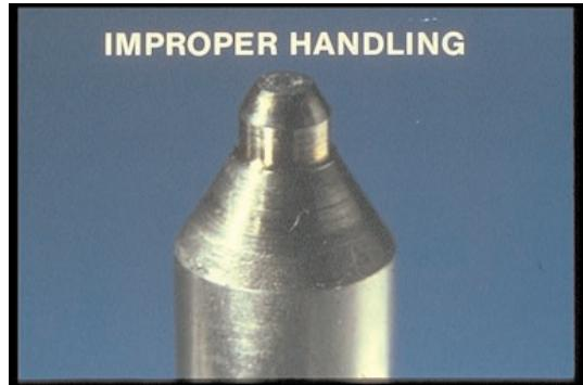
53. Suppose you find a needle valve with a broken pintle like this — or a bent pintle? You'll know the nozzles were dropped or mishandled during assembly or installation. Improper handling is a problem for service technicians.
