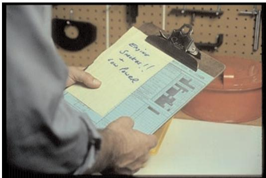
10. Check the work order for engine complaints. Most injector complaints are not injector-problems — they're probably engine-related. That's a good reason to keep track of injectors by cylinder number.
