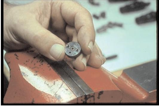
61. If you want to lap these machined surfaces of the nozzle-holder, the locating pins must be removed; and replaced after lapping.
