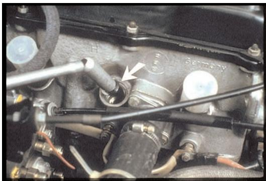
26. With the injector removed, use a magnet like this to remove a steel heat shield. Some engines use copper gaskets—non-magnetic; you'll have to fish them out. And in some engines, such as the Chevrolet 6.2 liter, you won't find a separate heat shield in the recess—it's inside the injector.
