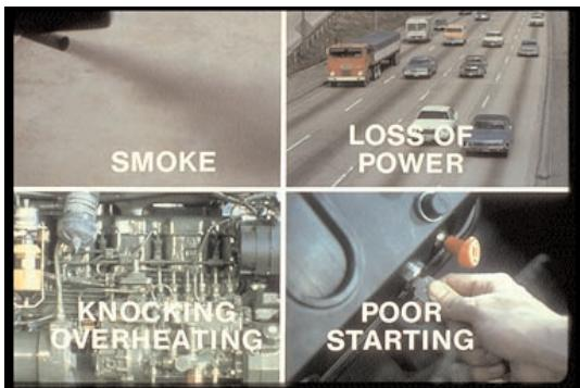
11. Whether the complaint is smoking, loss of power, overheating or knocking, or poor starting, you may be able to relate a specific injector to a specific cylinder or injection pump element.
