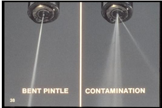
38. An off-center spray pattern is the result of a bent pintle, probably mishandled; fuel may not burn well. Or the spray pattern may be ruined from contamination of a pintle; the nozzle should be cleaned or replaced.
