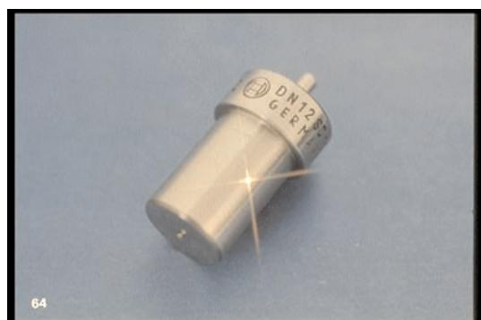
64. No wonder these gems need clean fuel, clean air, and clean service facilities. Unlike spark plugs, injectors should not be pulled just to be looked at.
