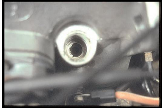
45. This injector recess is clean, especially around the inside where the heat-shield touches. If it were not, it might need reaming to remove the carbon; check instructions from the engine manufacturer.
