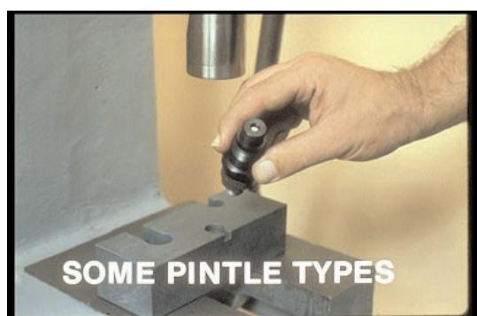
24. For this kind of pintle-type nozzle such as used on V-W and Mercedes, it's simpler. Clamp it in brass jaws, loosen the nozzle nut and remove it.
