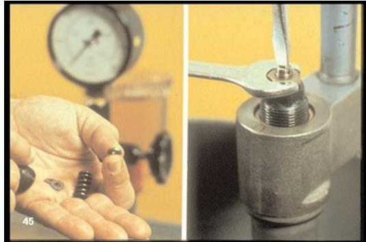
45. With shims, in some injectors. The thicker the shim, the greater the spring pressure. In other injectors, spring pressure is adjusted with a screw. So one job of the nozzle-holder is to apply adjustable spring pressure on the nozzle-needle.
