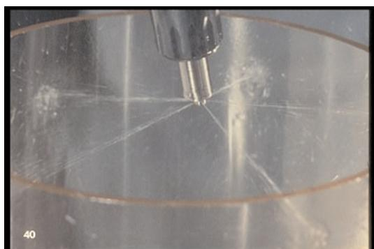
40. . . . with this poor spray performance. What began as a good nozzle has been damaged by improper handling, perhaps by being lapped, or contaminated -- perhaps by improper cleaning of the needle seat and spray holes. Result -- poor engine performance: smoke, loss of power, poor economy.
