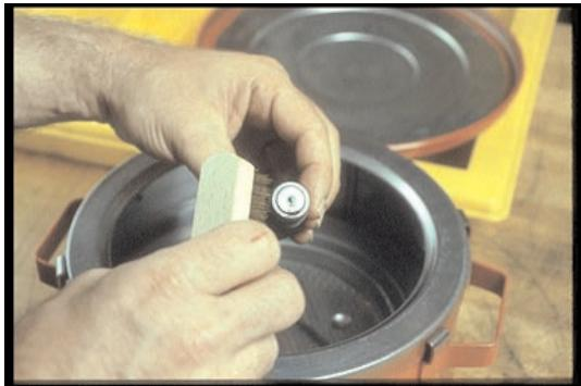
9. After cold-soaking nozzles in solvent, use the brass brush to clean the tip, removing any carbon residue.
