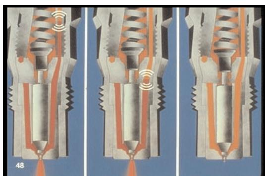
48. At port-opening in the pump, in a fraction of a millisecond, pressure drops at the tip. The spring snaps the needle shut. The valve seats with a sharp cut-off -- no drip, no dribble.
