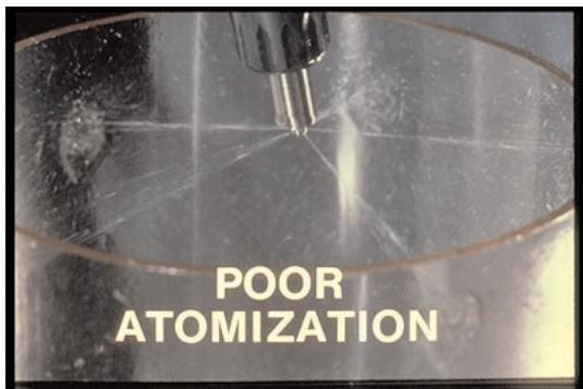
66. In a hole-type nozzle, poor atomization can cause this kind of pattern.
