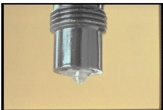
36. If a drop forms, count the time. If the drop falls off in 10 seconds, clean and retest the nozzles; if it still drops one drop, the nozzle should not go back in the engine.
