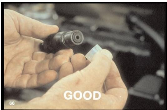
66. If you must remove an injector (to test or replace it), be sure your shop is good and clean -- on a scale of good, better, best.
