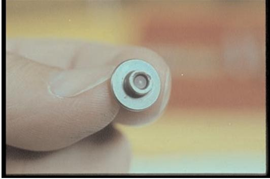
64. Be sure the lower end of the spindle is straight — not cracked or broken. If the spring seat is worn, you'll need to replace the assembly. This one's OK.
