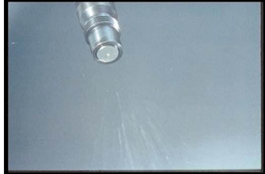
45. You will hear a soft chatter, very soft. But as you can see in this high-speed photography, the spray pattern is stringy, with split streams. Does this mean a bad injector? No. At slow pumping, neither a bad pattern nor a bad sound means a bad injector.
