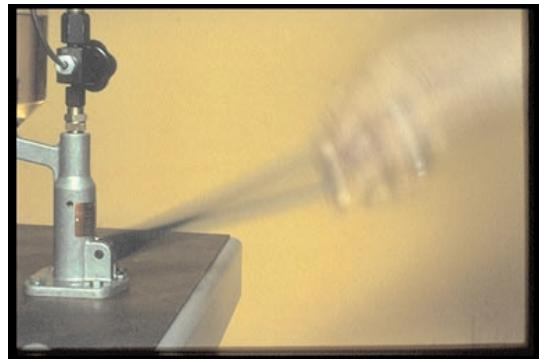
21. Rapid strokes bleed the system; they could also damage the gage. Stop now for review of preparation for testing.
