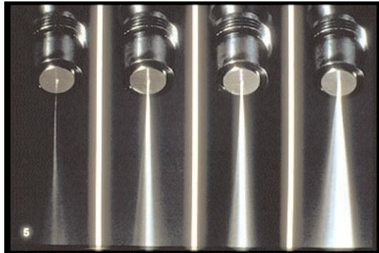
5. Each time they operate -- from start to finish of delivery -- injection duration can be as little as one-thousandth of a second, one millisecond!
