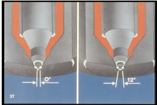
37. The angle of the pintle determines the spray angle. Zero degree means straight, almost no spray angle, in contrast to a typical 12 degree angle.
