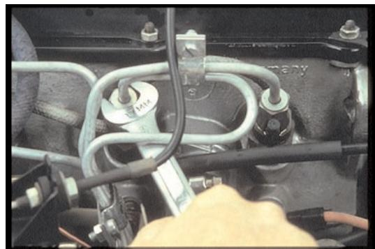
16. With idle speed recovered, loosen the next fitting and listen. When speed does not change or changes very little, you've probably found a faulty injector; it's a little like shorting out spark plugs on a gasoline engine. With other pumps, you may have to use a pyrometer instead of loosening fittings.
