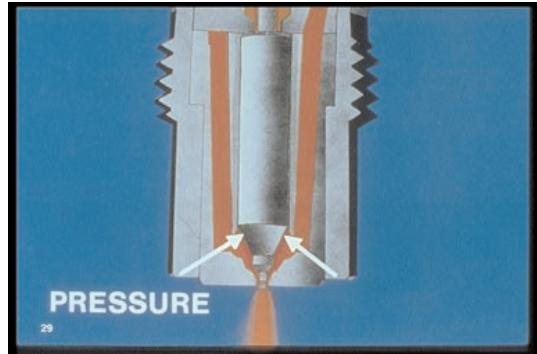
29. In this pintle nozzle, high-pressure fuel applies lifting pressure here against the spring-loaded needle. When fuel pressure is greater than downward pressure, it lifts the needle . . .
