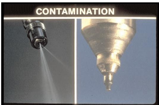
52. Here's a pattern resulting from contamination. Remember, don't reject a nozzle by its sound.
