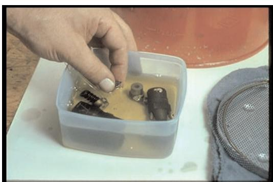
44. . . . dip the nozzles and holders in clean test oil. Stop now for review of cleaning operations.
