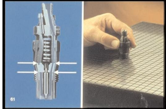
61. You'll find precision lapped surfaces between the nozzle-holder body, the intermediate plate and the nozzle. These are high pressure seal-areas, so each part should be clean and perfectly flat.
