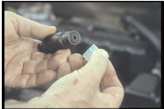
29. Be sure to cap removed injectors—all openings. Don't damage the needle at the tip.
