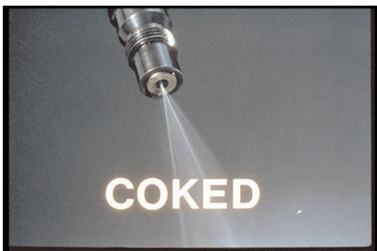
75. Even when you pump fast, a coked nozzle will show a poor spray pattern like this.
