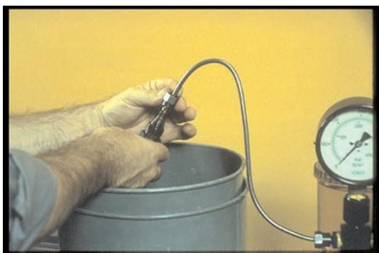
12. Before disassembly, test the injector, as shown in another program. You may find it's not an injector problem at all — or the injector needs a new nozzle.
