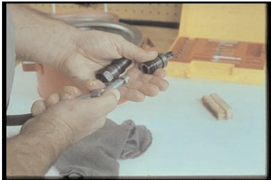
41. After washing in solvent, blow the parts dry and dip in clean test oil.
