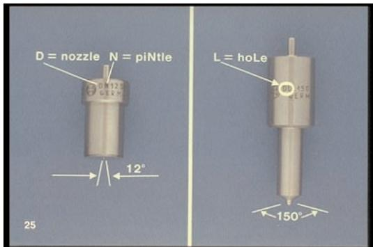
25. Compare the pintle-type to the hole-type. On a hole-type nozzle, you'll see D for nozzle, and L for hole. The 1-50 indicates the spray angle; notice it's much wider for direct injection.
