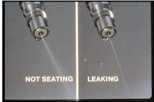
53. When a nozzle is not seating, its spray-pattern may look like this; or when it's leaking, like this below opening pressure. It's two views of the same problem. Clean the nozzle or replace it.
