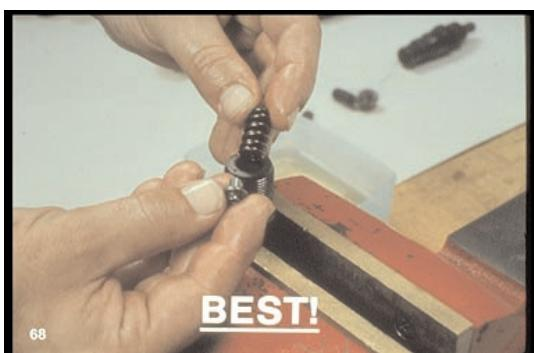
68. Be sure you have the best clean shop if you disassemble an injector. You really need separate "clean room" facilities before disassembly. Dirt is the enemy of injectors! Stop now for review.
