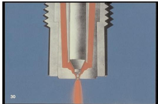
30. . . . and delivers fuel. When pressure at the pump is relieved by port-opening,
