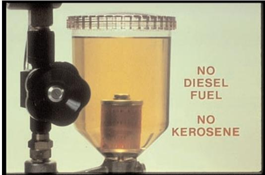
17. Diesel fuel is not recommended; when it gets old, it may form gum. Kerosene is usually forbidden; it's so flammable, it's unsafe in spray-testing.
