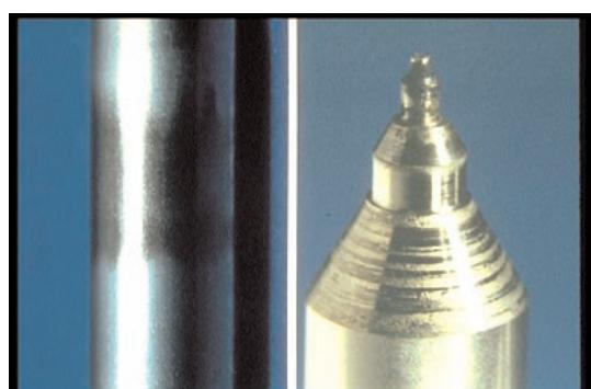
48. On the finished surface, you'll probably find marks like this; the pressure-shoulder is normally rough. This needle valve is OK.
