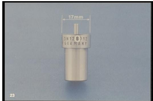
23. You can tell the size by this code letter. For example, a 17 millimeter nozzle -- the most common size -- is indicated by this letter, S.
