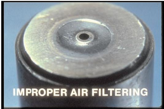
57. Improper air filtering allowed dirty air to erode and ruin this nozzle. A torn filter should be changed without delay.
