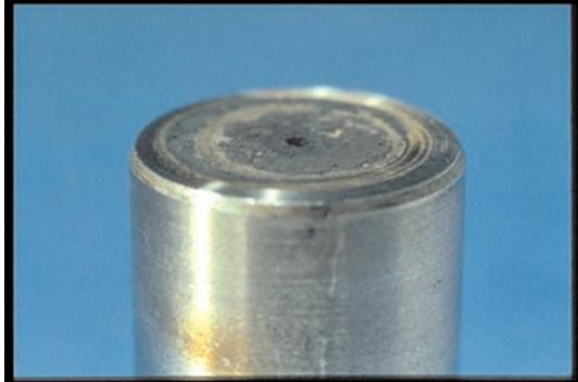
49. On the nozzle-tip, you may find normal, hard carbon, which can be removed. This nozzle-body is OK.
