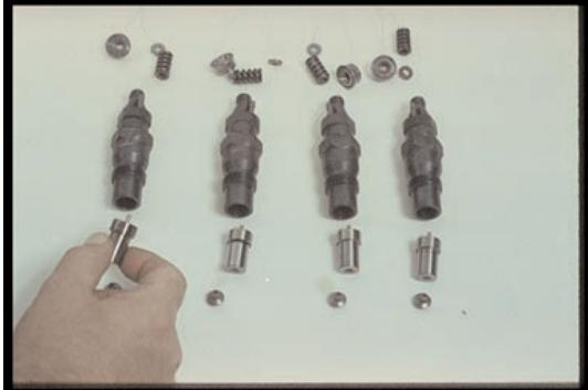
30. You may spread them like this, organized on clean paper, or in a pan of clean test oil, with nozzle nuts reinstalled to protect the lapped surfaces of the nozzle holder. Stop now for review of disassembly.
