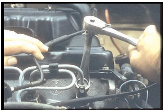
66. When removing lines, you don't want to bend them so you loosen line clamps first.
