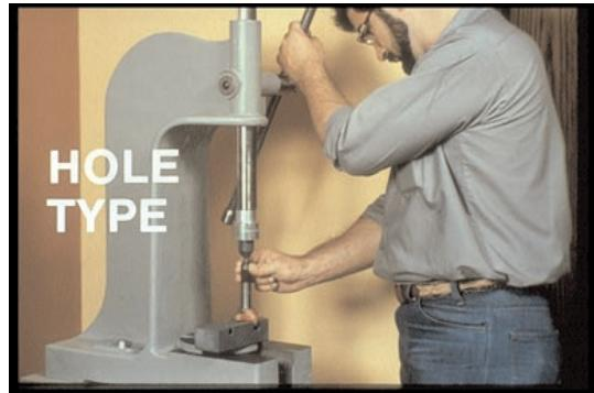
21. For many injectors, including all hole-types, you have to relieve the pressure of the adjusting spring by applying downward pressure like this on the injector in this fixture.
