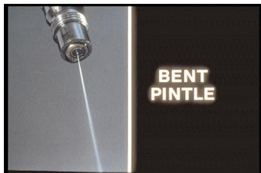
54. This spray-pattern is caused by a bent pintle, the result of care-less handling. And if the handling is rougher,
