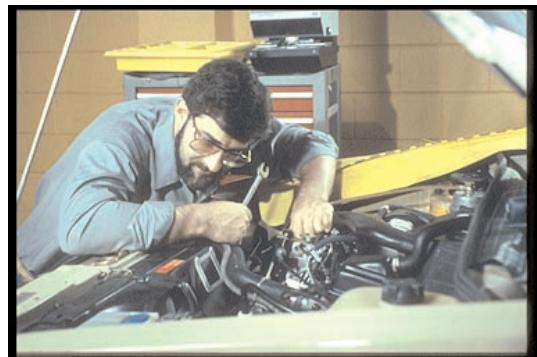
14. One way is to listen to the idling engine as you cut out injectors, one at a time. This may not work with all injection pumps, but with Robert Bosch pumps,
