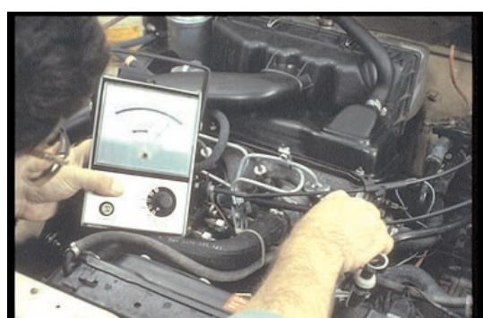
64. If you're checking injectors, you know how to check for rpm drop, with a tach or by ear as you loosen each injector in turn.
