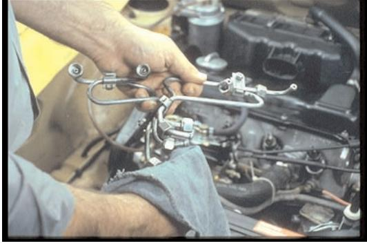
56. Keep the high-pressure lines clean, and wipe the ends before installation, just to be sure.
