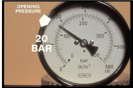
29. At twenty bar below opening pressure of this nozzle, you want to be sure it does not open enough to drip one drop.
