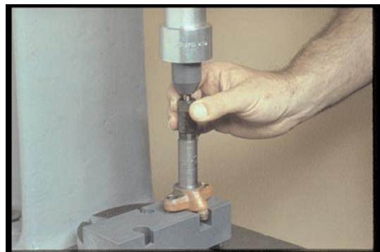
23. In the same way, some pintle type injectors should be relieved by pressure on the nozzle to avoid contamination with metal chips.
