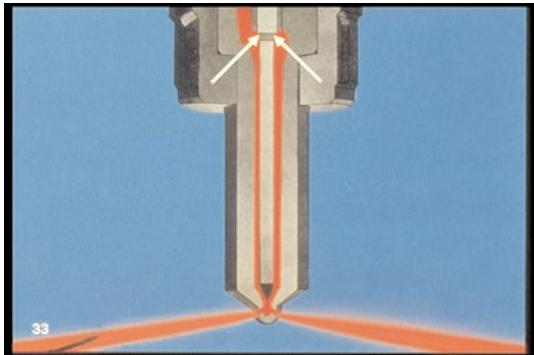
33. When high-pressure from the pump is applied here, the needle-valve lifts to deliver fuel in the broad angle of hole-type nozzles.
