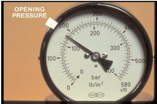
25. . . . that's your opening pressure — in this example (on the inner scale) 125 bar. This one is within checking tolerance from 120 to 130. What if opening pressure were not in spec?
