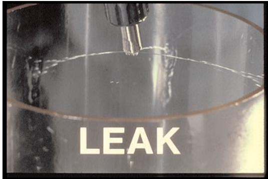
65. A leak at the needle seat could deliver fuel in a pattern like this.
