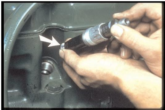
49. On some nozzles, you'll need a new washer to be sure it will seal the nozzle, as well as position and cool the injector in the head.
