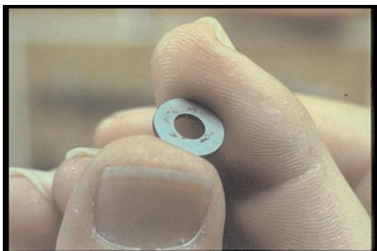
66. The adjusting shim must be smooth and not worn or corroded. Otherwise, replace it.
