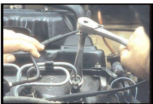
22. That means you'll have to disconnect all the fittings (notice the special wrench). But don't bend the high-pressure lines because inside particles could flake off and get into the injectors.
