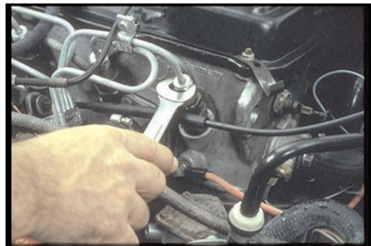
15. . . . loosen one high-pressure fuel line fitting, a little like this—
