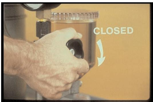
20. Close the valve to protect the gage mechanism. Close it whenever you're going to stroke rapidly.
