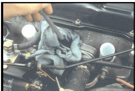
28. Before you leave the engine, stuff a rag in the openings to keep dirt out of the cylinders.
