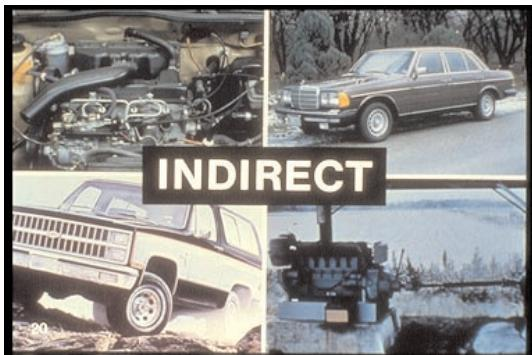
20. You'll find pintle-type nozzles and indirect injection in most passenger car engines, as well as some light truck, industrial, and small marine engines. Indirect injection is usually smoother and quieter than direct injection.
