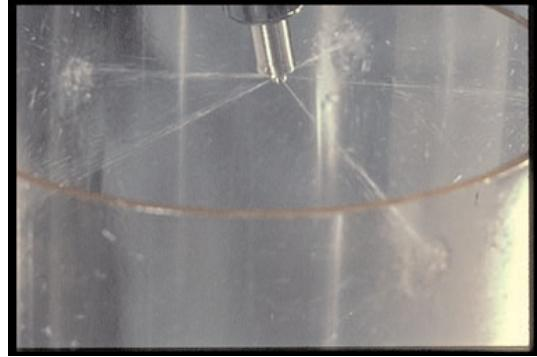
61. But, at this slow pumping rate, the spray pattern is not good – it is divided, with coarse atomization.
