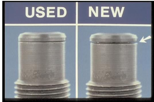
69. You've learned the importance of replacing a separate used heat-shield or washer with a new one to insure a good seal and good heat-transfer.
