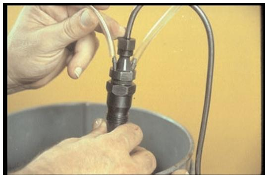
38. For some nozzles, you'll need to slip on clear plastic lines like this to hold extra leak-off fuel. Otherwise fuel runs down the side and fools you into thinking this nozzle won't pass its leak test.
