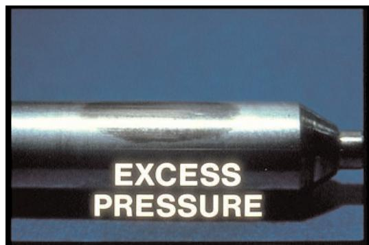
54. Some technician's improper handling — incorrect gaskets or excessive torque — caused excess pressure on the nozzle body distorted the body, causing pressure marks, and leading to nozzle failure.
