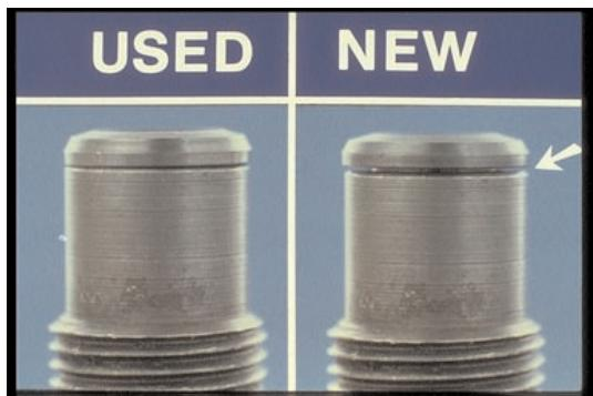
46. Never put in a used heat shield. Remember only a new heat shield can be properly crushed to insure good seal and good heat transfer from the nozzle tip to the cylinder-head. And be sure you install it the right way.
