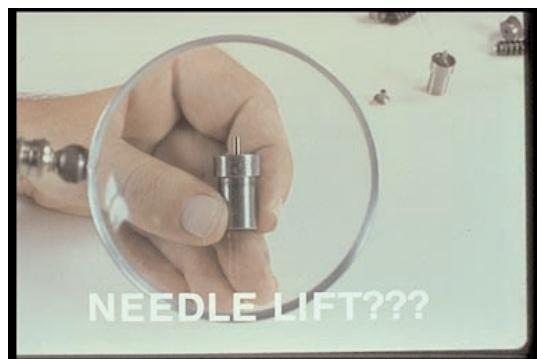
15. Without such equipment, excess needle lift might cause increased flow-rate and you wouldn't know it.
