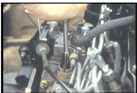
59. . . . reconnect the electric fuel shut-off or turn on the fuel and crank the engine to bleed the lines.
