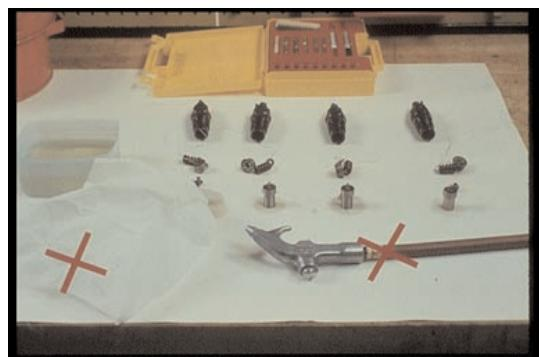
71. . . . with towels and compressed air. But no! This could leave dust particles on the pressure faces of the valve body and the nozzle holder.
