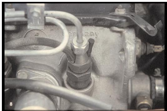
8. Each line leads from the pump to an injector mounted in the cylinder head.
