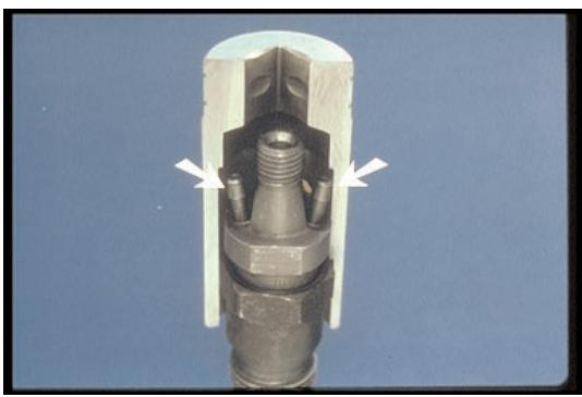
24. On this widely-used nozzle holder, the proper socket will clear the return line fittings like this. If the socket is not properly relieved, it will probably break them off.
