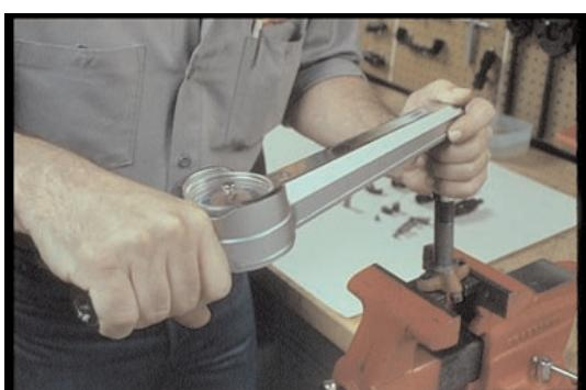
76. In the vise, tighten the nut the final part of a turn, according to the torque values in your specs.
