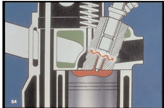
54. In other type nozzle holders, heat from combustion is carried away like this through heat shields and gaskets to the cylinder head. You can see why good contacts of gaskets, or heat shields, are important to the job of the nozzle holder -- cooling the nozzle.
