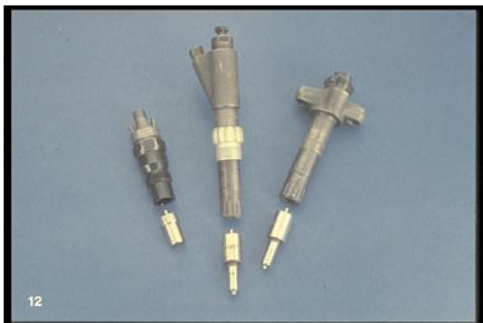
12. Whatever the type nozzle, whatever the type of nozzle-holder, every injector must operate reliably and with great accuracy within the heat and combustion gases of the engine.
