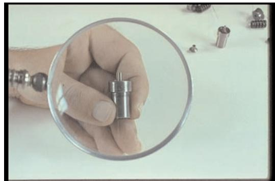
46. The nozzle body should also be inspected for signs of damage. This body is OK.
