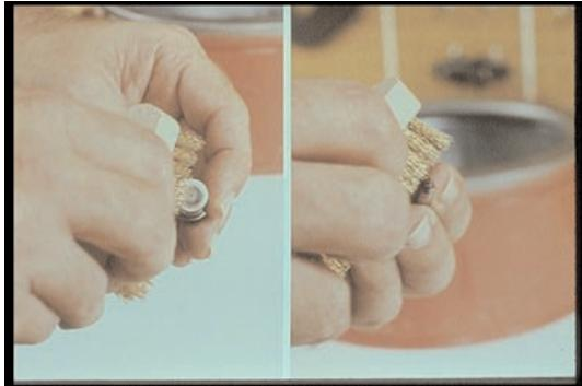
33. With the brass brush, remove any carbon from the outside of the nozzle body and needle tip, especially the needle seat. Never use emery paper or any abrasive to clean the nozzle.
