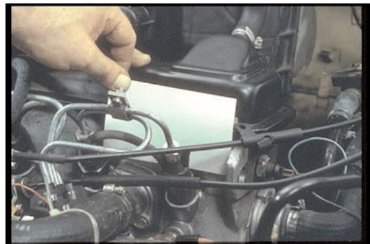
62. Then, with a card like this near each fitting in turn, you can check all lines for leaks. If you remember the kind of high-pressure in those lines, you won't feel for leaks with your hands as you complete injector servicing on the engine.
