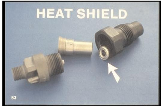
53. . . . with this holder, also KC, used on Chevrolet six-point-two liter engines; the heat shield goes inside the capnut -- on the right.
