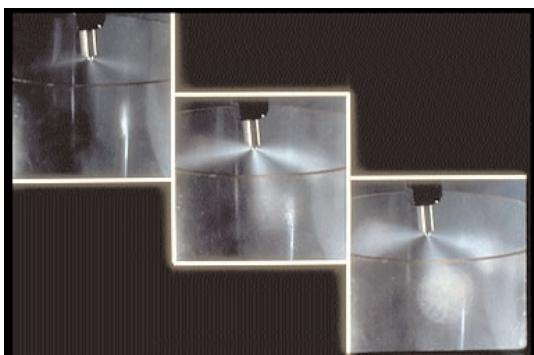
76. When you fast-pump a good hole-type nozzle, you expect to see a good spray pattern like this, and hear a good chatter, like this. You know the difference between a good hole-type spray pattern,
