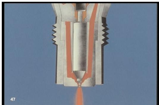
47. When pressurized fuel lifts the needle, fuel is delivered. Delivery continues until pressure drops.
