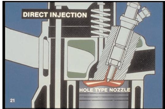
21. In this direct-injected engine, notice the wide spray-angle patterns of the hole-type nozzle required to distribute fuel directly into the cylinder.
