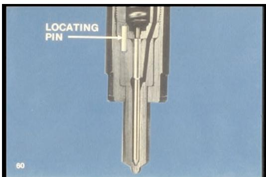
60. . . . the nozzle is positioned by locating pins in the intermediate plate. When servicing injectors, you'll want to take good care of these locating pins.
