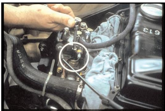
43. First, shut off the fuel (in this engine by disconnecting the electric fuel shut-off).
