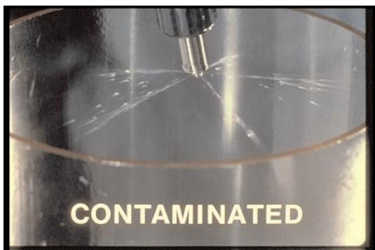
67. Contaminated fuel can clog the delivery holes of this hole-type nozzle, causing this kind of pattern.
