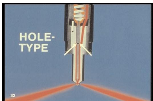
32. . . . to the operation of the hole-type nozzle. High-pressure applies lifting force here -- on this part of the valve.
