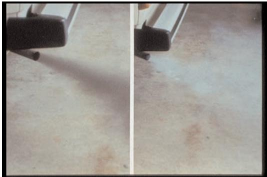
9. Smoke—black smoke which could also come from overfueling; white smoke which could also come from incomplete combustion, or water in the combustion chamber.
