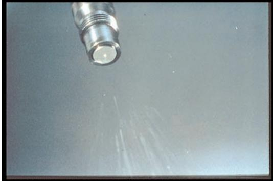
73. You've got the message — at slow tester pumping, you might see a poor spray pattern like this, but that doesn't mean a bad injector. You might hear a good, soft chatter like this. And that doesn't mean a good injector.
