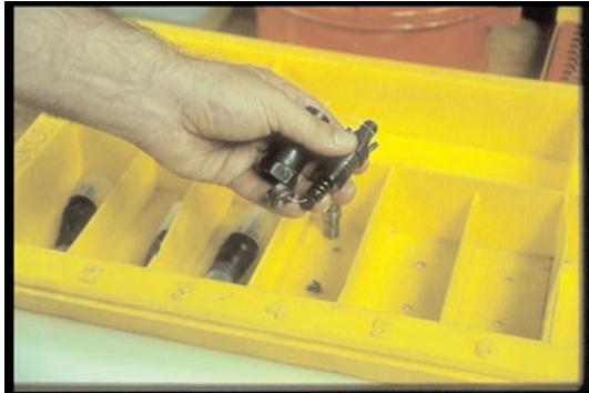
25. In your parts tray, keep parts from each unit together; wiring spring and shims like this helps a lot.
