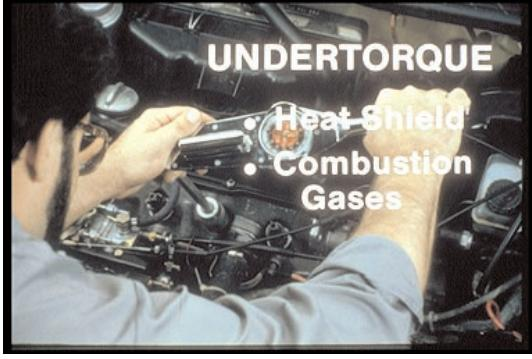
54. If you undertorque, you will fail to seat the heat shield; combustion gases may leak and burn the nozzle tip.
