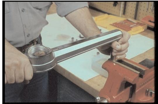
77. Of course, many pintle type nozzles can be tightened and torqued right in the vise. In this program, you've learned to recondition injectors, precision parts,
