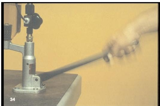
34. When you pressure-test a nozzle on the nozzle-tester, you should hear a chatter sound, depending on how fast you're stroking the tester handle.
