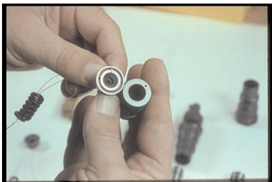
60. These lapped surfaces seal high-pressure fuel; they must be flawless in fit.
