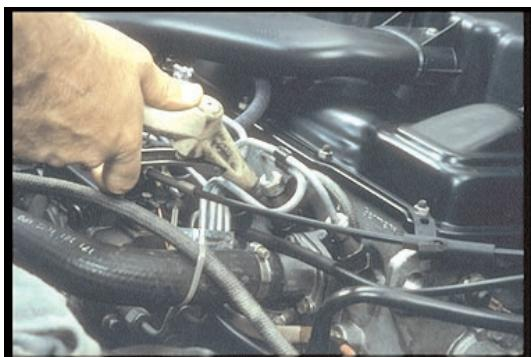
20. Be sure to clean around the nozzle-holder assembly; you don't want dirt to fall into the engine when you remove the injector. After removing the return lines,
