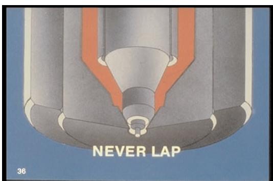
36. You can see that the needle seats precisely in the nozzle body. Never lap a nozzle needle or seat; you could change an OK nozzle into a drip!
