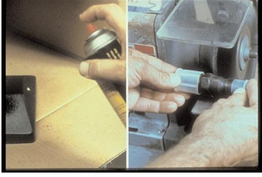
7. . . . no spray-painting and no grinding. Your best clean rooms have an air-filtering system and are separate from dust-making service operations.
