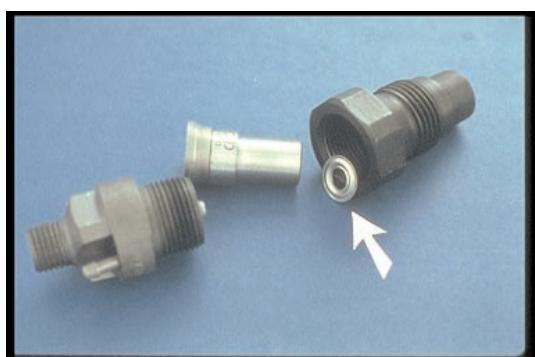
48. In some injectors like this, the heat-shield is inside the injector so don't add another heat-shield in the recess.
