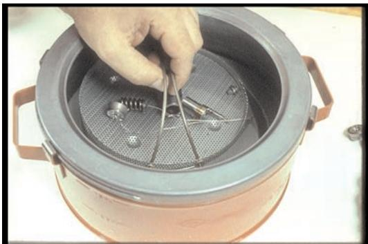
32. To clean burnt-on combustion deposits, use a commercially-available parts solvent.
