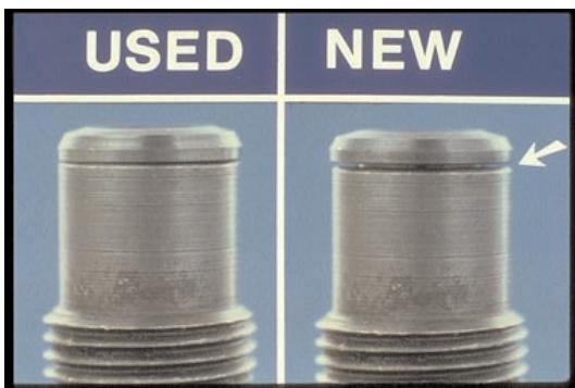
27. A separate used heat shield should be thrown away. When you torque a new one in place, it will crush this space properly to provide good heat-transfer and to seal the pressures.
