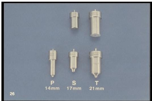
26. In pintle types and in hole types, you'll find nozzle sizes to match different fuel delivery requirements. As you have seen, different letters indicate the size of the nozzle, generally bigger nozzles for bigger engines.
