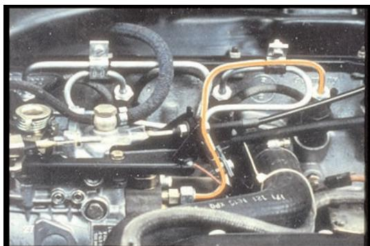
27. Now, take a look at how nozzles operate. Start with fuel at less than injection pressure. We've shown that in orange in one line, from pump to injector. When the pump plunger strokes,
