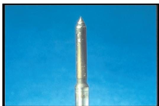
56. These combustion residues collected because the nozzle-spring pressure was less than combustion pressures. Adjust opening-pressure so the cylinder gas can't blow back inside the nozzle.
