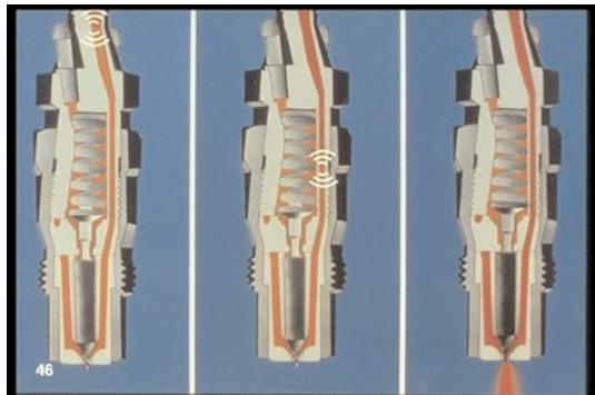
46. Another job is to deliver the fuel. In a fraction of a millisecond, high-pressure from the pump reaches the tip and overcomes the spring-force to lift the needle.
