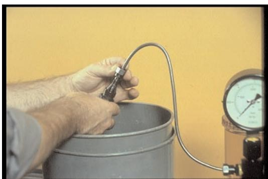
19. When your tester is ready, connect your first injector to be tested and snug it down.
