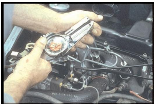
60. Now, torque all fittings, injectors and pump. Don't forget to replace the leakoff lines.
