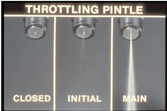
17. Good atomizing can depend on the rate of injection. As the throttling pintle is lifted from closed, the pintle shapes the initial spray for easy injection. Further lift delivers the main-spray -- wider, more finely atomized for complete burning. Good atomizing means a smoother-running engine with reduced emissions and smoke.
