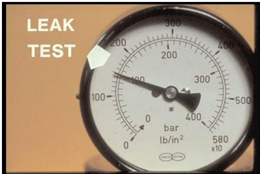
33. For your leak test, in this example, you want to build and hold to 20 bar less than opening pressure, or as specified.
