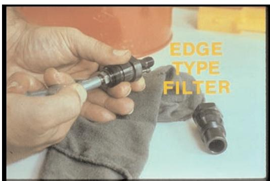
42. Use compressed air to clean the edge-type filters, blowing from the nozzle side of the holder; the filter is not removable.
