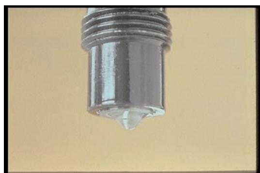
72. You know one drop can form. If it does not fall off in 10 seconds, the nozzle tests OK.
