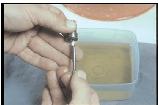
36. Use the scraper dipped in test oil to clean the seat.
