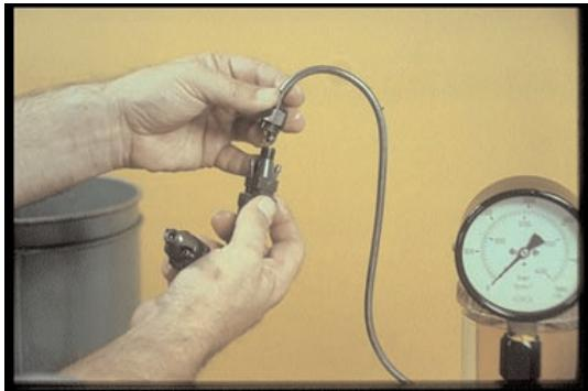
41. Check your specs: some nozzles chatter only softly, depending on how fast you pump the handle. In general, spray patterns should be judged only when pumping the tester handle fast, fast, fast.
