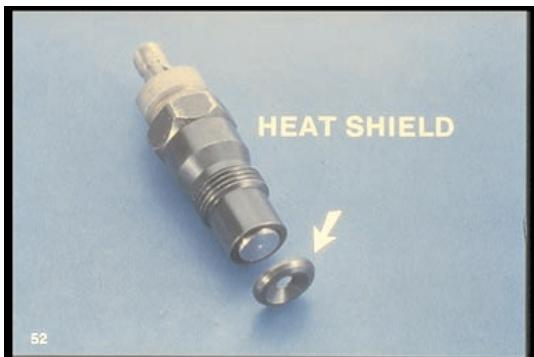
52. In this KC-type nozzle holder, a properly-torqued heat-shield provides heat transfer from the nozzle to the cylinder head; it also applies pressure from the cylinder head to the holder instead of to the nozzle. Contrast this location of the heat shield.
