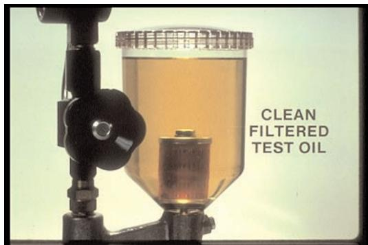
16. Your test oil should be clean filter test oil, or as called for in your specs.
