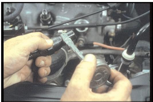
50. Use an anti-seize type compound to make the next removal easier—a long way down the road. When you start threading by hand you can be sure you're not cross-threading.
