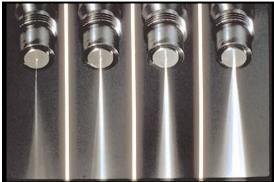
49. When you pump fast, you should see a good pattern, here slowed by high-speed photography. You have a good nozzle. But you must check your manuals to know what pumping rates should produce what kind of chatter. To judge spray-pattern, be ready to pump fast. Fast pumping is the way to test patterns.
