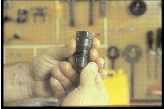
63. Inspect the nozzle nut for physical damage; check for coking inside the surface or damaged seating surface.
