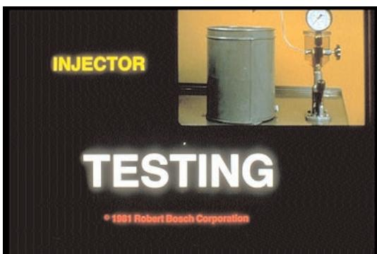
3. Injector testing — for opening pressure, leakage, chatter and spray pattern — that's what you'll be able to do when you finish this program,
