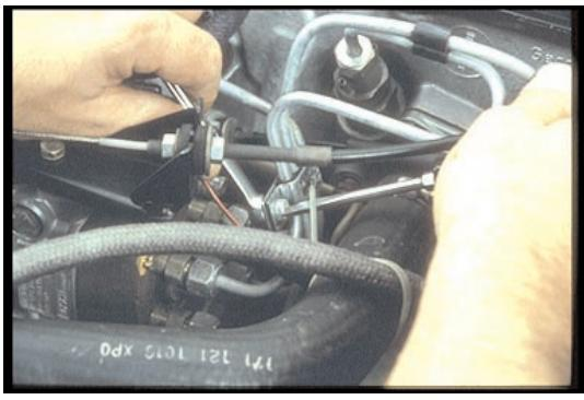
21. . . . loosen the clamps before you disconnect the high-pressure lines, even if you are pulling only some of the injectors.
