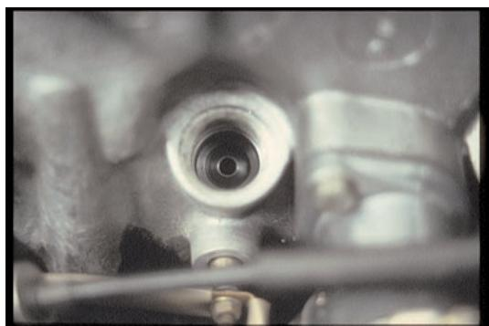
47. This kind of heat shield looks like this when it's properly installed, the flat outer-rim facing you. When you install the injector, be careful not to strike the nozzle tip or the pintle.
