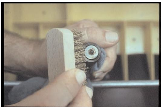
34. Using a brass brush, clean the carbon from the nozzle tip. And be careful of the pintle needle.
