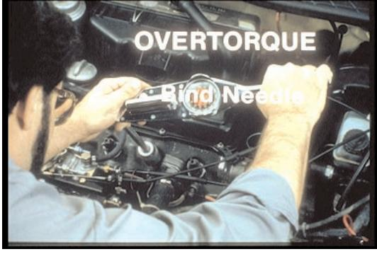
53. With most injectors, if you overtorque the injector, you may cause needle binding.
