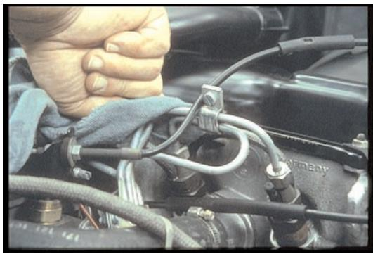
19. . . . clean up before you start. You don't want to let any dirt into the injector or into the pump.
