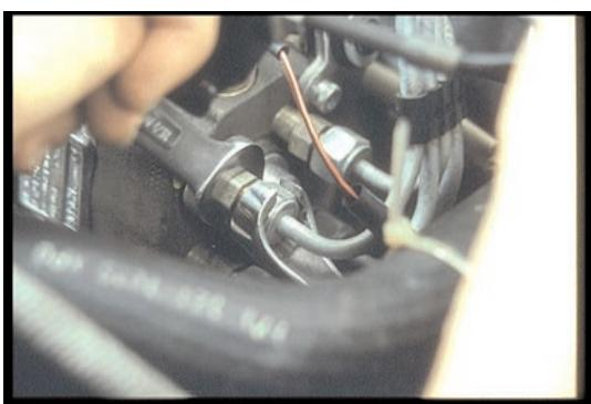
23. At the pump, hold the delivery-valve holder while you loosen the line fitting. Once removed, the lines should be capped to keep the insides clean.
