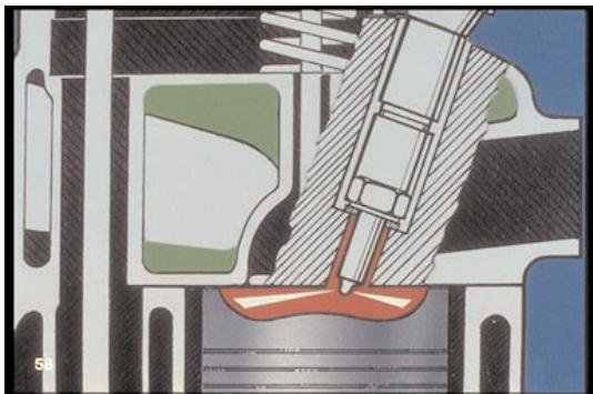
58. In contrast, with direct injection, the KB and KD holders are usually positioned at an angle to the combustion chamber and the piston. If the nozzle is not vertical, the spray holes must be angled to match the piston crown.
