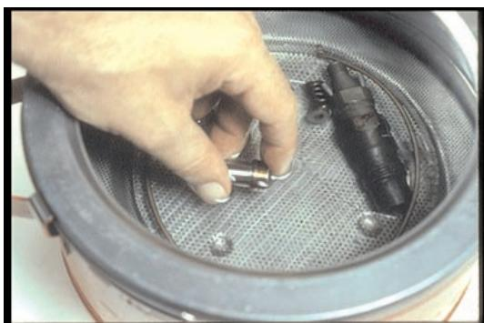
35. When you've finished scraping, rinse in clean solvent to remove the dirt and carbon you've loosened.
