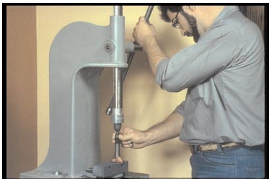
74. Remember hole-type and some pintle injectors need force down against the pressure-spring,
