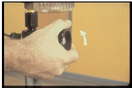
23. To measure the pressure, you'll need to open the gage valve — open it just slightly.
