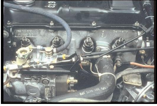
55. With all injectors properly torqued in place, you're ready to reinstall the lines.
