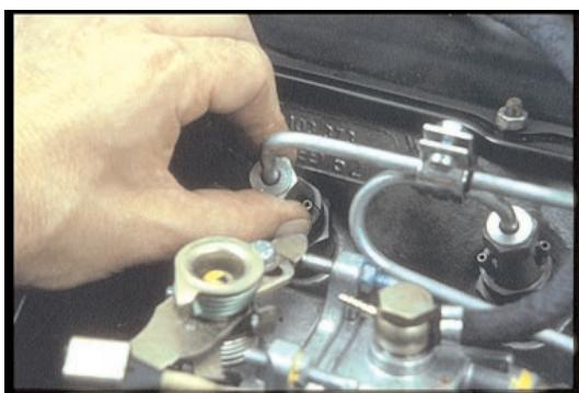
58. That way, you'll find it easier to thread the fittings onto the injectors. But before you tighten the injector fittings,
