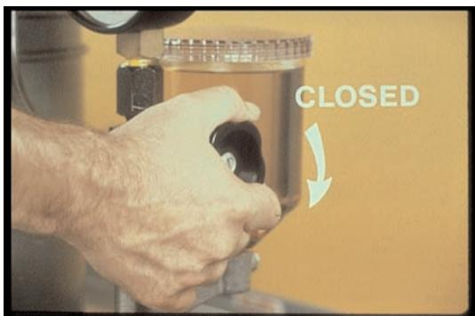
42. You want the valve closed because later, you're going to pump fast enough to damage the gage.
