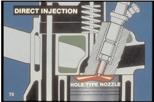
73. . . a hole-type nozzle with its wider spray-pattern -- direct-injection into the cylinder.
