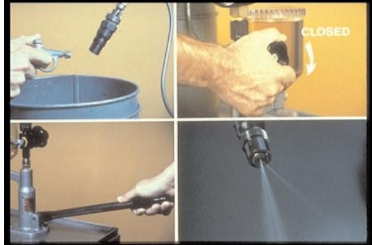
37. See if you can clear it out; dry the tip, close the gage; a few fast strokes may clear it. But if you still see the spray pattern of a contaminated needle, or if fails the leak test, don't try to lap it; replace it.
