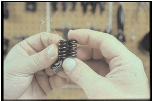
65. Compare spring length to a new spring. If in doubt, replace it. Also, if the spring is pitted or shows excessive wear, replace it.
