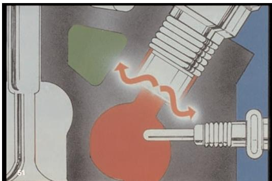
51. Cooling the nozzle is an important job of the holder. Nozzle-tips are exposed to the heat and pressure of combustion -- heat which is carried away to the cooling system by the holder.
