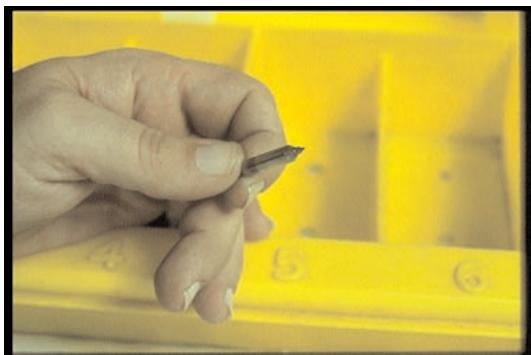
26. Of course, you hold the needle valve by the stem unless you have wet your fingers in test oil to protect the lapped surfaces from skin acid. Is that really a problem?
