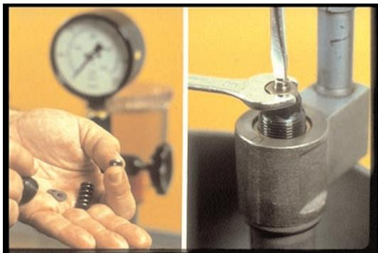
26. Some injectors need disassembly — in the best clean-room facilities — to change the shims; in others, you turn the adjusting screw without disassembly.
