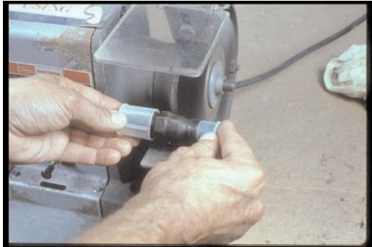
33. In the shop, you can clean the outside if you're going to test injectors or inspect the outside.
