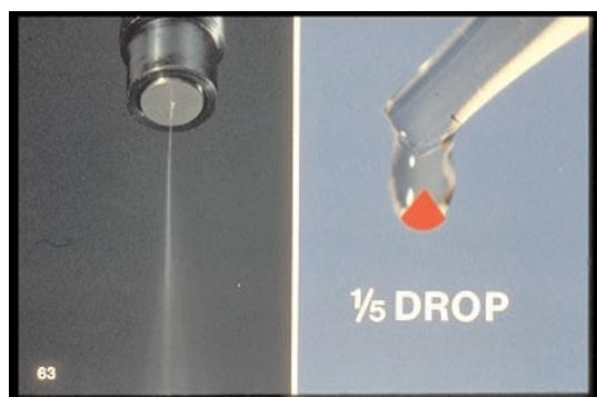
63. Precision delivery. In some idling engines, one stroke of an injector must deliver only one-fifth of a drop of fuel, no more, no less!
