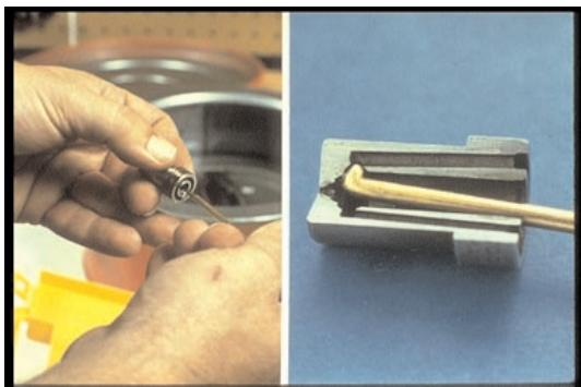
34. When you clean the ring groove, the scraper loosens the dirt like this.
