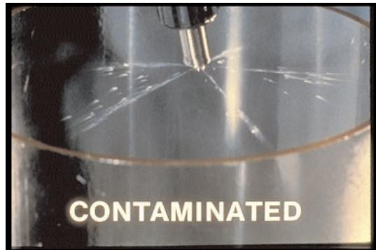
77. . . . and a poor pattern, such as from a contaminated nozzle, like this. Judge a nozzle as bad by its pattern, not by its sound.
