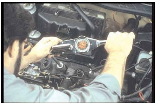
51. Screw in and torque the injector according to specifications.
