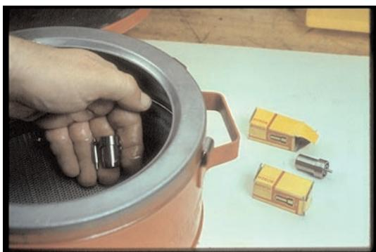
43. New replacement parts need cleaning too. Solvent removes the protective coating. And new or re-used, when the parts are completely clean,
