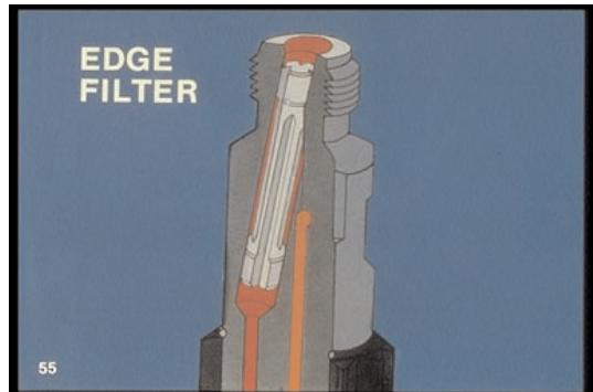
55. Some holders do another job; they contain an edge filter for incoming fuel. The filter is not removable so it must be cleaned as part of the holder.
