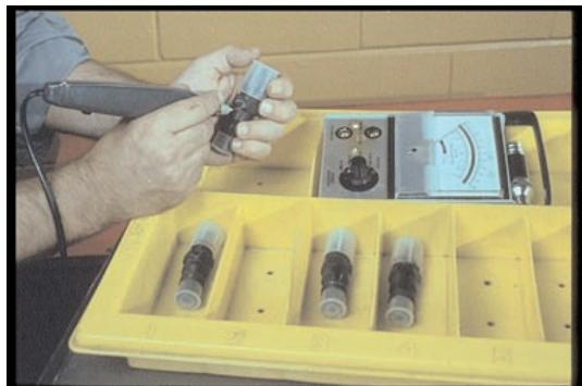
30. Numbering injectors now may help you find an engine problem later, such as a bad valve in one cylinder which shows up on that injector. Stop now for review of injector removal.
