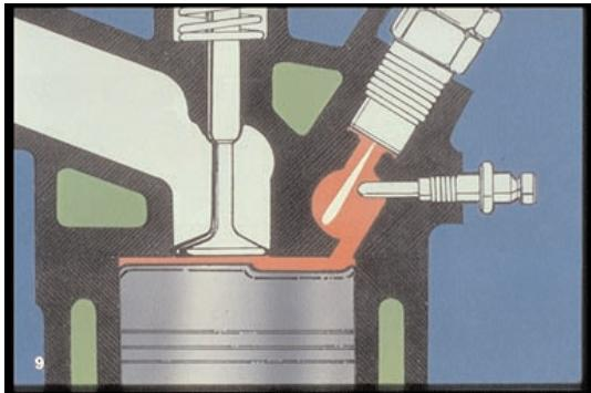
9. The injector sprays high-pressure fuel into the combustion chamber; it must provide accurate delivery, and good atomization.
