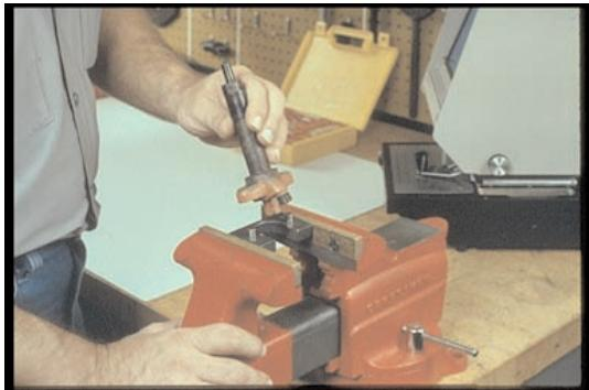
18. Disassembly procedure includes knowing injectors and how they're put together; otherwise, in your first step, you could ruin one.
