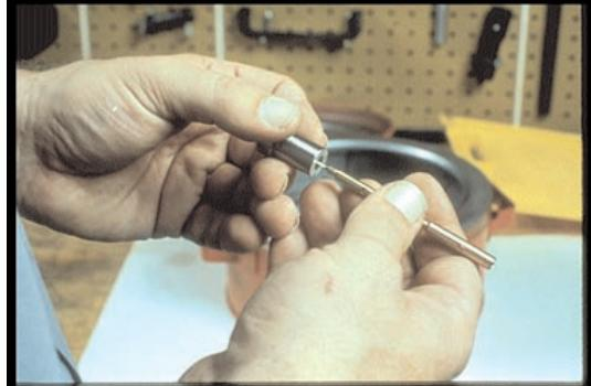
38. Same thing for these orifices in the hole-type nozzles. Be sure the wire is just small enough to fit in the hole without forcing. Never use a ream; you might enlarge the hole and ruin the nozzle.
