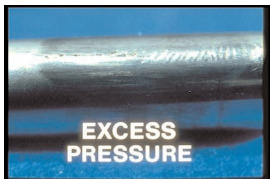
55. Another improper handling — score marks from scuffing in a deformed nozzle body as a result of excess torqueing pressure on the nozzle.
