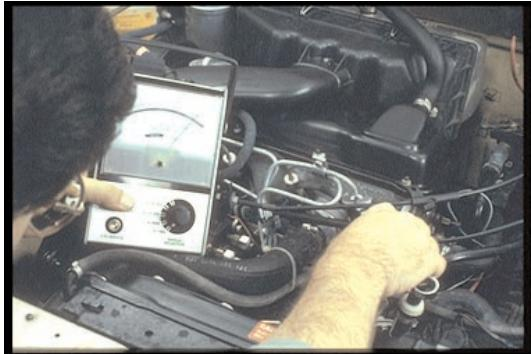
17. If you're not sure, use a diesel tachometer. As you loosen one fitting, check the RPM drop. This one's OK. If you get the same RPM drop on all of them, it's likely the problem is in the engine. With some exceptions, removing a good injector can do more harm than good. Stop now for review of troubleshooting.
