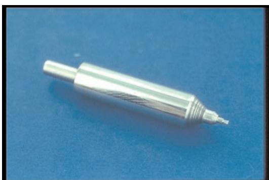
28. . . . in a few hours, you'd have a ruined needle! You'd have to throw it away, along with its mated nozzle body — just because of a careless fingerprint!
