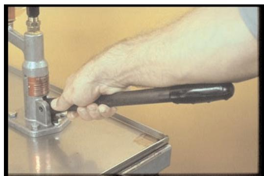
24. Now, slowly apply pressure; using your arm like this, you can control it better. If necessary, pump to maintain the pressure. When the spray starts,
