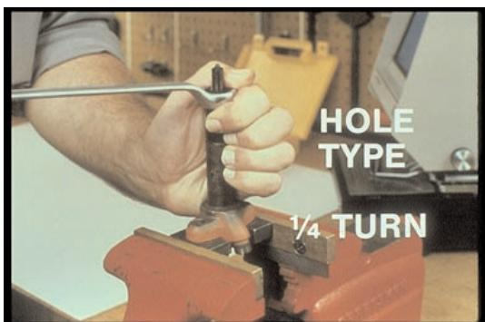
19. For most injector types, using a fixture in your vise, hold the injector upside down, like this.
