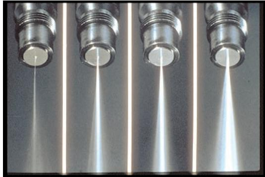
5. You've seen how the nozzle delivers the metered fuel, atomizes and distributes it for power, economy and emission-control.
