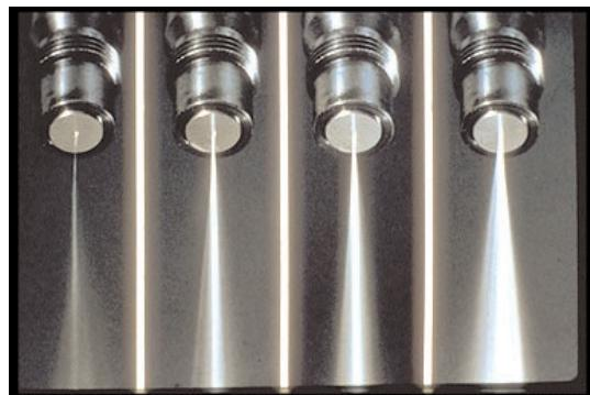
6. . . . to open the nozzle and deliver fuel, as in the engine. The action is slowed by high-speed photography. You should know that these high pressures can be dangerous.
