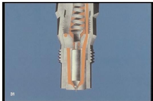
31. . . . pressure drops at the injector so the needle can snap shut, seating the valve with a sharp cut-off -- no drip, no dribble. That's how a pintle nozzle operates. Compare that,
