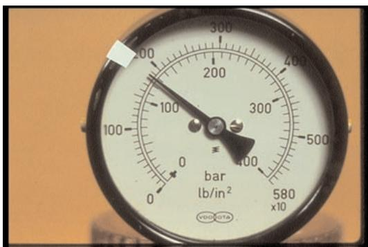
27. Whenever you set opening pressure, set it toward the high-end so it will stay in tolerance after the injector seats in. Stop now for review of the opening pressure test.
