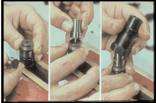
73. After the intermediate plate, and the nozzle, thread the nozzle nut several turns, but if it's a hole-type injector, do not snug it up yet.
