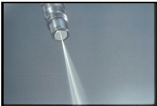
10. In your blood stream, this can cause blood poisoning. Keep your hands out of any spray — and always wear glasses for eye-safety. High-pressure test oil can seriously damage your eyes.
