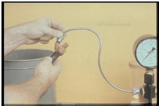
59. Install the nozzle; snug it tight and be sure to close the gage. Testing hole-type nozzles for opening pressure and leak-testing is the same as for pintle nozzles
