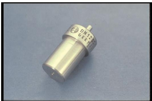
43. You can check the spray angle from the code on the nozzle. On this nozzle, the first numbers after DN – 12 degrees.
