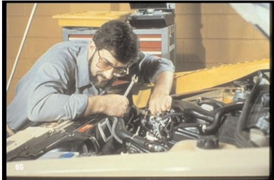
65. Don't break into the fuel system until you've done proper engine diagnosis. Be sure you have good reason to remove injectors from the engine.
