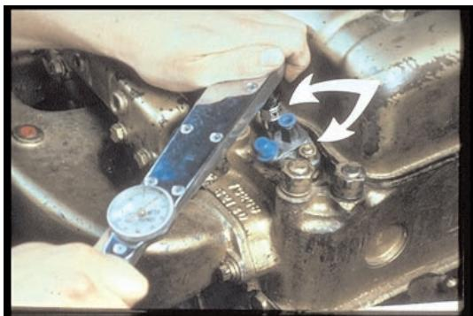
52. With these KB nozzle holders, be sure to alternate from one hold-down nut to the other to prevent cocking the injector; that could cause jamming of the nozzle.
