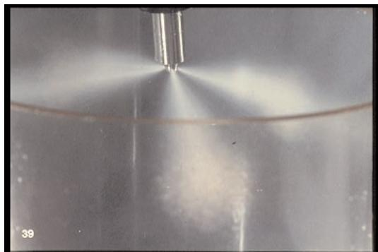
39. In a hole-type nozzle, a good spray pattern like this is determined by the holes. When you clean the holes, you must never change the size or the angle; you must never round the edges of the holes. Compare the fine atomization and distribution from nozzles properly handled,
