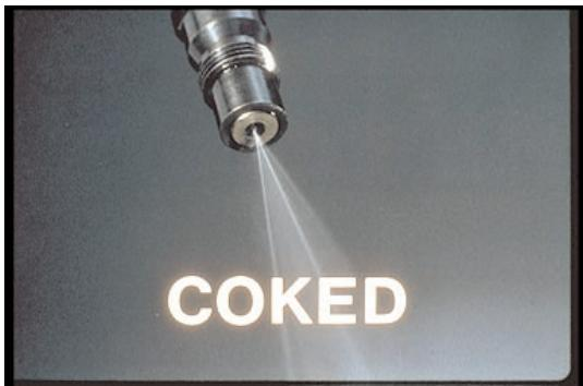
51. You might see this pattern from the coking of the needle as a result of combustion gases being forced inside the nozzle body. Judge such a nozzle by the pattern, not by the sound.
