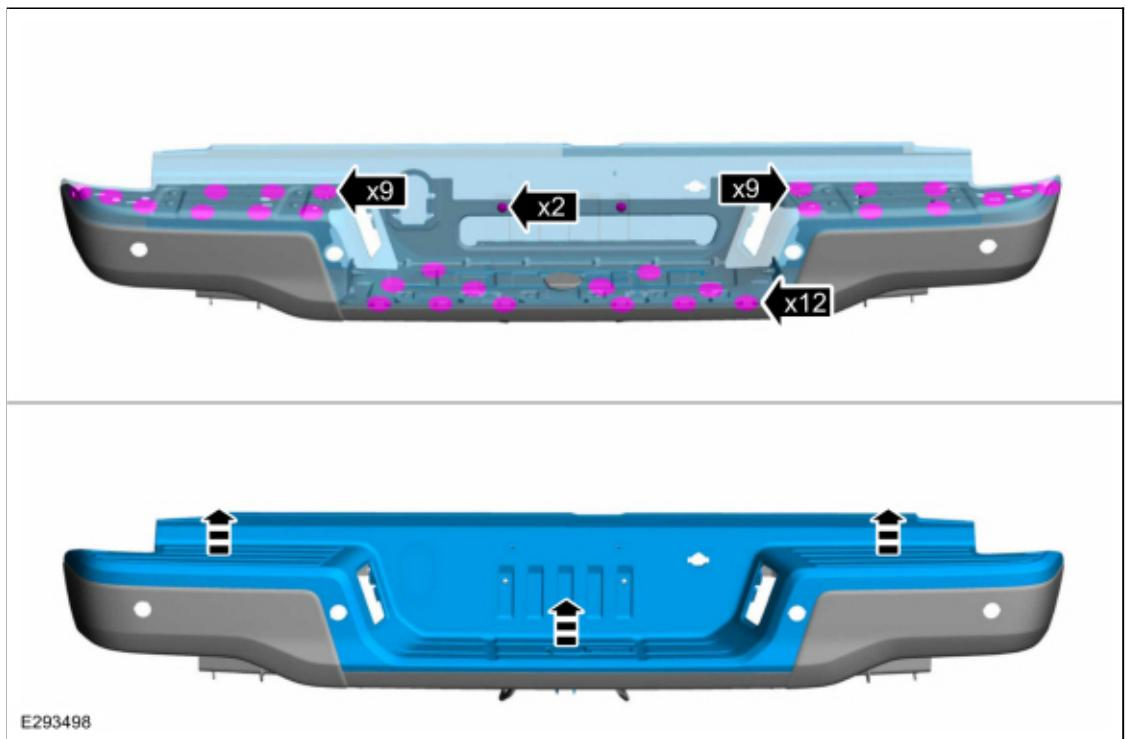
9. Remove the trim pins, the bolts and the rear bumper lower cover.
