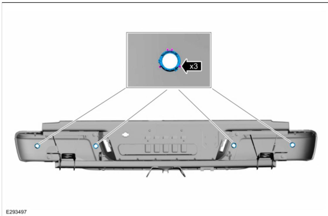
8. Remove the trim pins, release the tabs and remove the rear bumper step plate.
