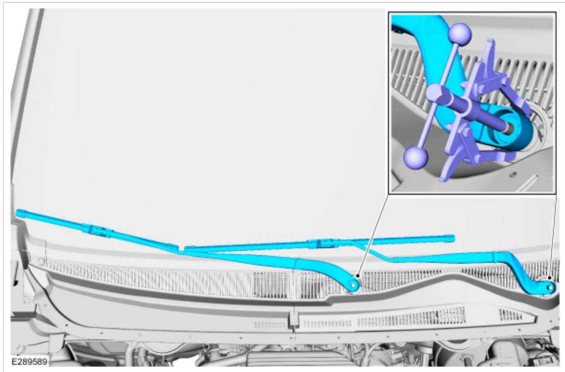
4. **NOTICE: Make sure that the component aligns with the installation mark.**
