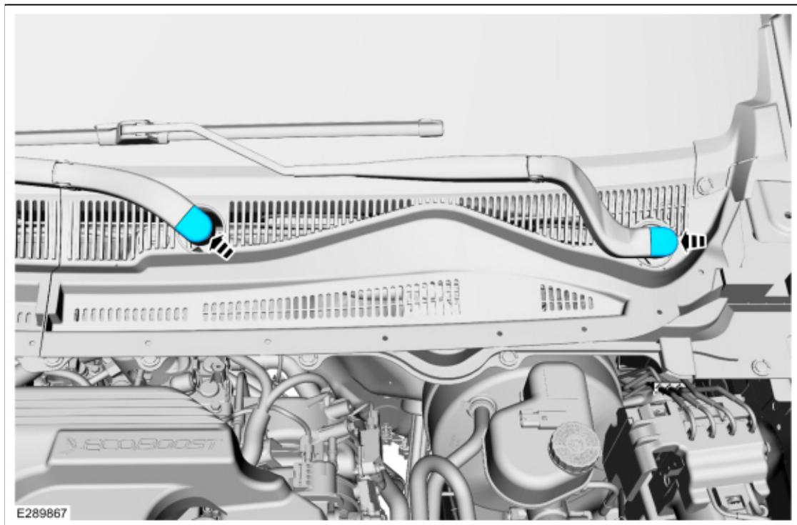
7. If necessary, adjust the wiper blade and pivot arm.
