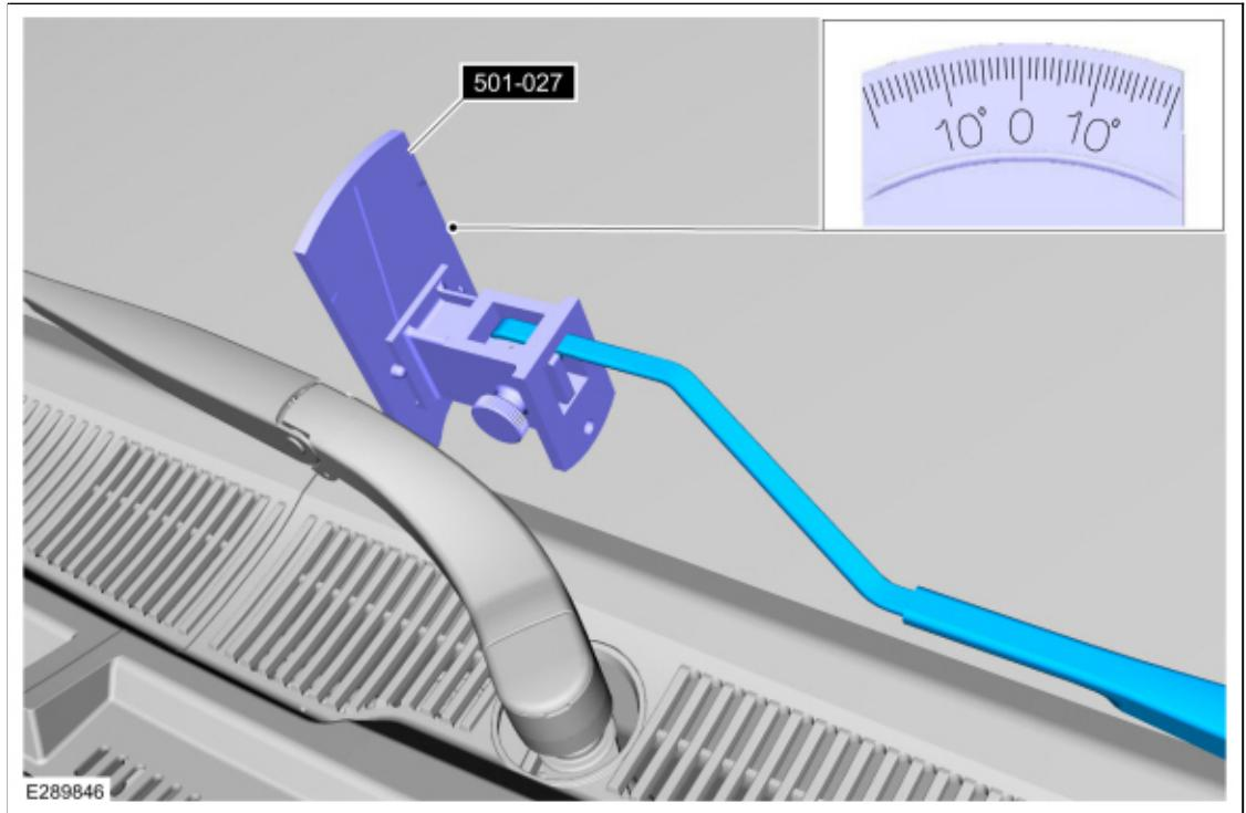
4. **NOTICE: Make sure that the special tool is lifted off the glass while adjusting the angle.**
