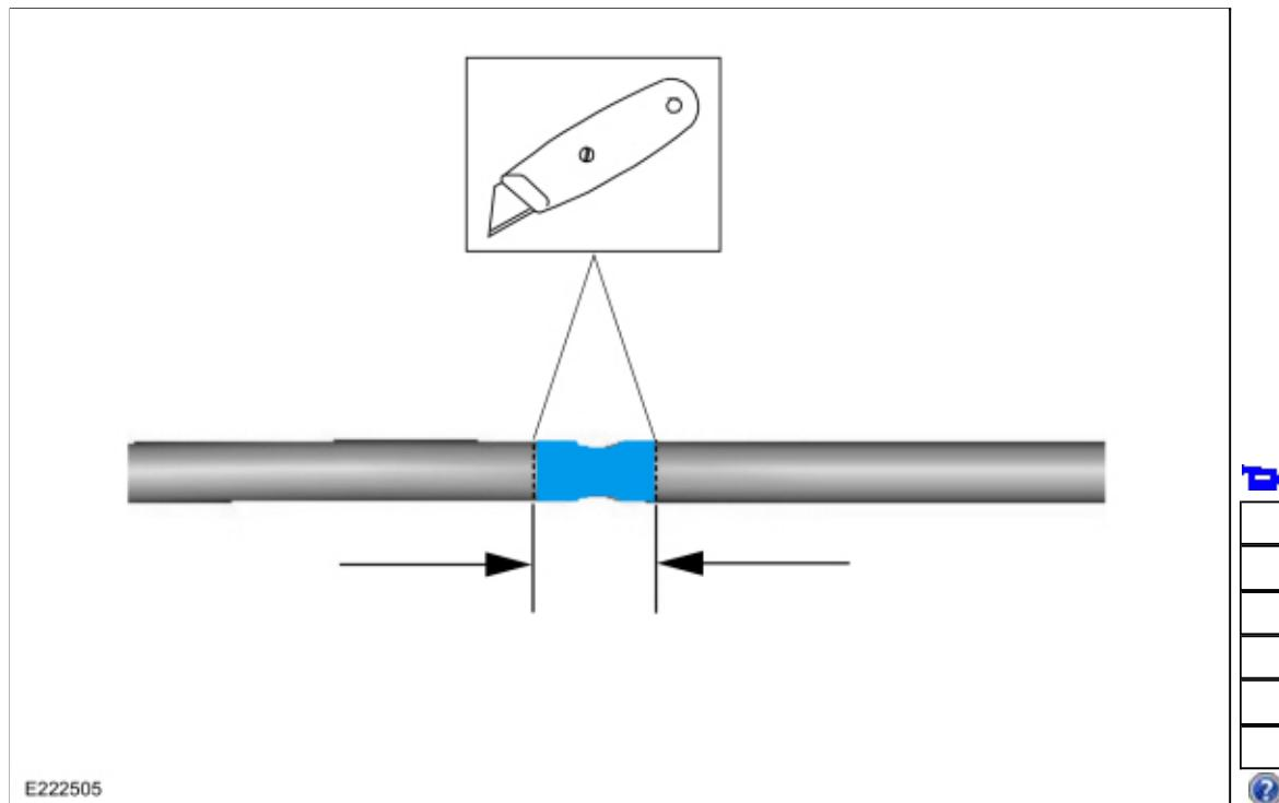
3. Install a windshield washer hose adapter between the cut ends of the hose.
