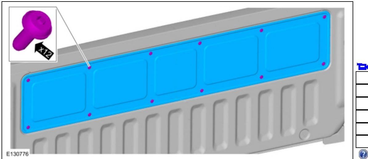
2. Remove the bolts from the tailgate control assembly and position aside.
