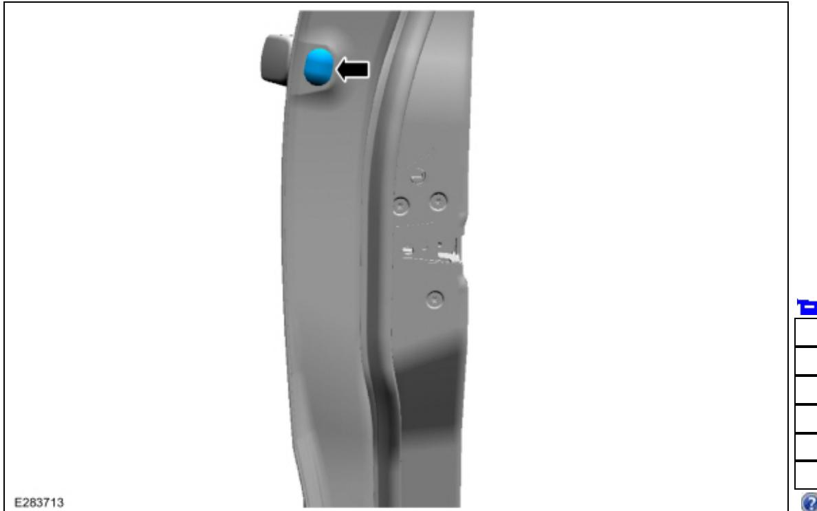
2. Remove the door lock cylinder.
