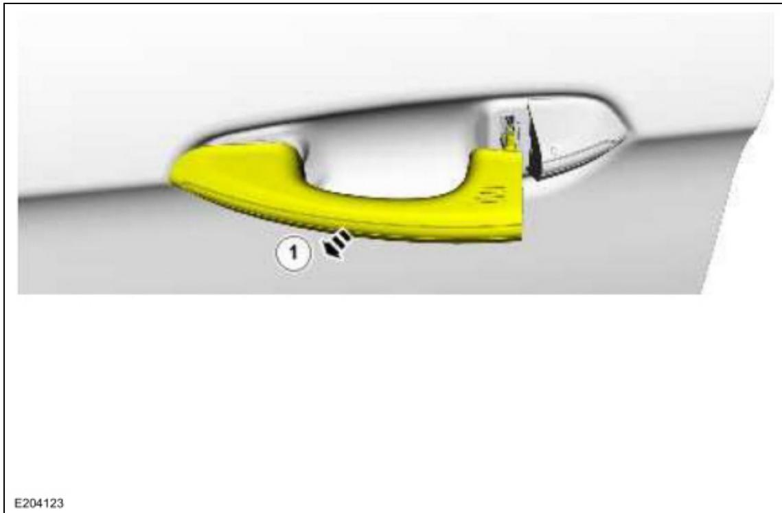
5. Open and close the door several times to circulate the lubricant inside the latch.
