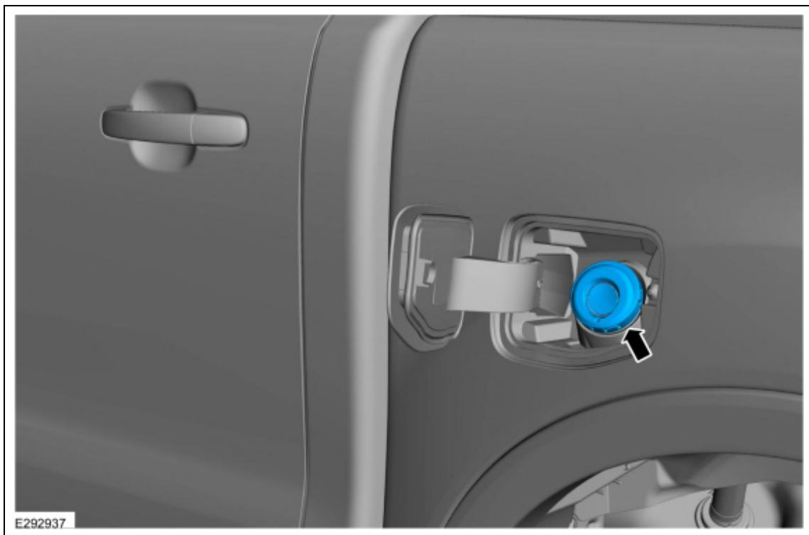
3. Using a knife, slice through the heat stakes holding the fuel filler molding to the outer sheet metal panel.
