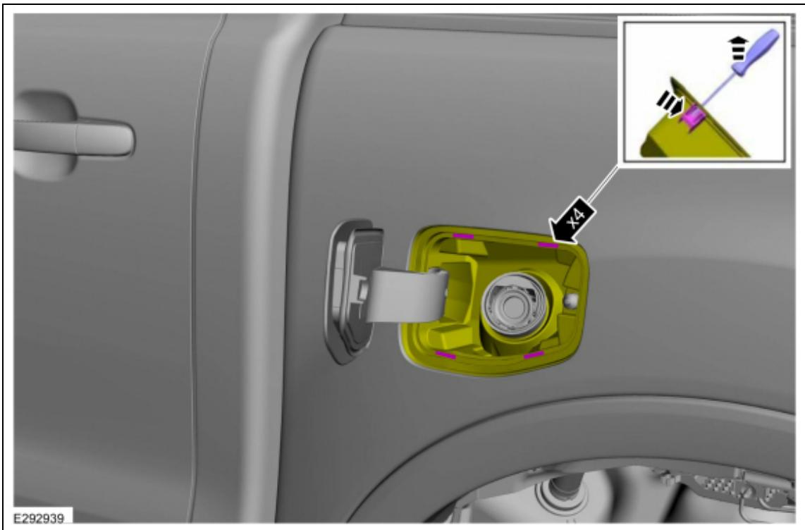
5. Pull the fuel filler door assembly away from the vehicle and remove.
