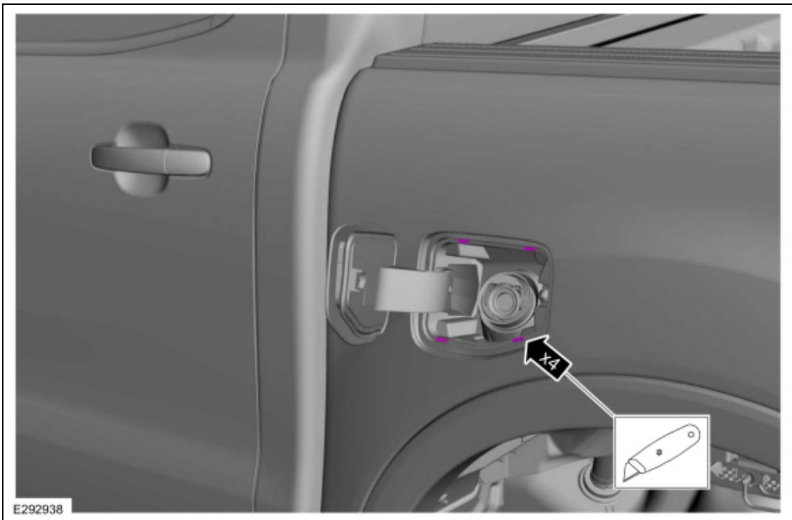
4. Insert the screwdriver and release the clips while pulling the fuel filler door housing away from the vehicle.
