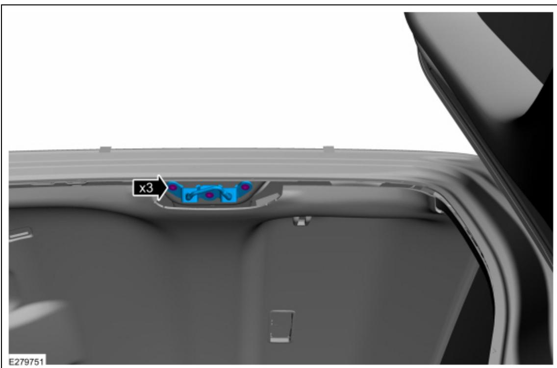
16. Install the upper striker assembly trim panel cover, position the weatherstrip.
