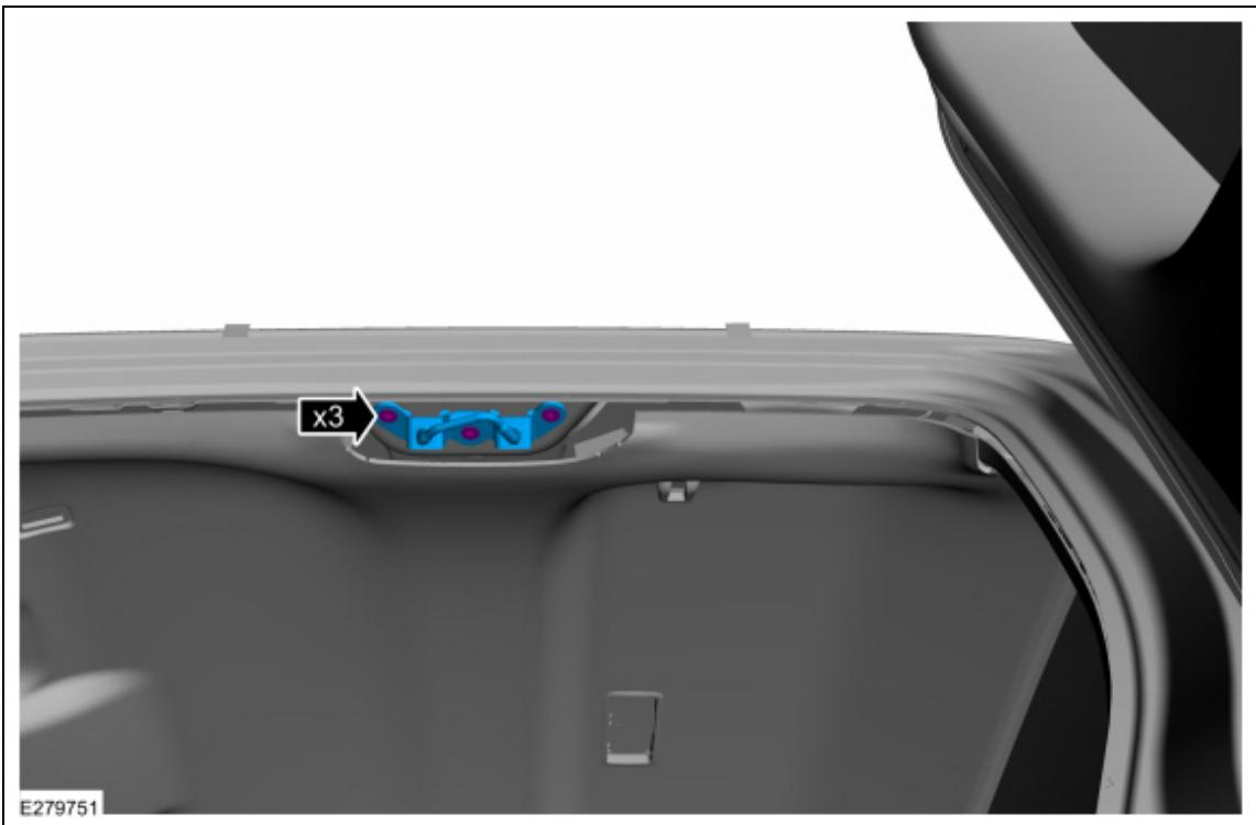
5. Remove the bolts and the lower striker assembly.
