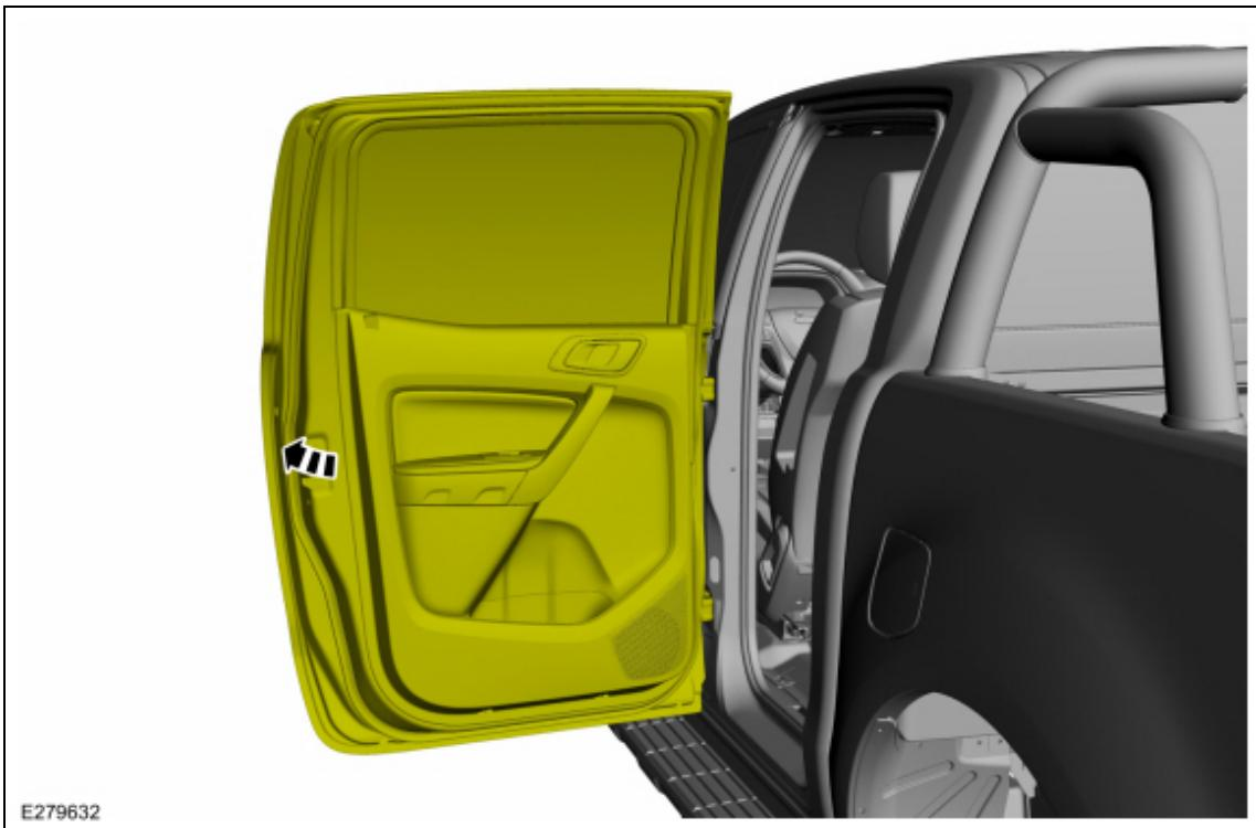
12. Loosen the nuts enough to permit movement of the door.
