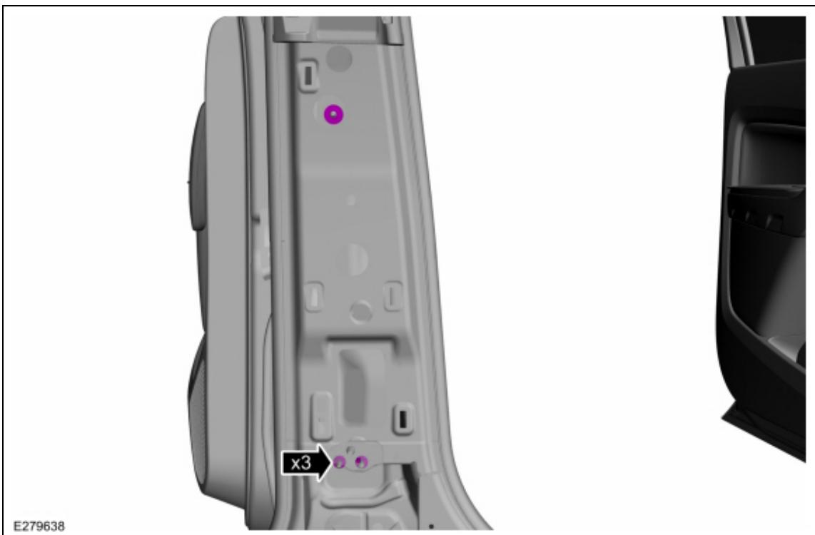
20. **NOTE:** During installation, make sure the safety belt webbing is not twisted and the safety belts and buckles are accessible to the occupants.
