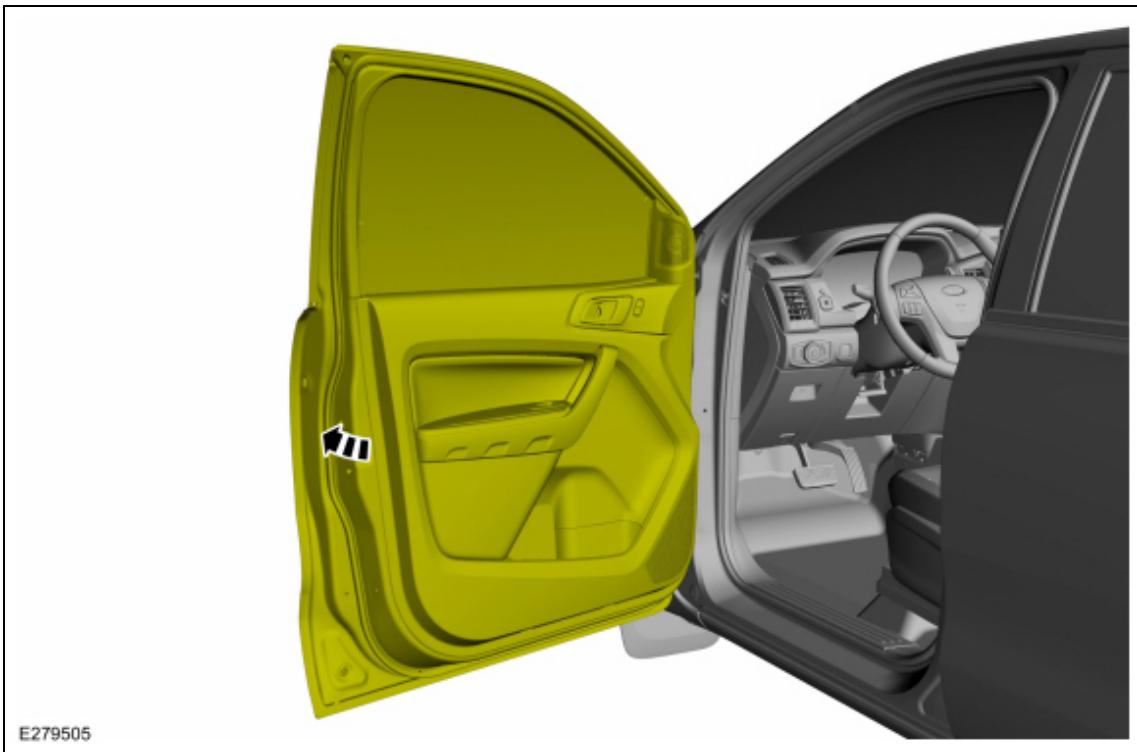
10. Loosen the bolt enough to permit movement of the door.
