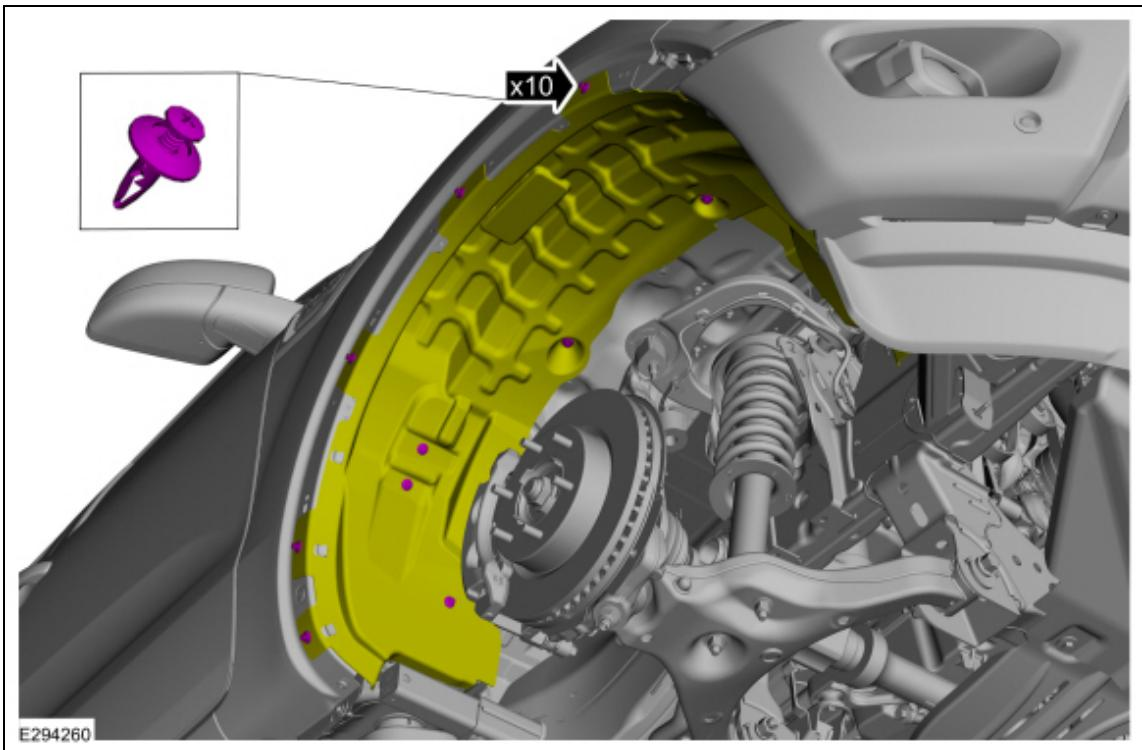
5. Remove the pin-type retainers and the fender splash shield.
