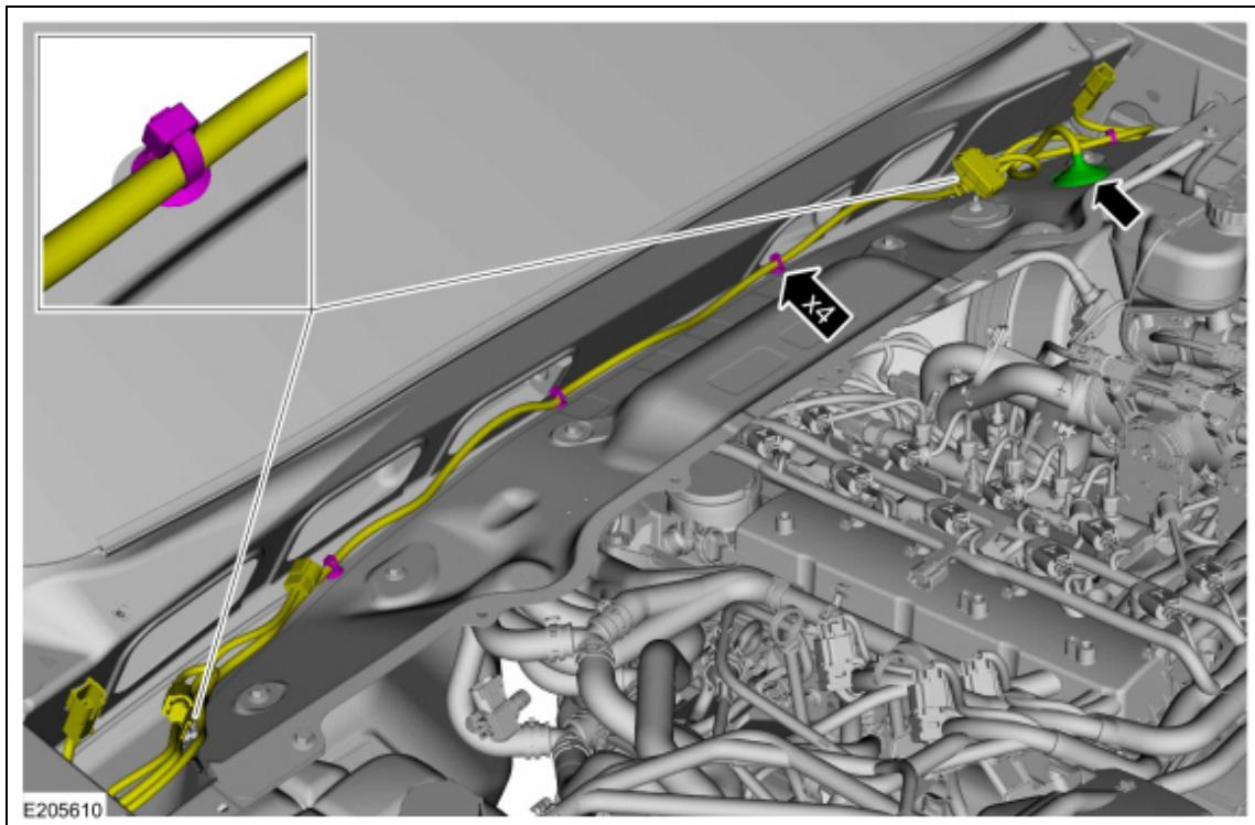
3. Remove the bolts, nut and the cowl panel.
