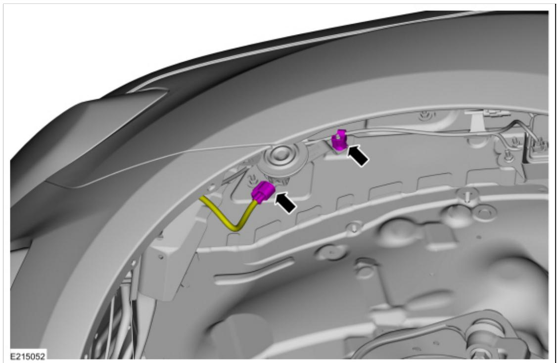
3. Remove the nut and the ant-theft alarm horn.
