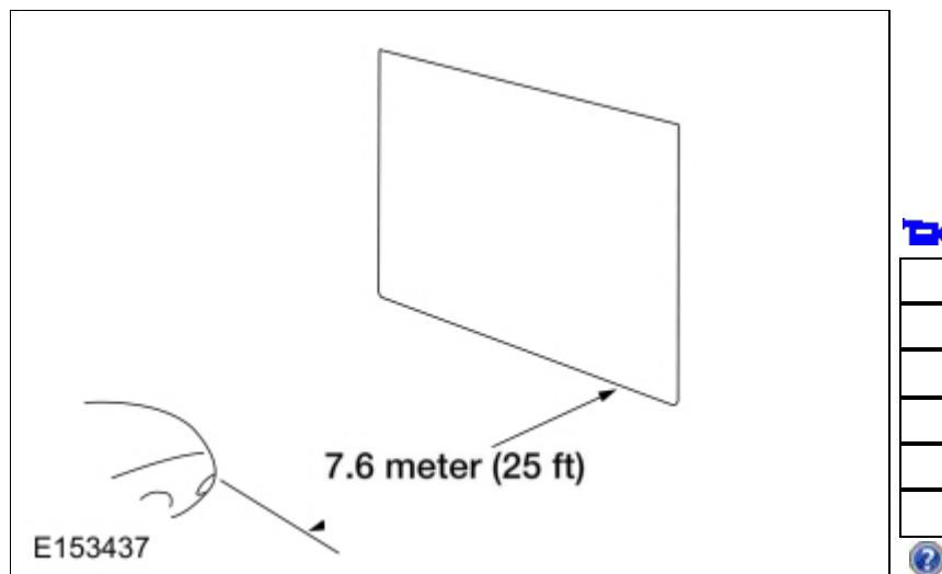
3. The correct visual aim for the fog lamps is with the top edge of the high-intensity zone 101.6 mm (4 in) below the horizontal center of the fog lamps.
