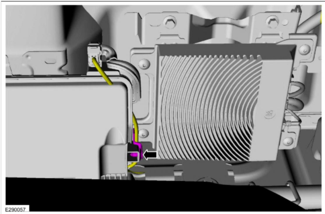
3. Disconnect the electrical connectors, remove the screws and the subwoofer speaker.
