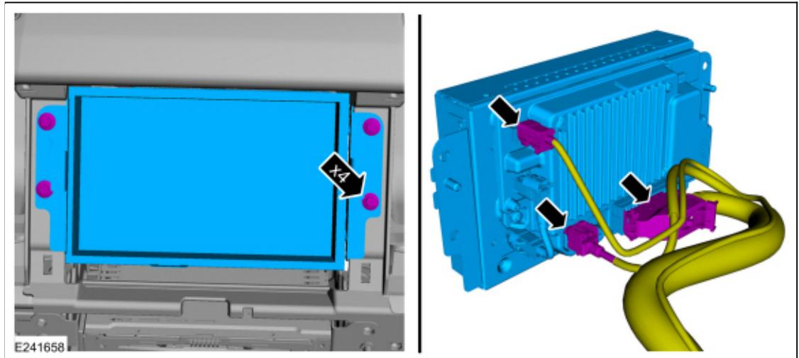
6. Remove the screws, disconnect the electrical connectors and remove the APIM.
