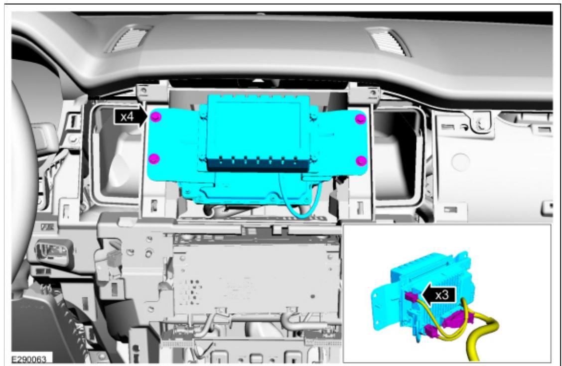
3. Disconnect the LVDS cable electrical connector.
