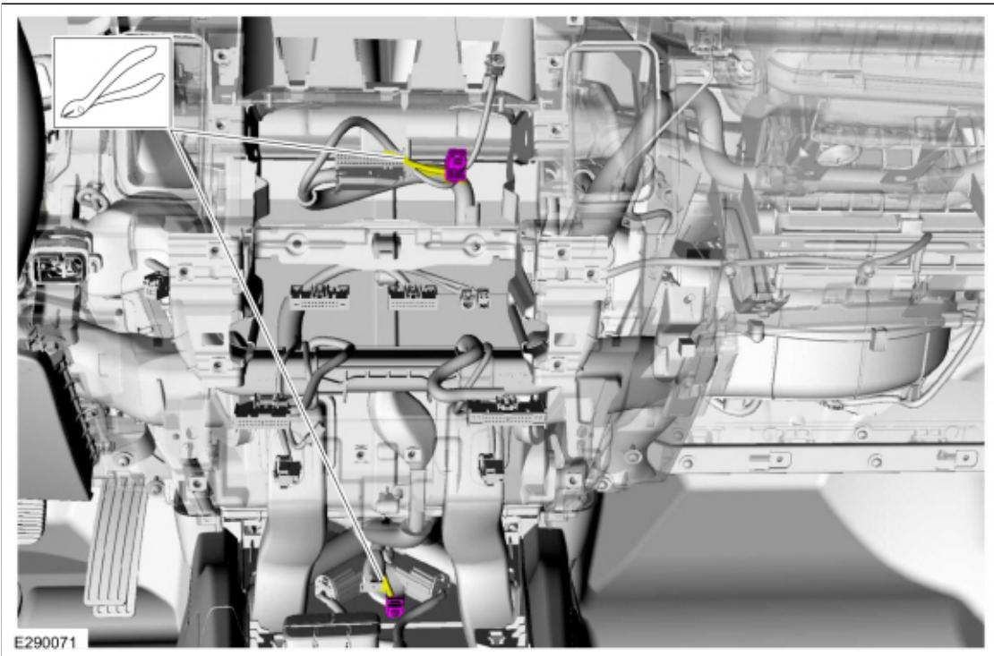
2. Overlay using the routing shown and secure the new USB cable and secure to the instrument panel wiring harness, as necessary to prevent NVH concerns.
