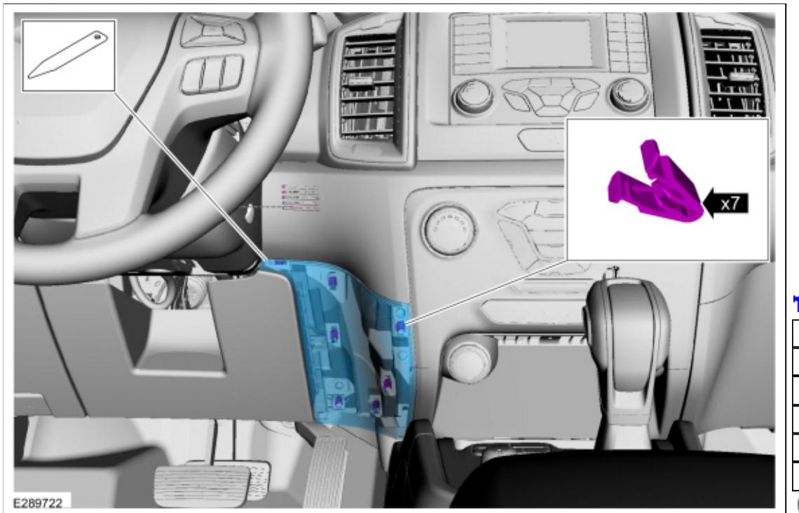
3. Using a non-marring tool, release the clips and remove the RH lower instrument panel closeout panel. Use the General Equipment: Interior Trim Remover
