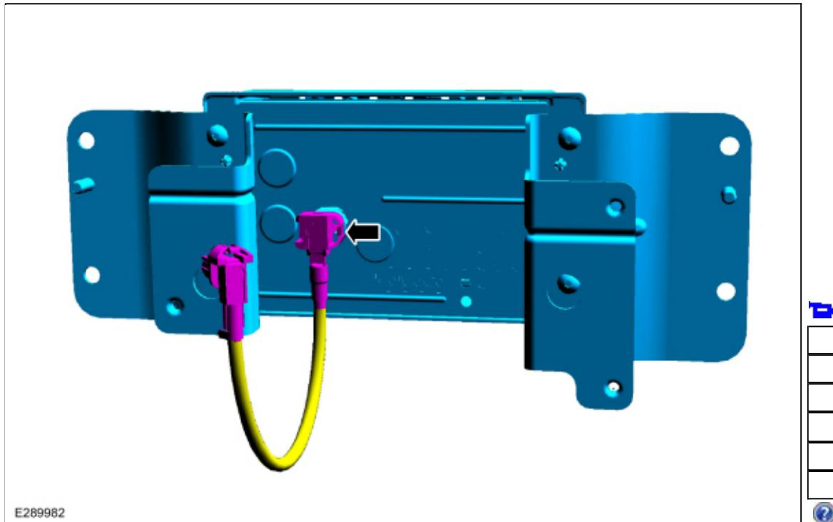
3. Remove the screws and FCDIM from the brackets.
