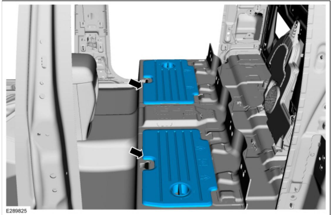
12. Remove the pin-type retainers and both under seat storage compartments.
