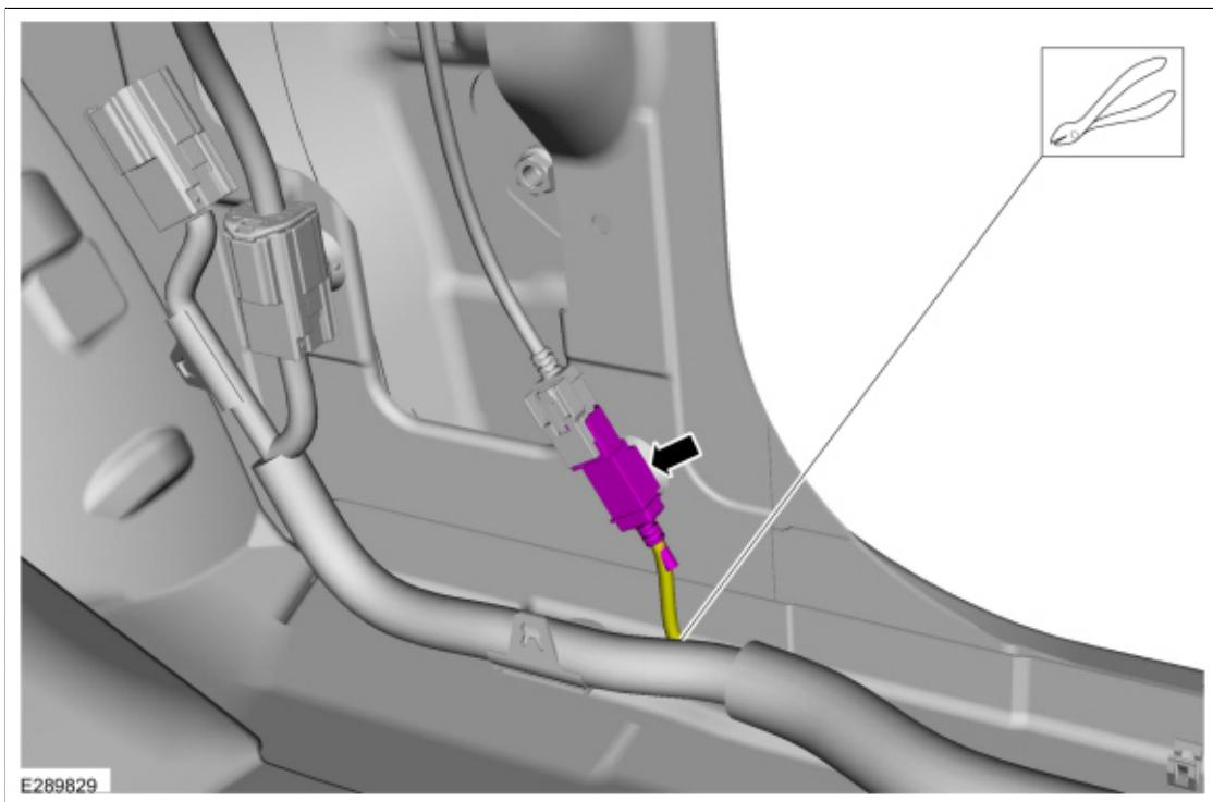
14. Disconnect and trim the electrical connector from the main body harness.
