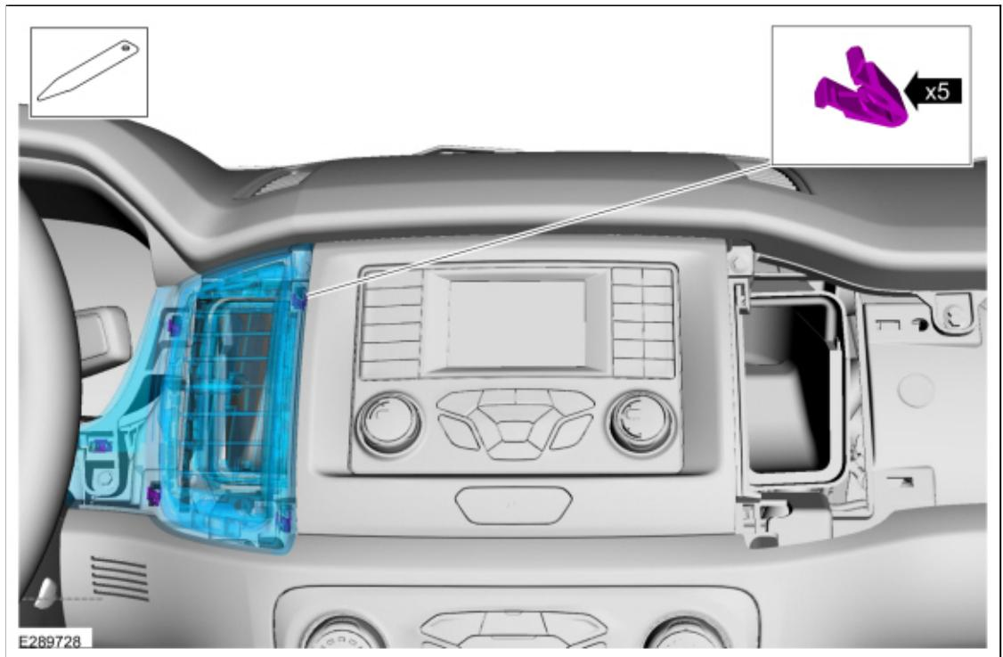
6. Using a non-marring tool, release the clips and remove the RH instrument panel center trim panel.
