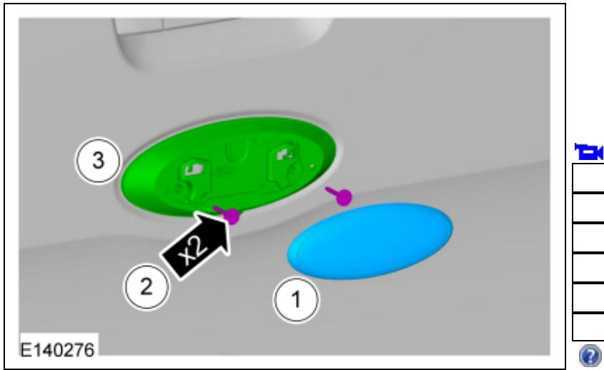
2. Remove the screws and the rear view camera bracket.
