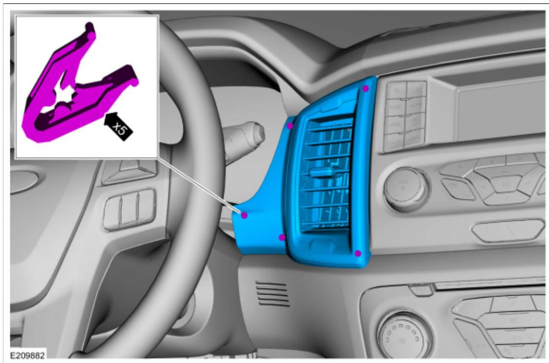
5. Remove bolts, release the clips and remove the IPC bezel.
