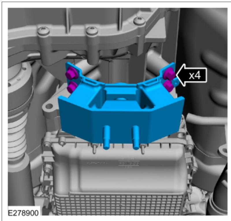
2. Tighten the transmission support insulator bolts in the sequence shown.
