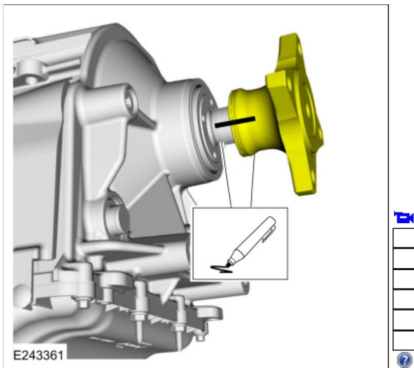
5. Remove the output shaft flange.
