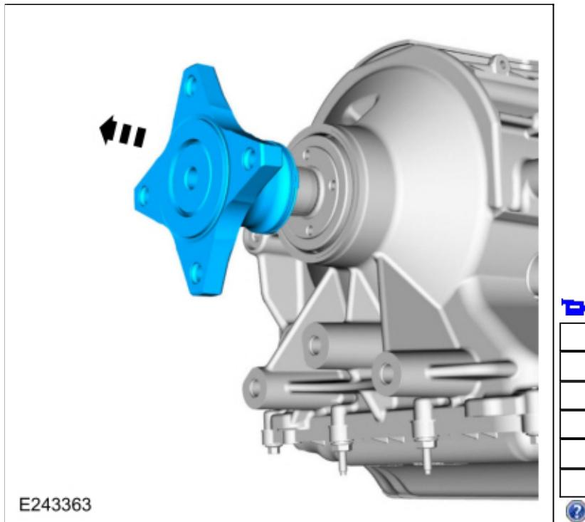
6. Using the special tool, remove and discard the output shaft nut (7085). Use Special Service Tool: [307-458 Socket, Output Shaft Locknut](#).
