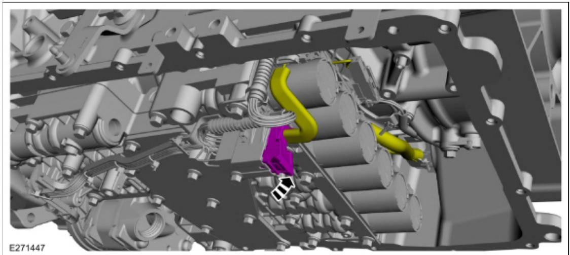
3. Remove the bolts and the main control valve body.
