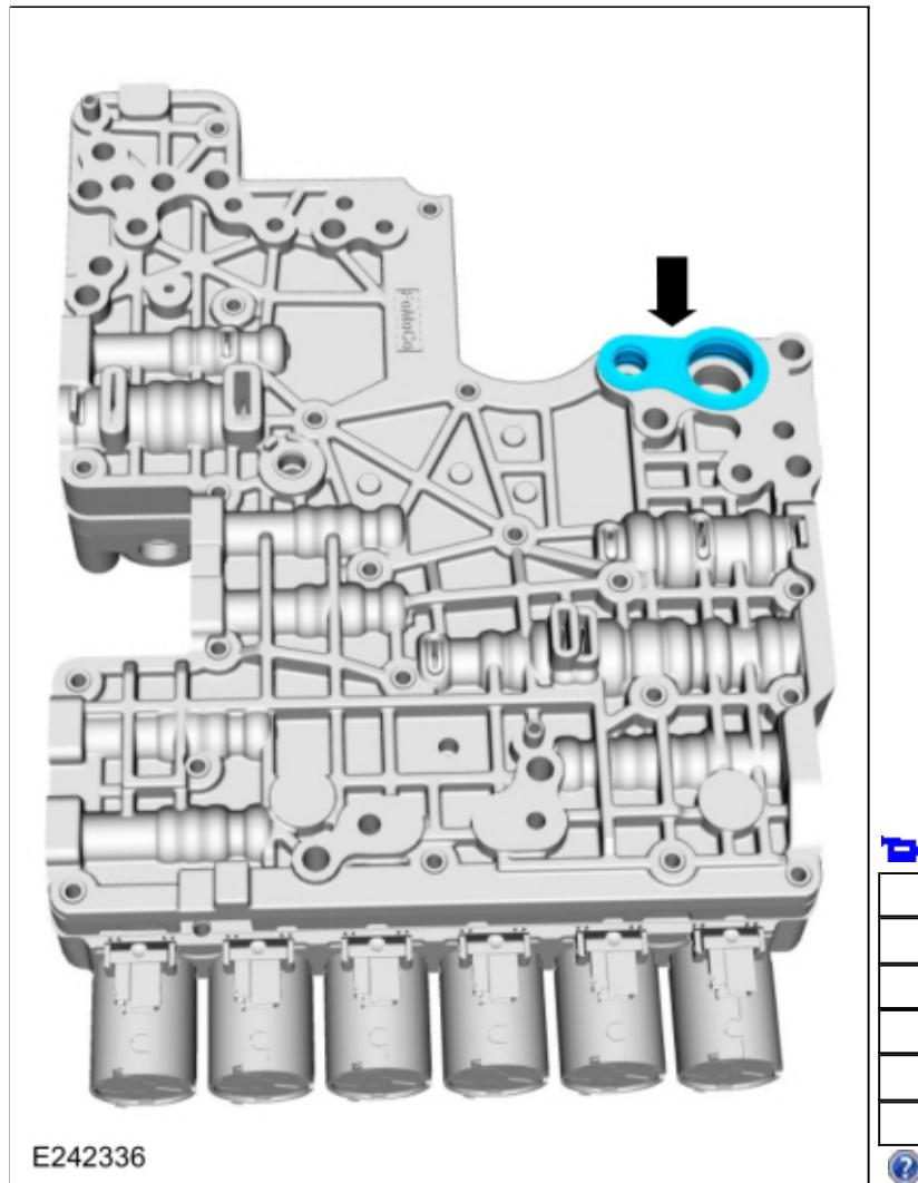
2. **NOTICE: Do not install a 71 mm length bolt in the location shown or the transmission clutch and planetary container will be damaged and result in transmission failure.**
