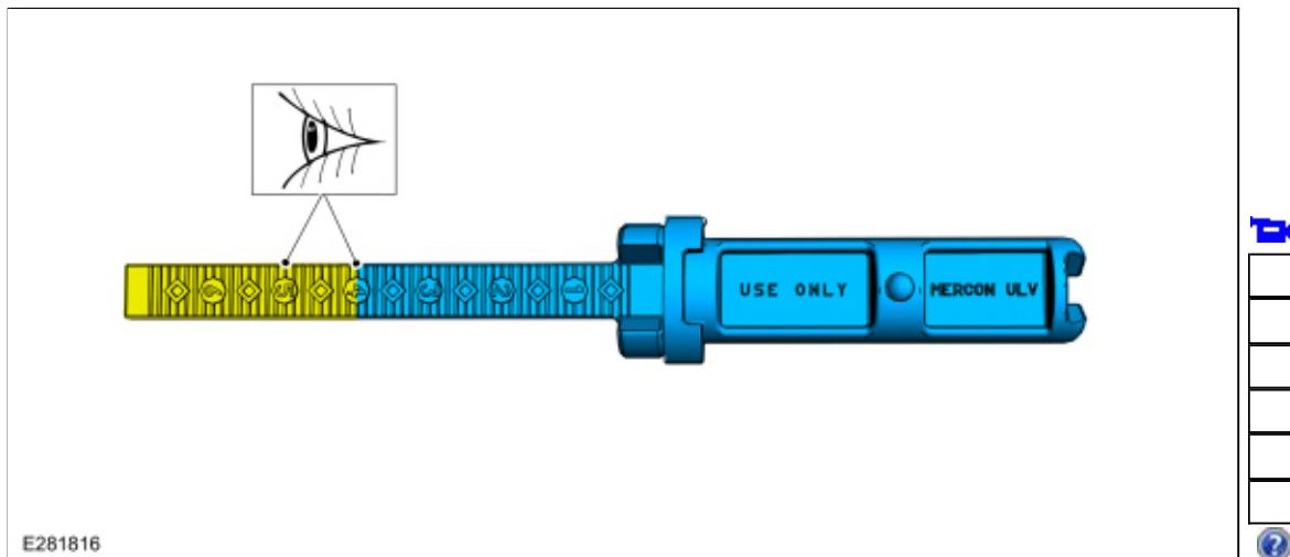
6. If the transmission fluid is not at the correct level, follow the steps for adding or removing transmission fluid.
