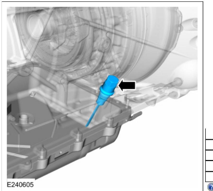
5. **NOTE:** The transmission fluid level indicator uses 1 through 6 to indicate the fluid level. The different numbers are for different vehicle models. Use the area between 4 and 5 when checking the transmission fluid level. The correct transmission fluid level is between 4 and 5 on the transmission fluid level indicator.
