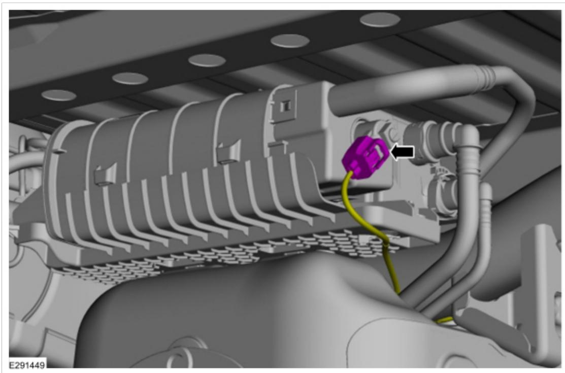
3. Rotate the EVAP canister solenoid clockwise and remove the EVAP canister solenoid.
