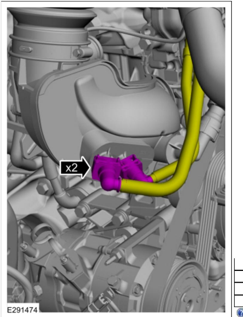
4. Disconnect the quick connect coupling and detach the wiring harness straps.
