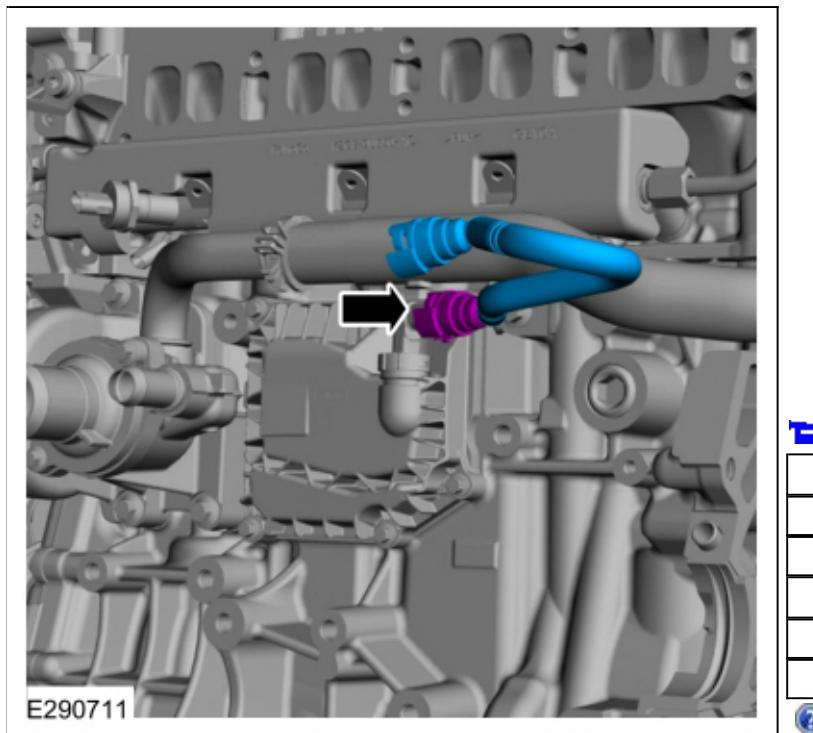
3. Inspect the crankcase vent oil separator gasket.
