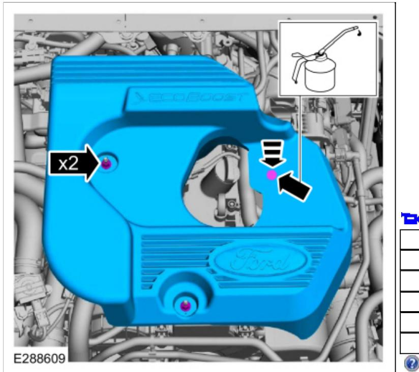
14. Check the engine oil level and fill as needed.
