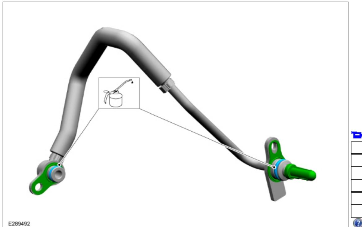
**2. NOTE: The oil supply tube must be fully seated prior to fastener tightening.**
