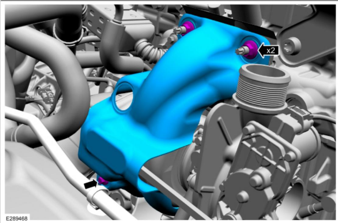
11. Remove the bolts, then remove and discard the turbocharger oil supply tube.
