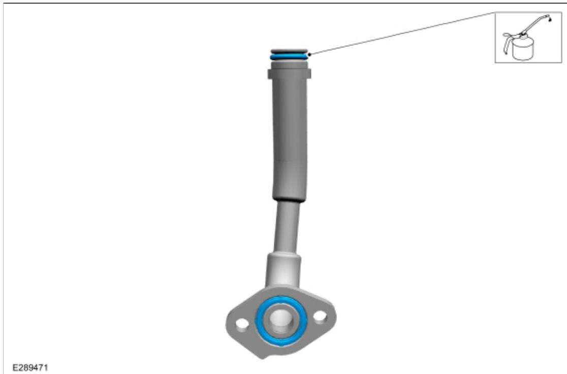
**2. NOTICE: Do not use a metal brush, damage to sealing area will result in leaks.**
