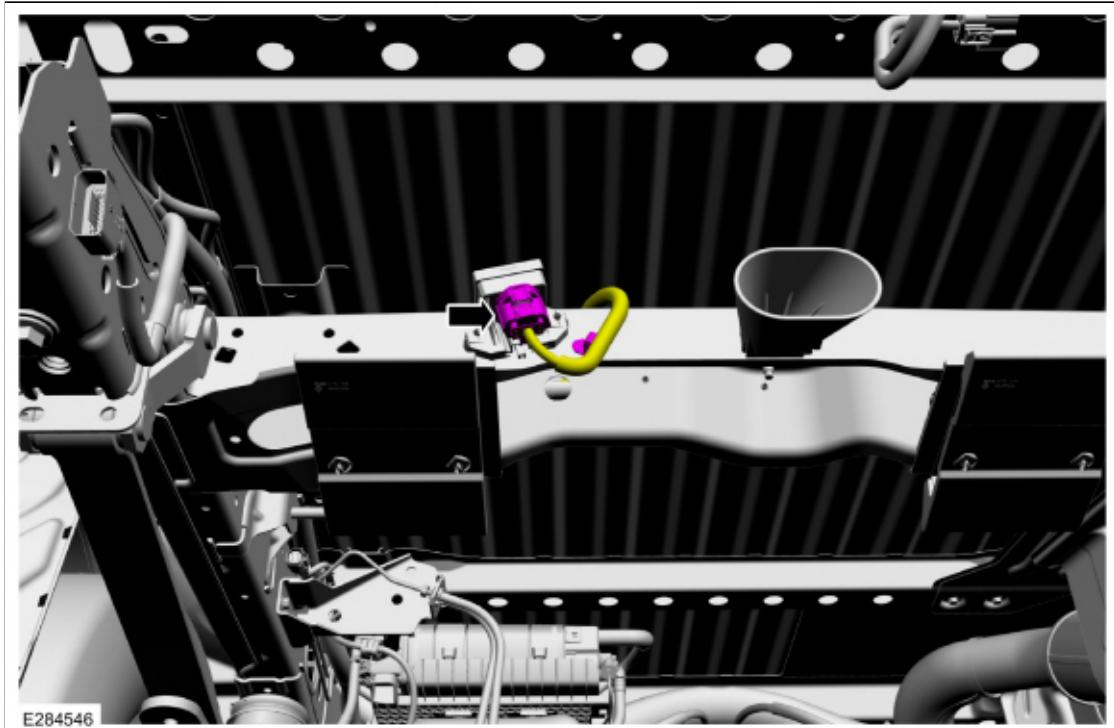
4. Remove the fuel pump driver module fasteners, then remove the fuel pump driver module.
