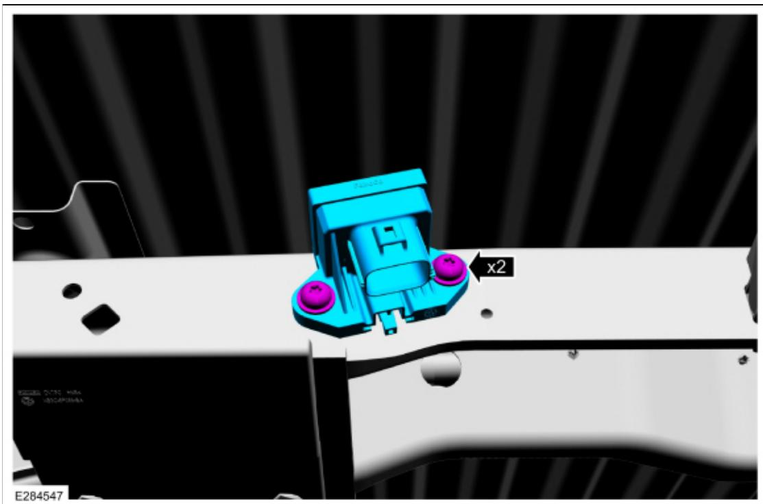
2. Connect the fuel pump driver module electrical connector.
