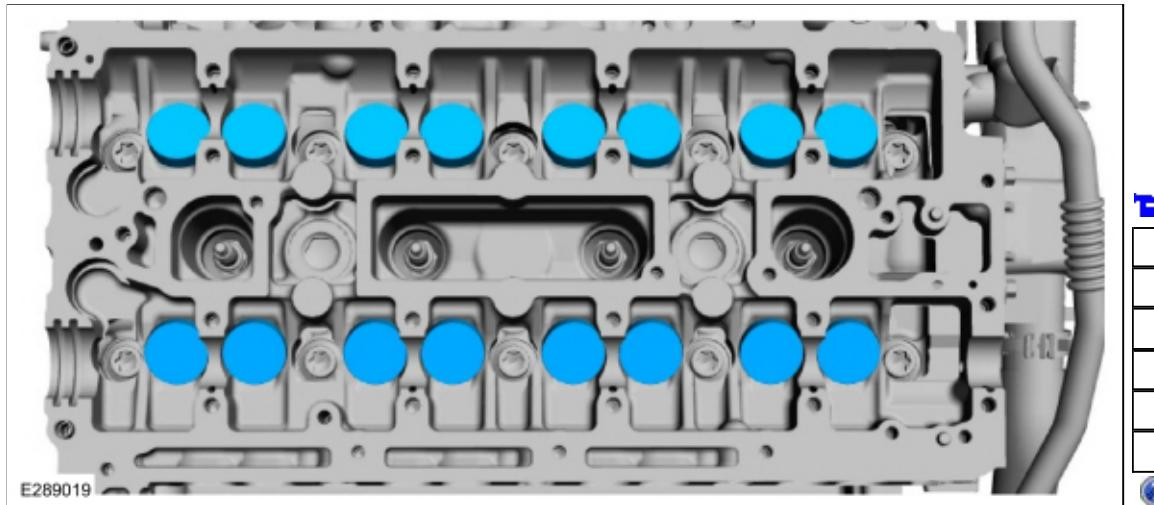
3. **NOTE:** There are two numbers on the valve tappet, one is date code and the other is valve tappet thickness.
