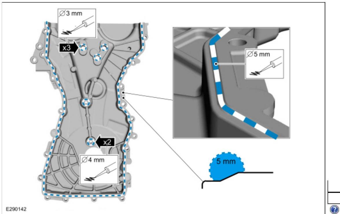
5. **NOTE:** The engine front cover must be secured within 10 minutes of Silicone Gasket and Sealant application. If the engine front cover is not secured within 10 minutes, the sealant must be removed and the sealing area cleaned.
