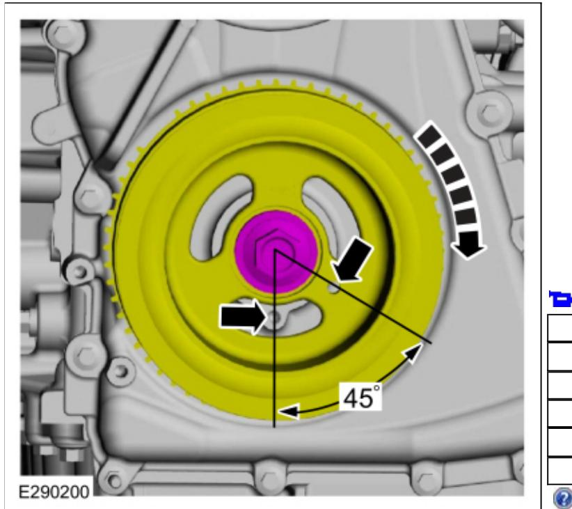
31. Remove the engine plug bolt.
