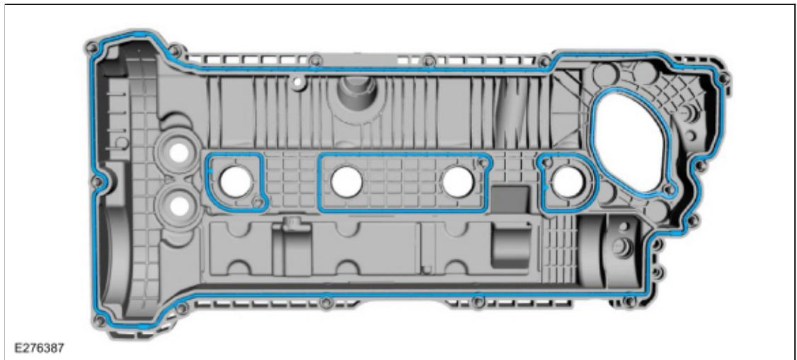
28. Apply a 5.5 mm (0.22 in) bead of silicone sealant in the 4 places shown.
