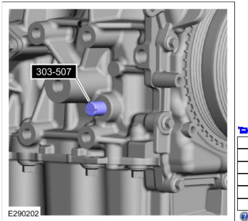
33. **NOTE:** The Crankshaft TDC Timing Peg will contact the crankshaft and prevent it from turning past TDC. However, the crankshaft can still be rotated in the counterclockwise direction. The crankshaft must remain at the TDC position during the crankshaft pulley removal and installation.
