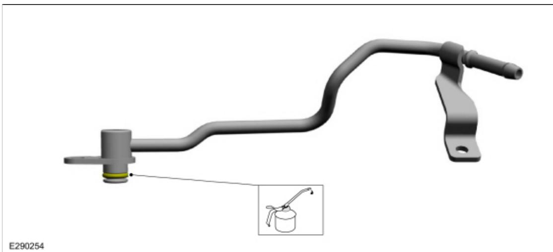
45. Install the coolant tube and the bolts.
