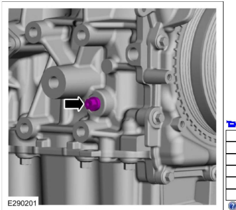
32. Install Special Service Tool: [303-507 Timing Peg, Crankshaft TDC](#).
