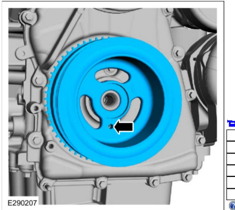
13. **NOTE:** This step will correctly align the crankshaft pulley to the crankshaft.
