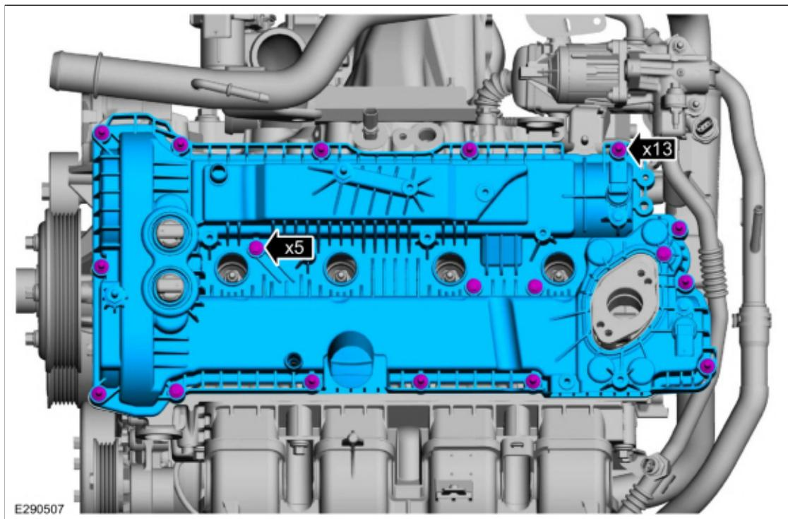
22. Remove and discard the valve cover gaskets.
