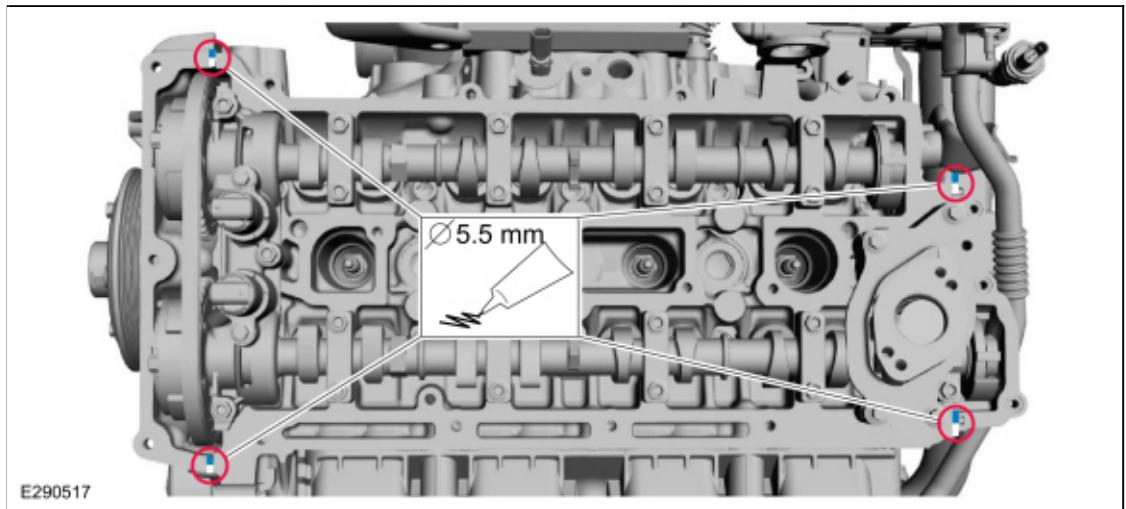
29. **NOTE:** The valve cover must be secured within 10 minutes of silicone gasket application. If the valve cover is not secured within 10 minutes, the sealant must be removed and the sealing area cleaned.
