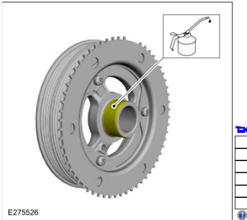
12. Position the crankshaft pulley onto the crankshaft with the access hole at the 6 o'clock position.
