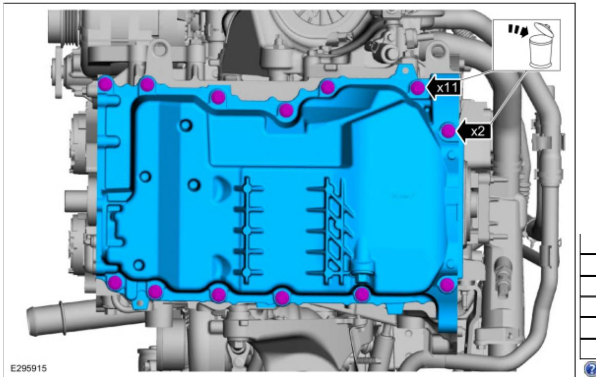
46. **NOTICE: Only use a 3M™ Roloc® Bristle Disk (2-in white, part number 07528) in a suitable tool turning at the recommended speed of 15,000 rpm, to clean the oil pan. Do not use metal scrapers, wire brushes or any other power abrasive disk to clean. These tools cause scratches and gouges that make leak paths.**
