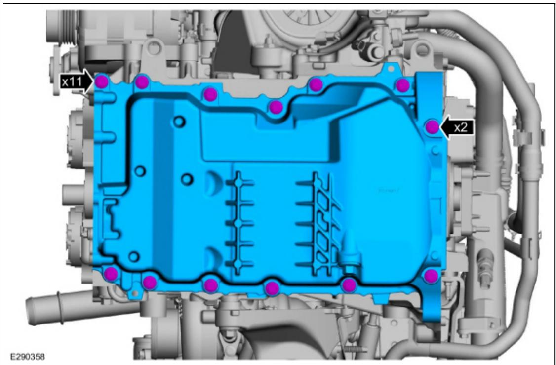
3. Tighten the bolts in sequence shown.
