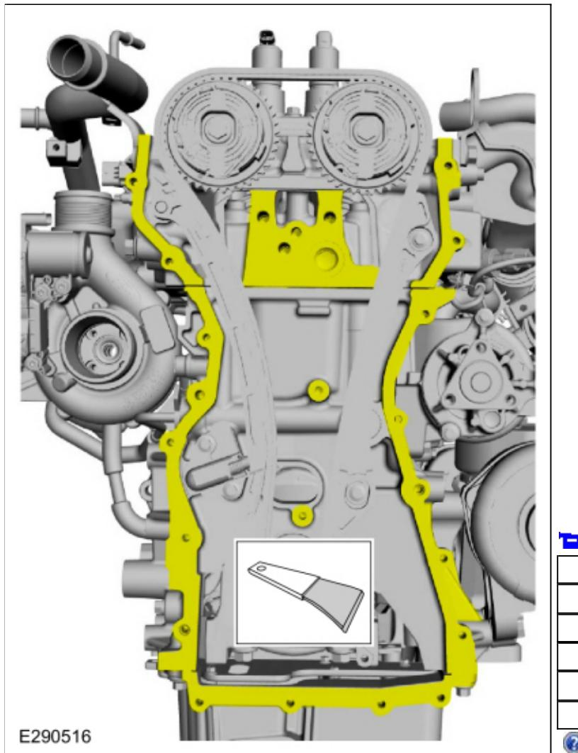
45. **NOTICE: Do not strike the oil pan sideways to remove, the oil pan is doweled and will damage the oil pan and engine block.**
