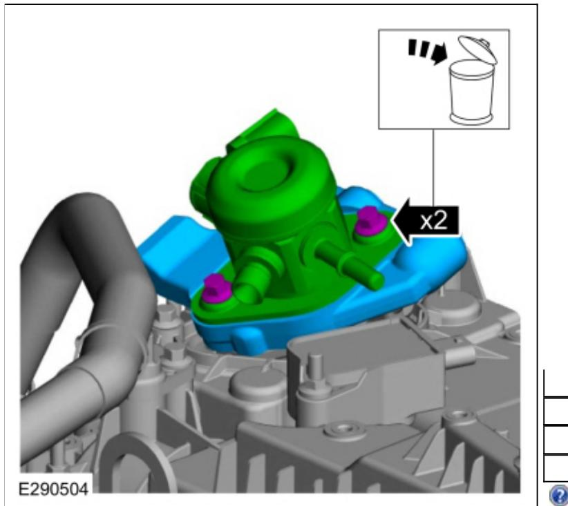
17. Remove and discard the high-pressure fuel pump O-ring seal.
