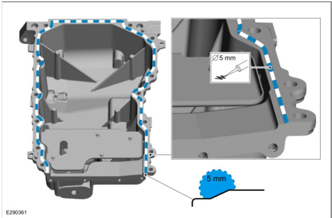
2. Install the oil pan and the new bolts finger-tight.
