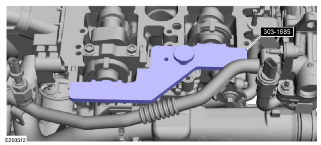
24. Install the high-pressure fuel pump drive unit and the bolts.
