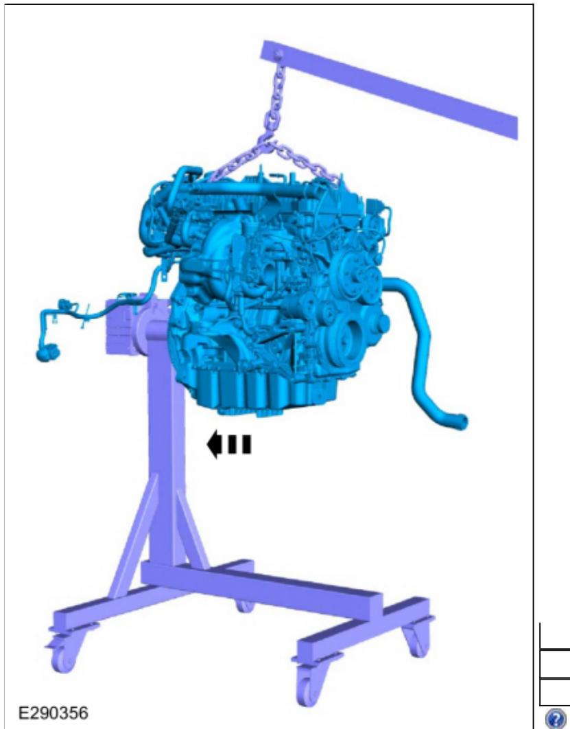
4. Remove the engine lift equipment.
