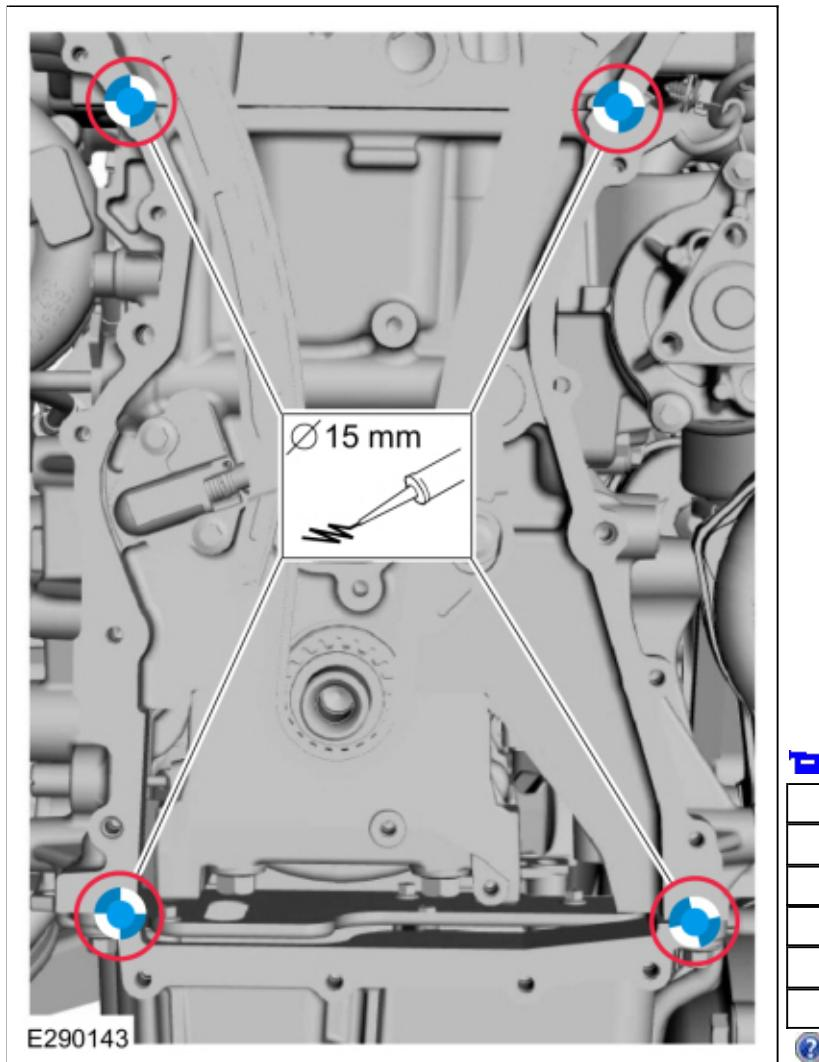
6. Install the engine front cover and the fasteners and tighten in the sequence shown.
