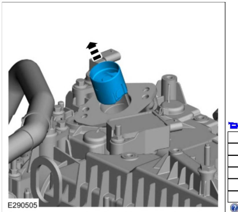
20. **NOTE:** Use compressed air to remove any foreign material from the ignition coil-on-plugs and surrounding area before removing the ignition coil-on-plugs.
