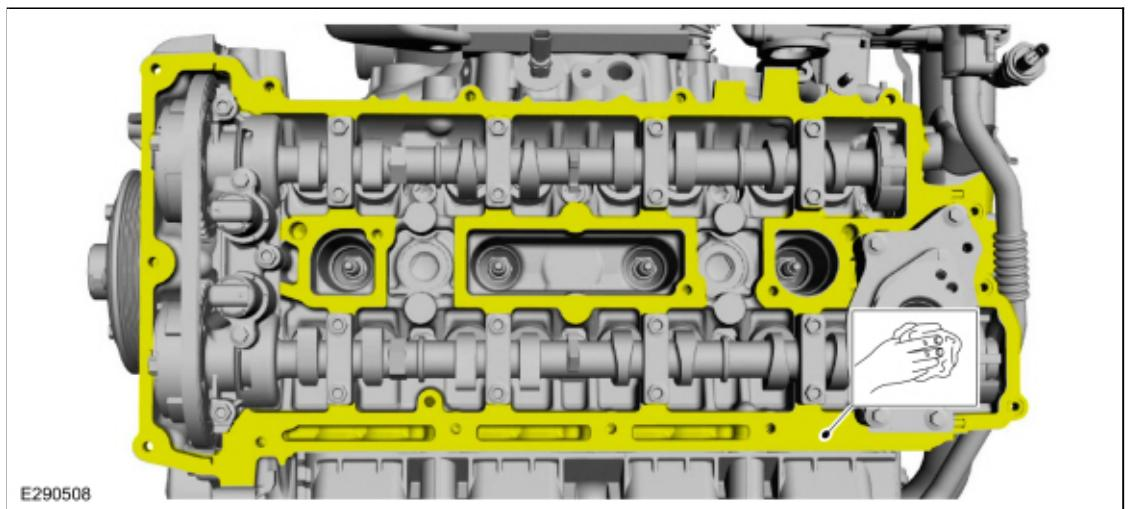
26. Remove the bolts and the high-pressure fuel pump drive unit.
