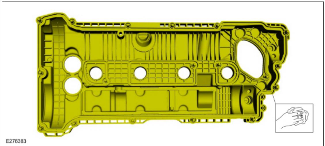
25. **NOTICE:** Do not use metal scrapers, wire brushes, power abrasive discs or other abrasive means to clean the sealing surfaces. These tools cause scratches and gouges which make leak paths.
