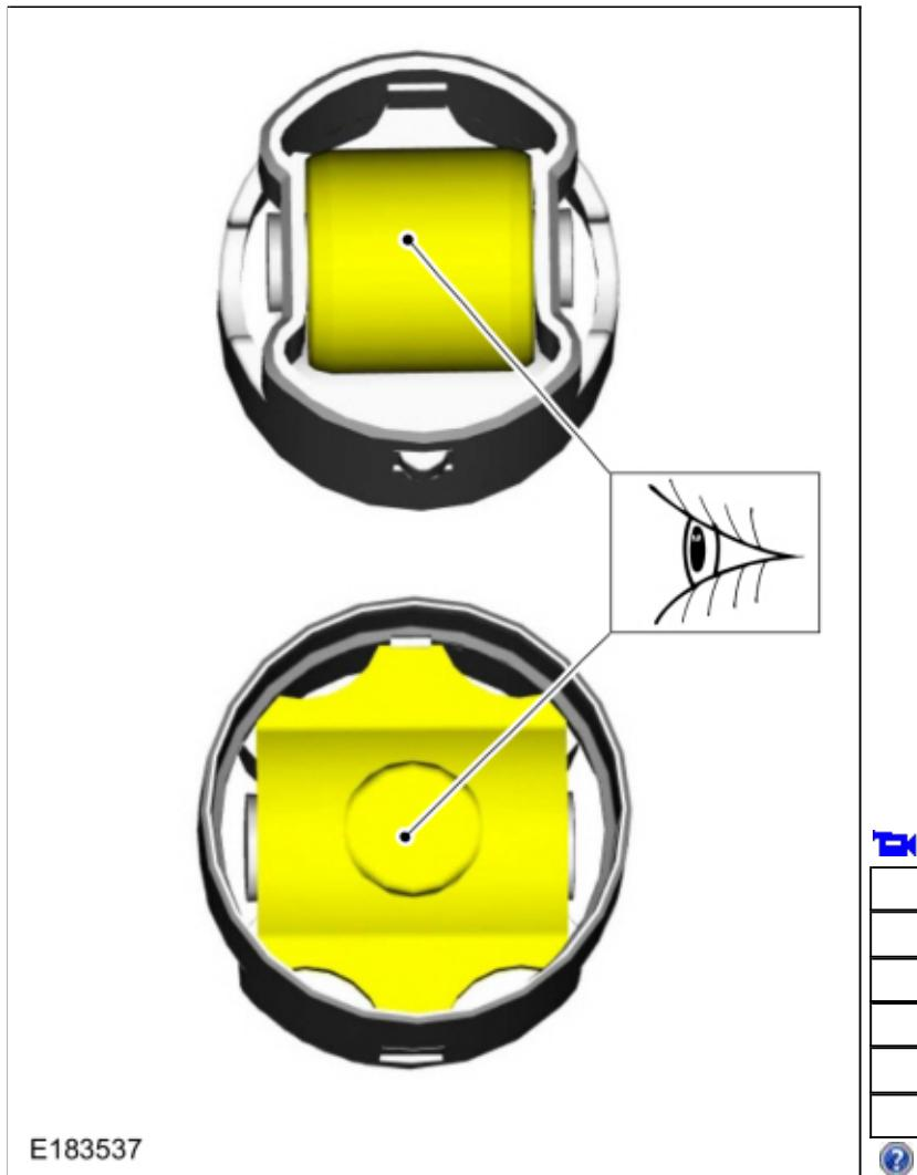
34. Lubricate with clean engine oil and install the high-pressure fuel pump tappet.
