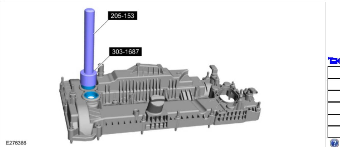
27. Install a new valve cover gaskets.
