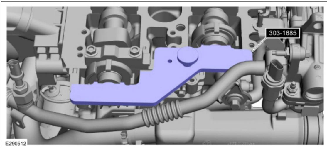
35. **NOTICE:** The crankshaft must remain in the TDC position during removal of the pulley bolt or damage to the engine can occur. Therefore, the crankshaft pulley must be held in place with the Crank Damper Holding Tool and the bolt should be removed using an air impact wrench (1/2-in drive minimum).
