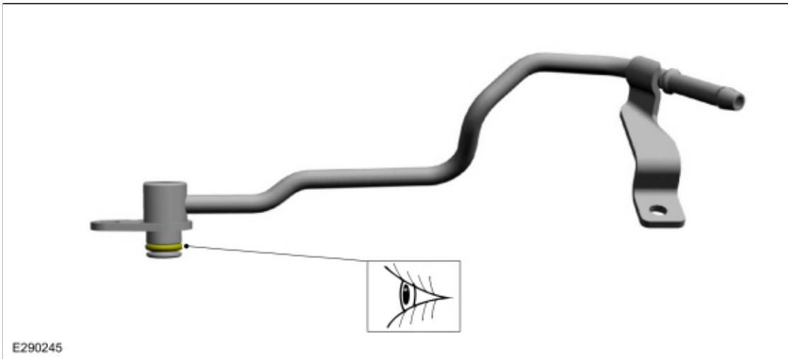
12. Remove the bolt and position the coolant tube aside.
