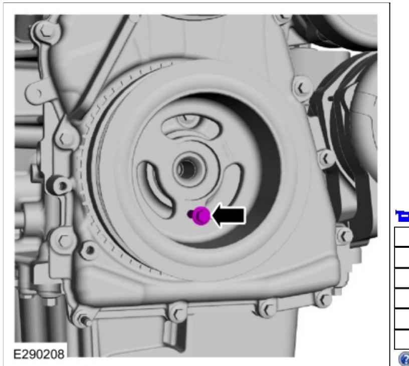
14. **NOTICE:** The crankshaft must remain in the TDC position during installation of the pulley bolt or damage to the engine can occur. Therefore, the crankshaft pulley must be held in place with the Crank Damper Holding Tool and the bolt should be installed using hand tools only.
