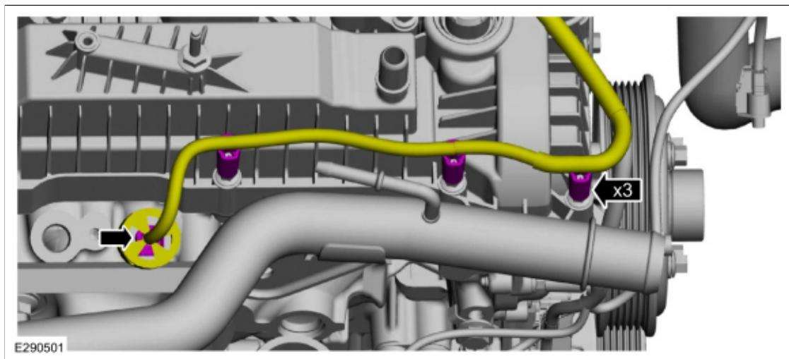
43. Position the coolant tube and install the bolt.
