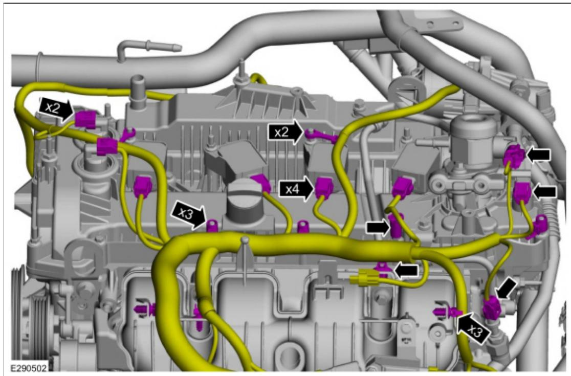
42. Connect the CHT sensor wiring harness electrical connector and attach the retainers.
