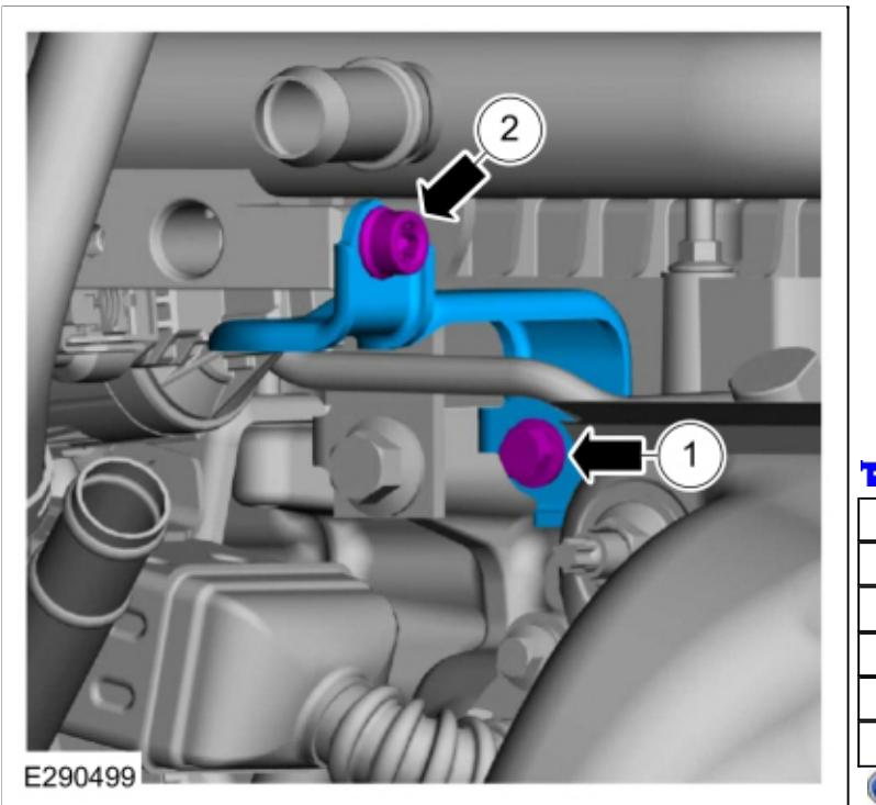
10. Remove the bolts and position the coolant tube aside.
