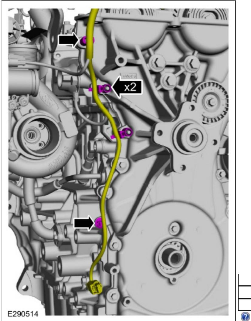
42. Remove the fasteners and the engine front cover.
