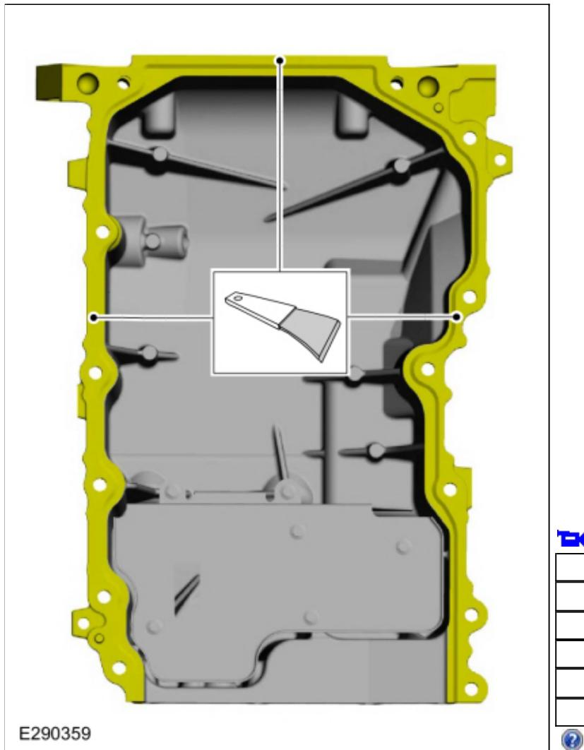
47. **NOTICE: Do not use wire brushes, power abrasive discs or 3M™ Roloc® Bristle Disk (2-in white, part number 07528) to clean the sealing surfaces of the engine block. These tools cause scratches and gouges that make leak paths. They also cause contamination that causes premature engine failure. Remove all traces of the gasket.**
