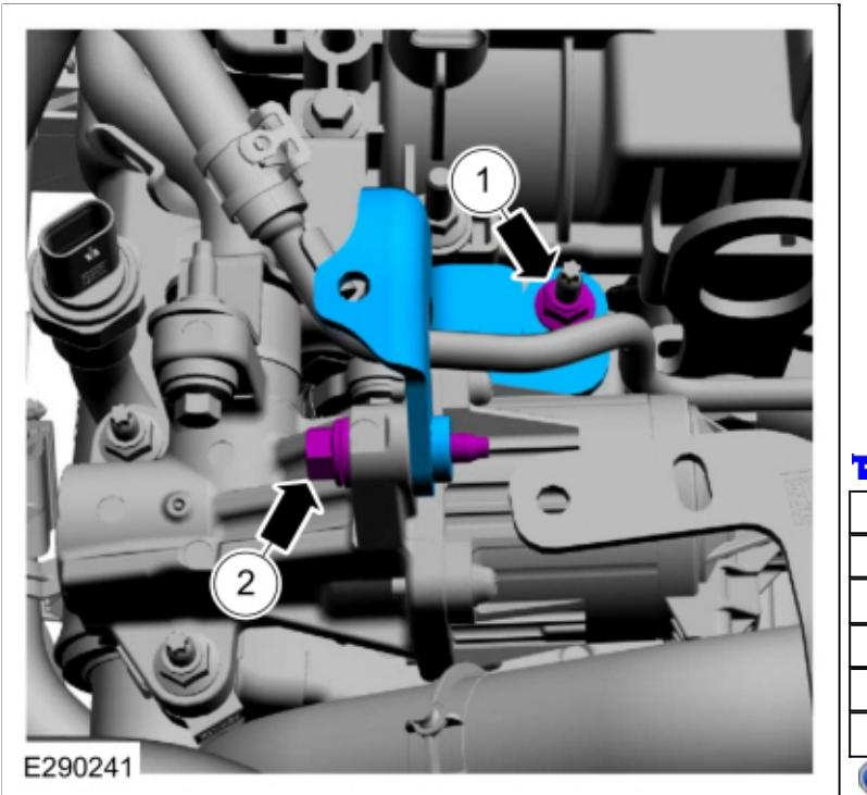
8. Remove the bolt and position the turbocharger coolant tube aside.
