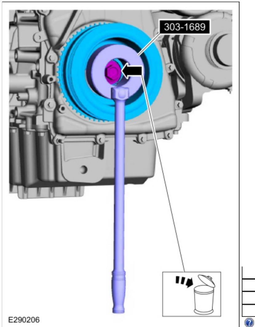
36. Install the old crankshaft pulley bolt.
