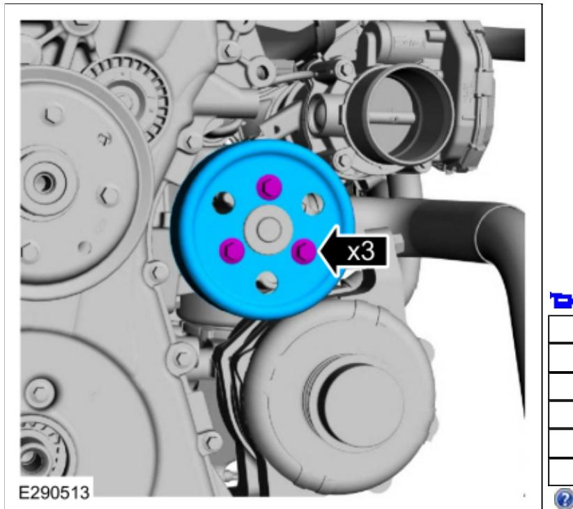
40. Remove the bolts and the accessory drive belt pulley.
