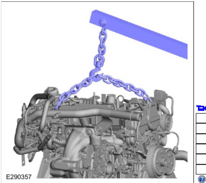
52. Using a floor crane, remove the engine from the mounting stand.
