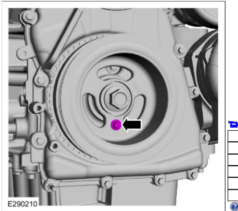
16. **NOTE:** Do not tighten the CKP sensor bolts at this time.
