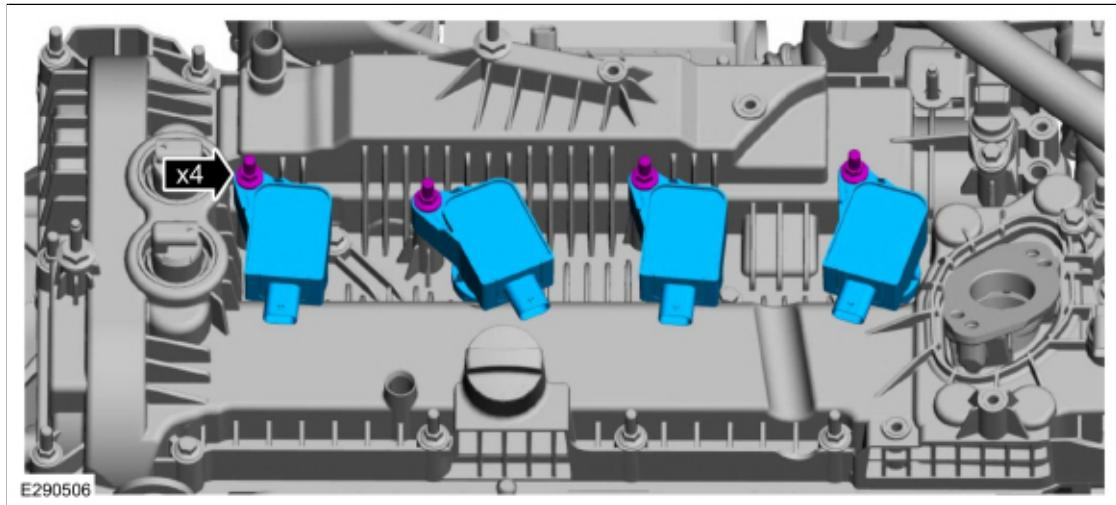
21. Loosen the fasteners and remove the valve cover.
