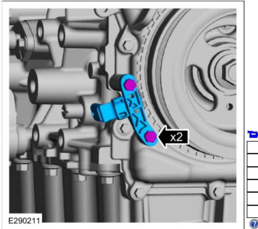
17. Install the special tool onto the CKP sensor and the tooth of the crankshaft pulley trigger wheel. Use Special Service Tool: [303-1521 Alignment Tool, Crankshaft Position Sensor](#).
