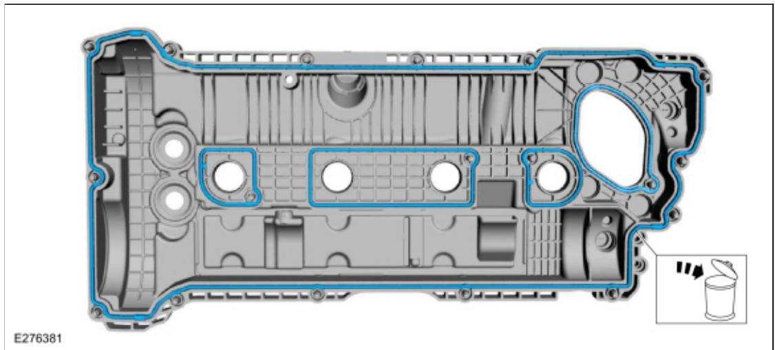
23. **NOTE:** The VCT solenoid seals should only be replaced if they are damaged.
