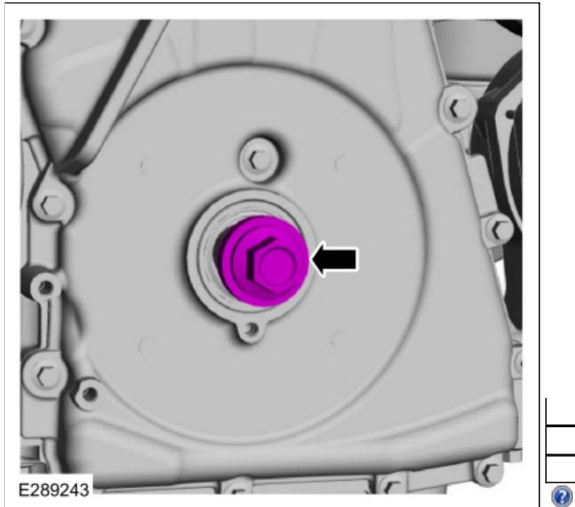
**37. NOTICE: Use care not to damage the engine front cover or the crankshaft when removing the seal.**
