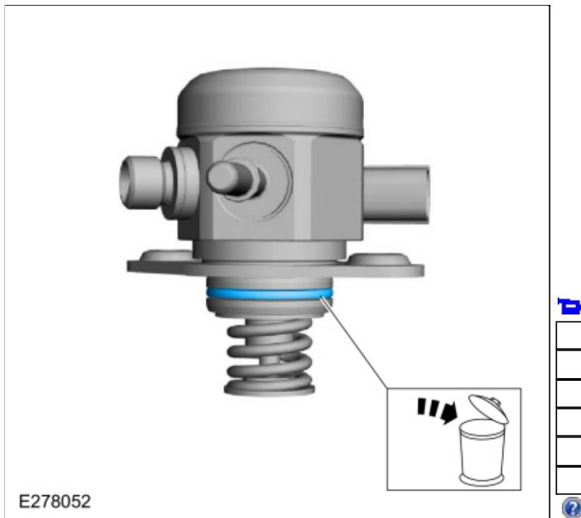
18. Remove and discard the fuel pump mounting plate O-ring seal.
