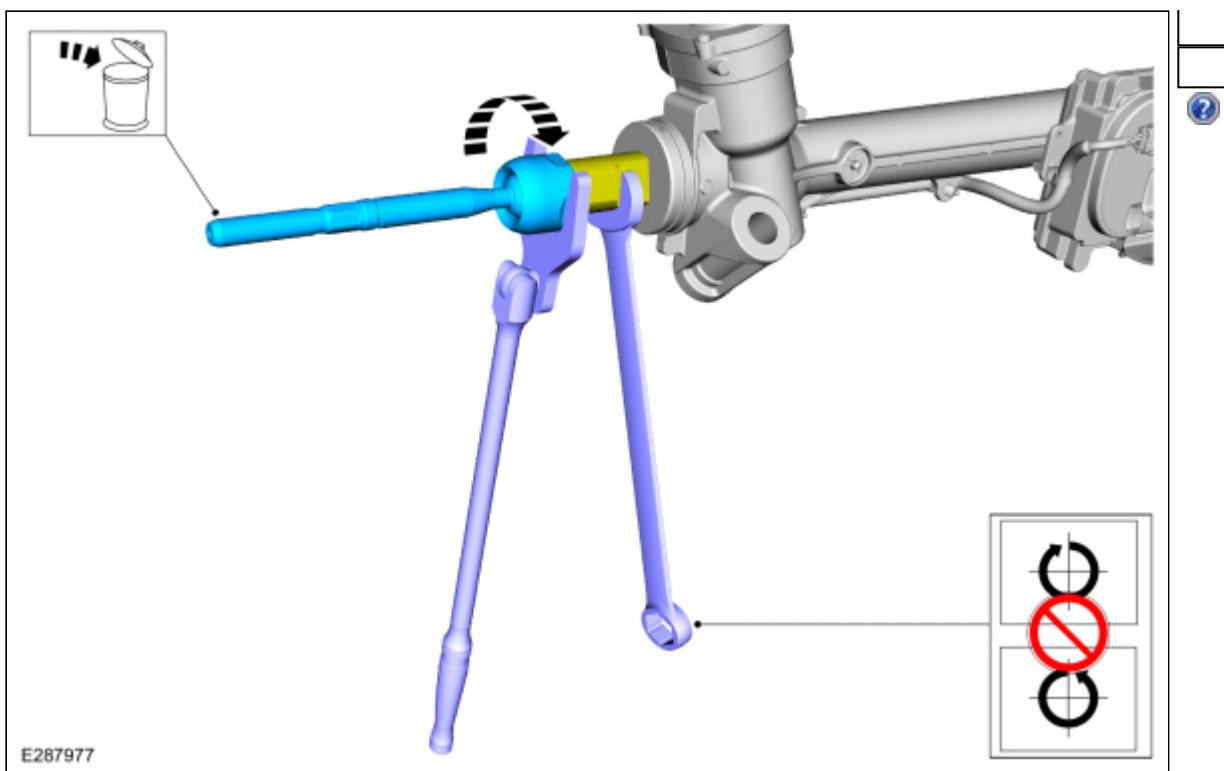
2. Install the steering gear boot.
