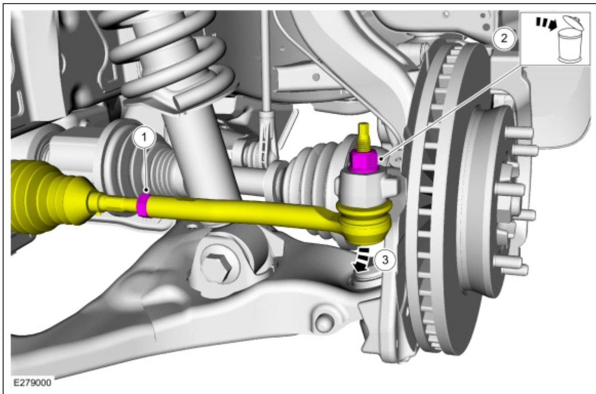
4. **NOTE:** Count and record the number of turns required to remove the outer tie-rod end for reference during installation.
