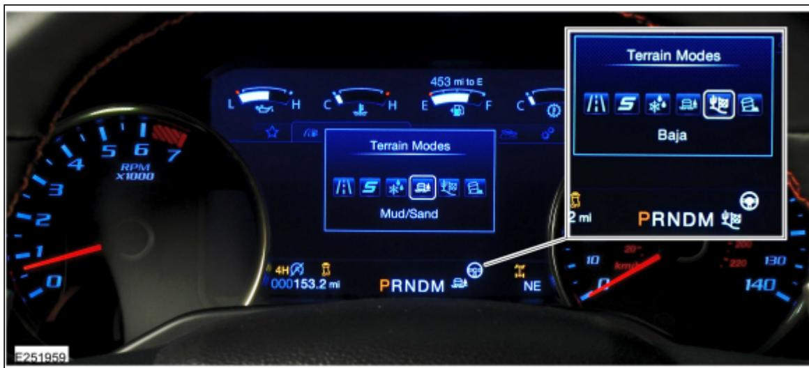
If the vehicle is equipped with the terrain management system, the steering feel changes when a new terrain mode is selected. This automatic selection can be overridden by using the selectable steering button.
