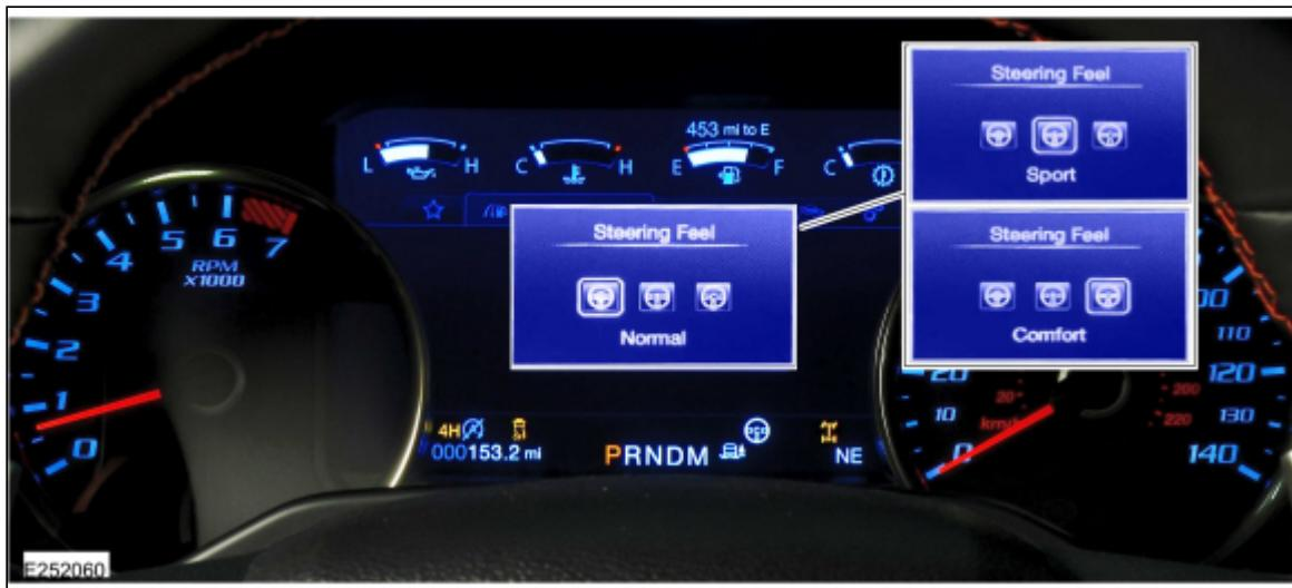
Pressing the switch sends a message to the IPC and the PSCM. The IPC displays the current mode in the message center and the PSCM modifies EPAS operation according to the selected steering mode:
