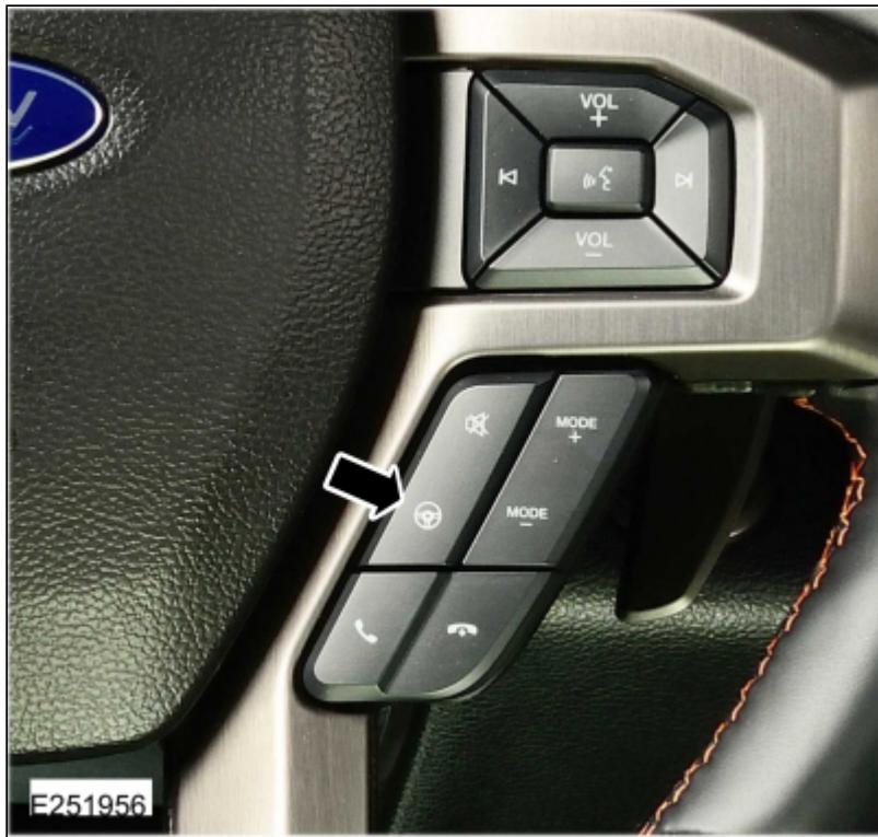
The selectable steering feature allows the driver to select 1 of 3 steering modes. These steering modes alter the feel and response of the EPAS system. Each steering mode can be selected using the selectable steering button on the steering wheel.
