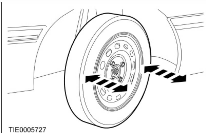
11. With the aid of another technician holding the steering against the left-hand steering lock stop, firmly grasp the left-hand road wheel and apply a rocking motion checking for any free play in the steering linkage.
