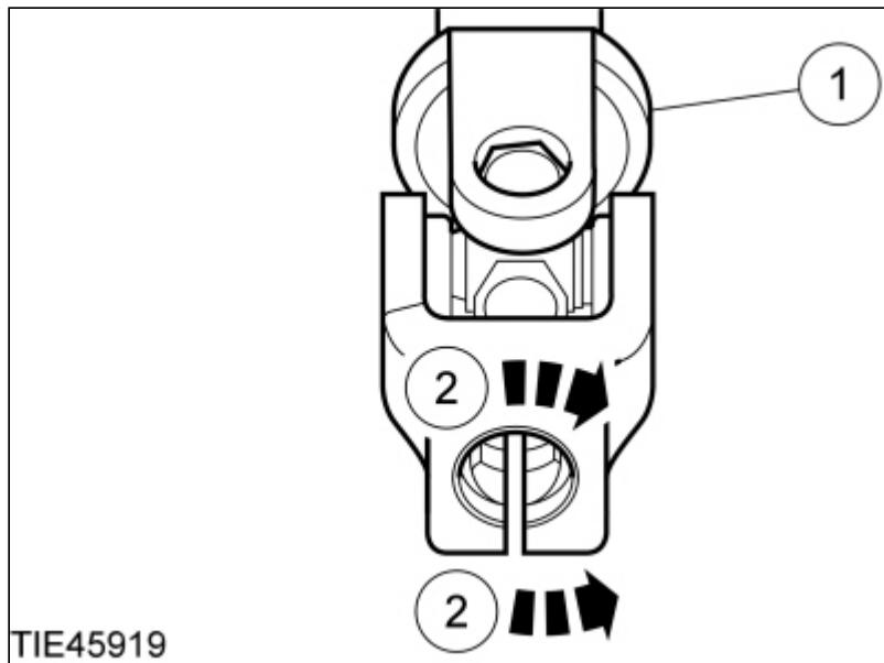
2. Check for smooth movement of the steering column universal joint.
