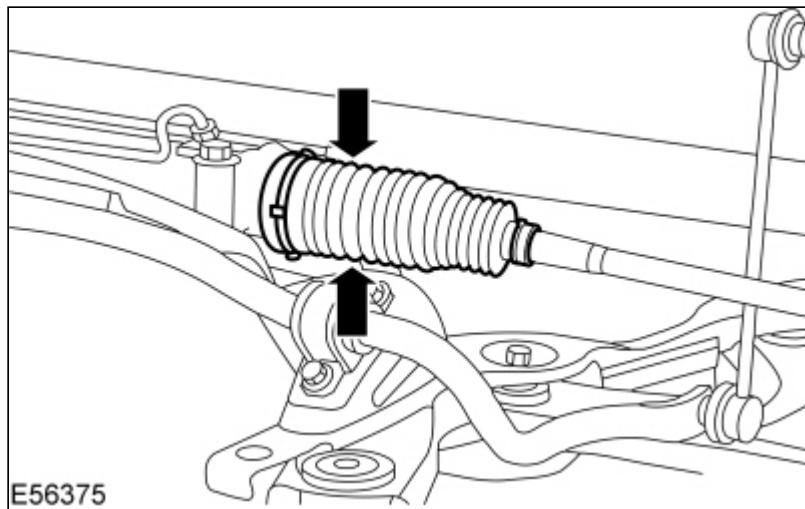
12. Detach the steering gear boot from the steering gear body and check for free play at the tie-rod inner ball joint.
