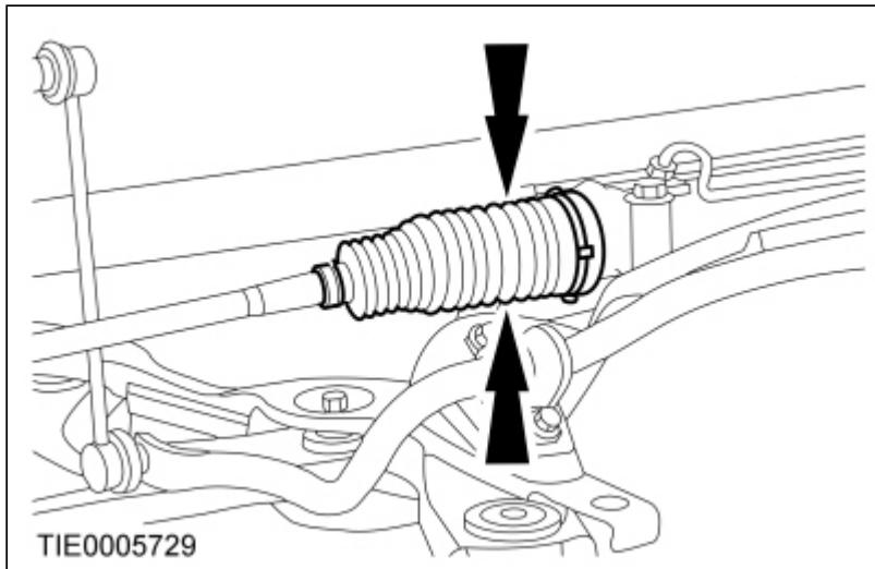
6. Detach the steering gear boot from the steering gear body and check for free play at the tie-rod inner ball joint.
