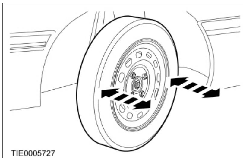
5. With the aid of another technician holding the steering linkage against the right-hand steering lock stop, firmly grasp the right-hand road wheel and apply a rocking motion checking for any free play in the steering linkage.
