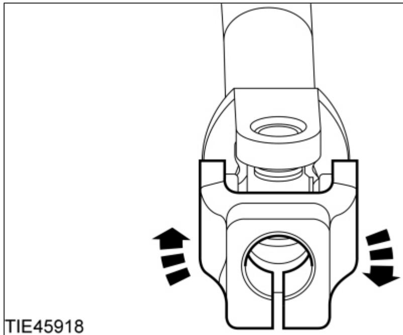
3. Hold both of the steering column universal joint yokes and twist them clockwise and counterclockwise.
