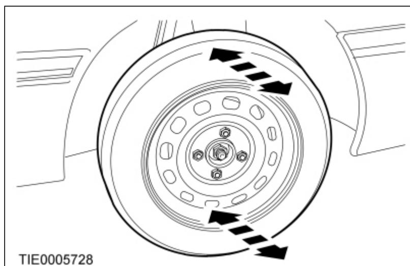
3. Firmly grasp the road wheel and apply a rocking motion checking for any free play in the wheel bearing or suspension components.
