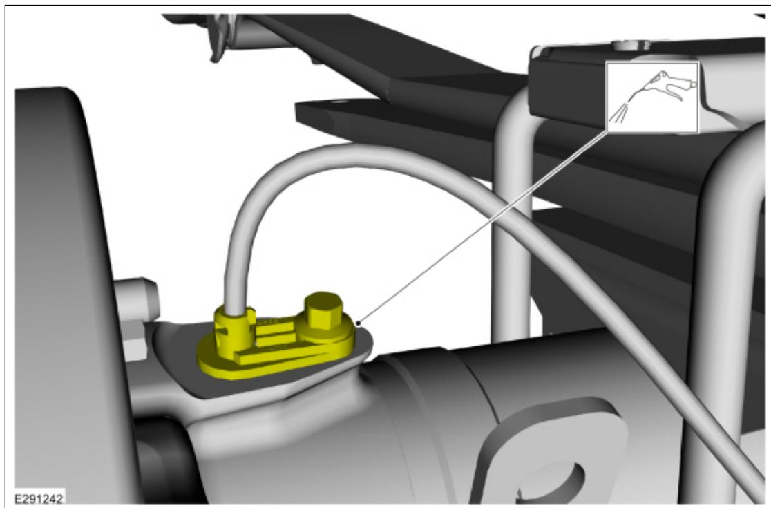
4. Remove the bolt and the wheel speed sensor.
