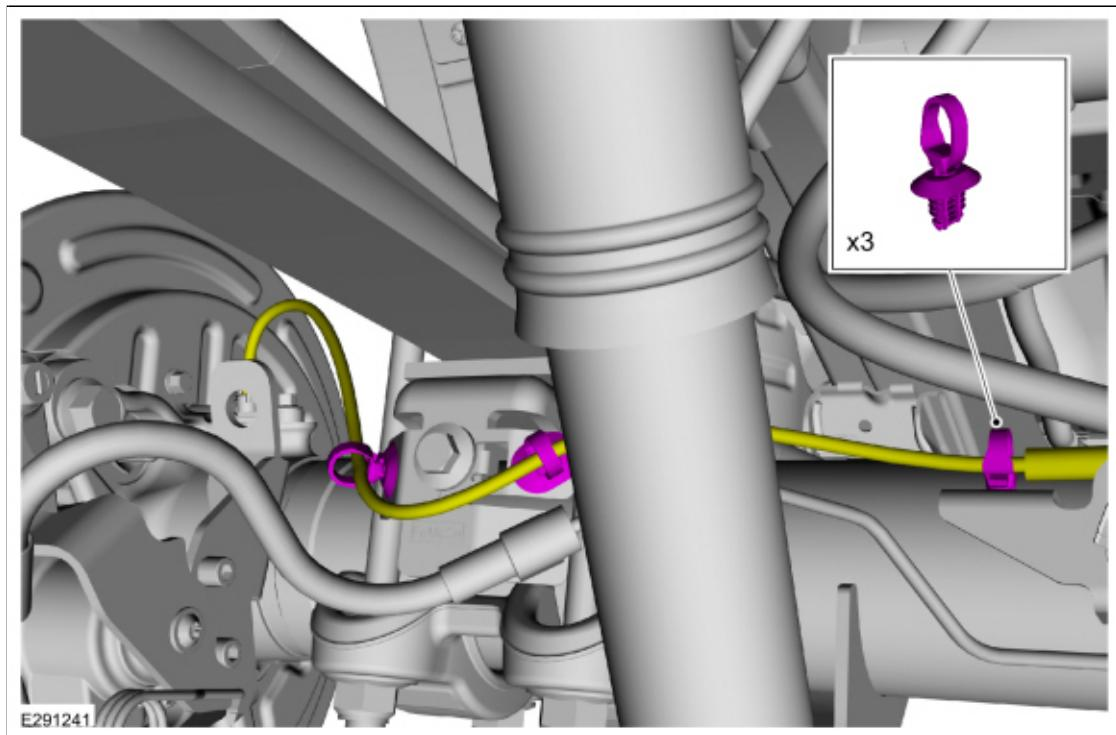
3. Using compressed air, clean the area surrounding the rear wheel speed sensor.
