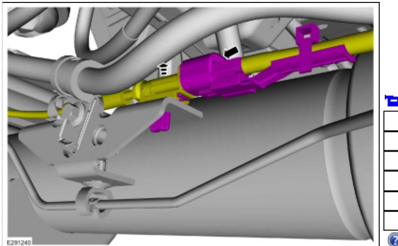
2. Detach the harness pin-type retainers.
