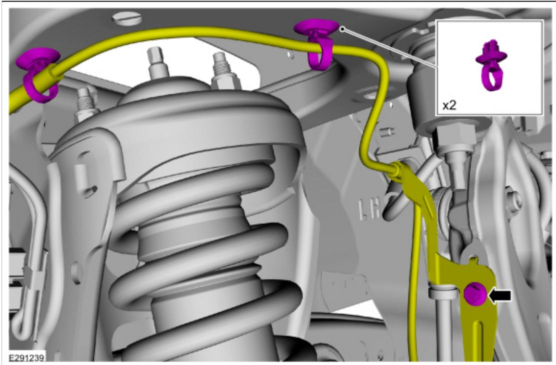
4. Using compressed air, clean the area surrounding the front wheel speed sensor.
