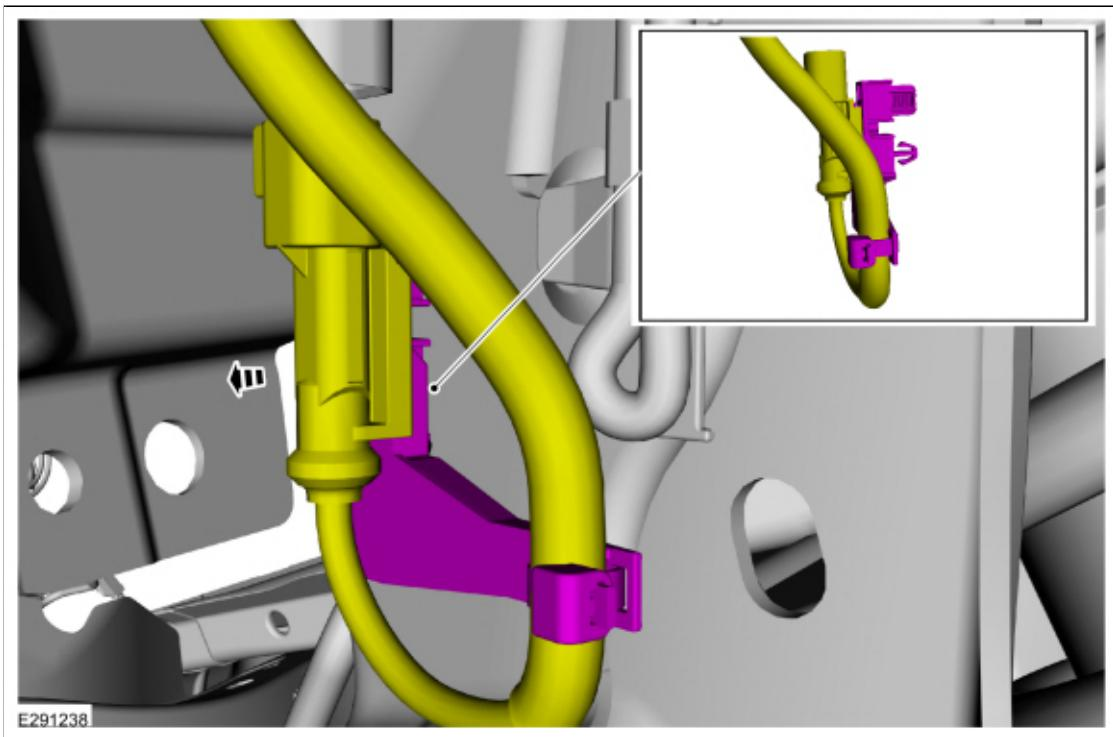
3. Detach the harness pin-type retainers and remove the harness routing bracket bolt.
