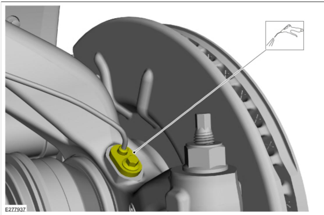
5. Remove the bolt and the front wheel speed sensor.
