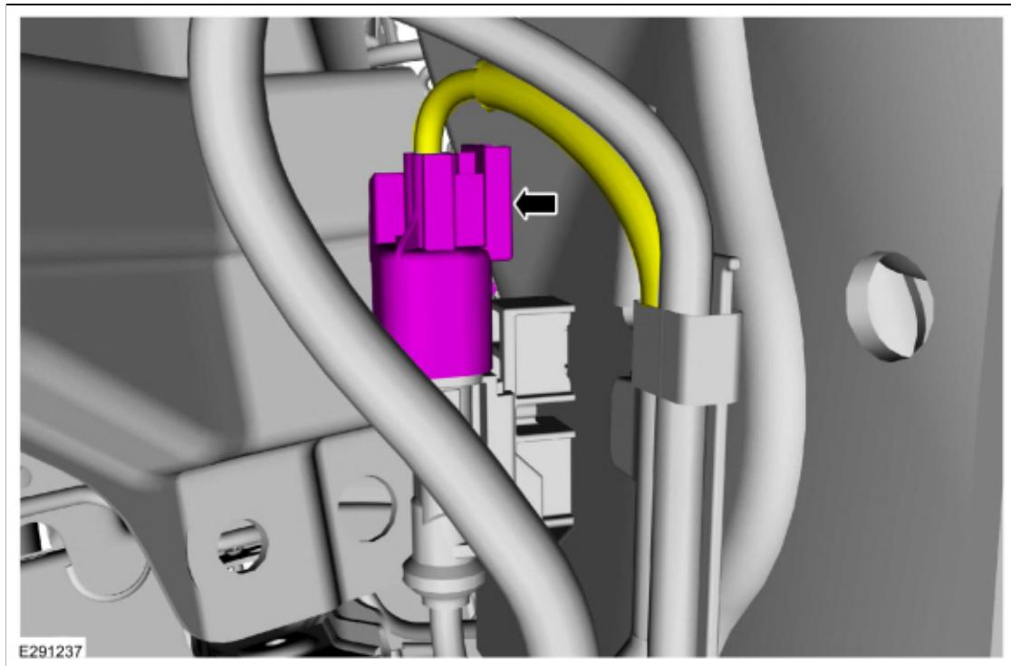
2. Detach the electrical connector bracket .
