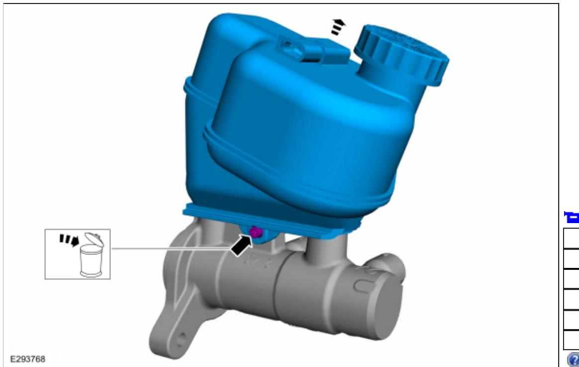
3. **NOTICE:** Only use the specified material to lubricate the seals.
