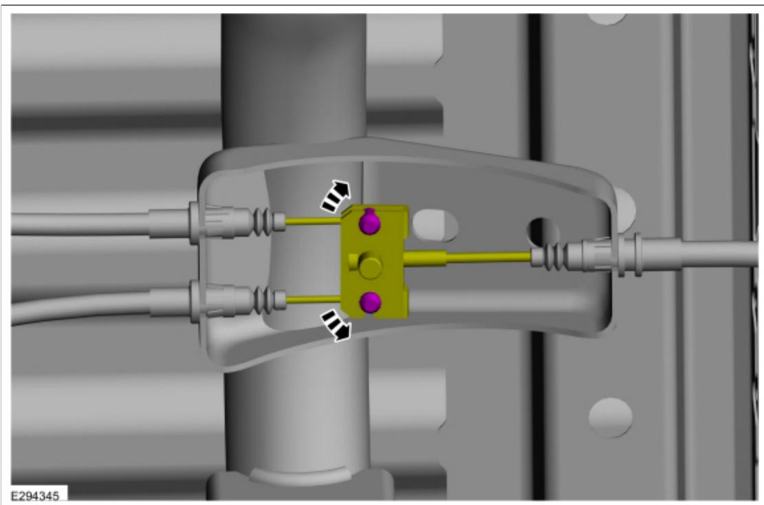
5. Remove the clip and detach the front cable from the bracket.
