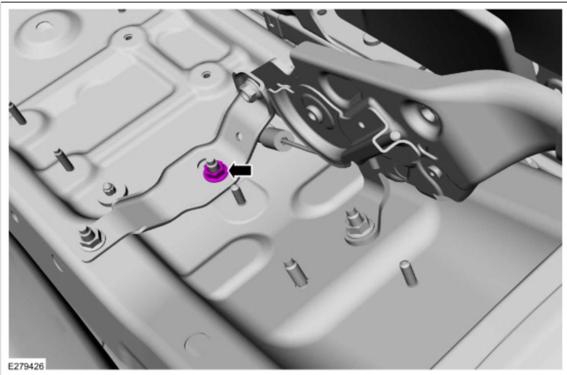
4. Detach the rear cables from the equalizer.
